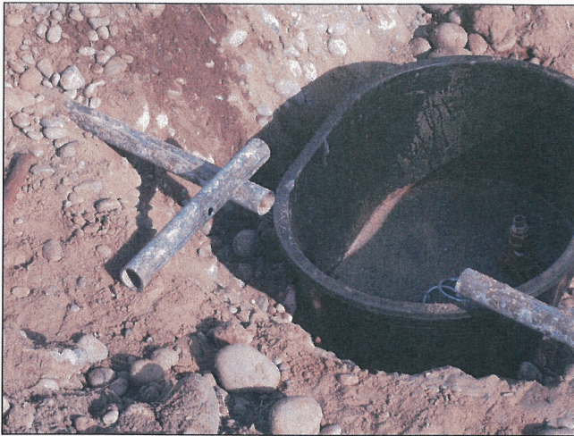
Rust-Scale Sample Material from Inside Pipe.
