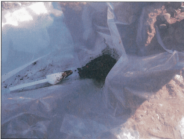
Rust-Scale Sample Material from Inside Pipe.
