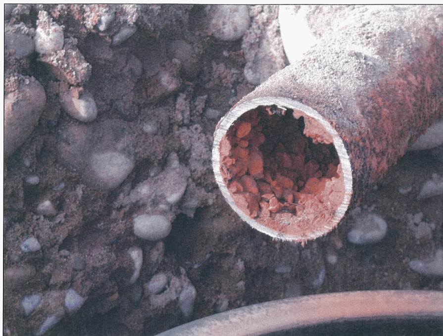
Figure 12. Rust and Scale Inside Pipe in Test Trench 2 at 100-F-52.
