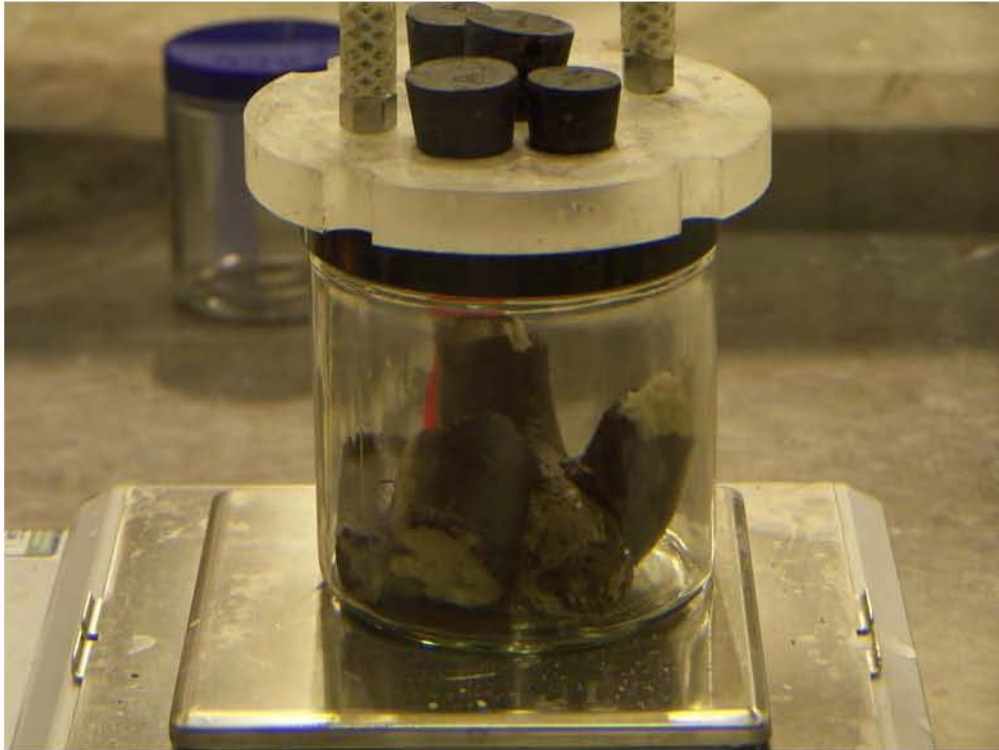
Figure 3. 241-AP-108 Core 330 Segment 24BR2 after Agitation.
