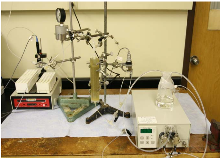
Figure 3.4: Photograph of the acid coreflood setup
