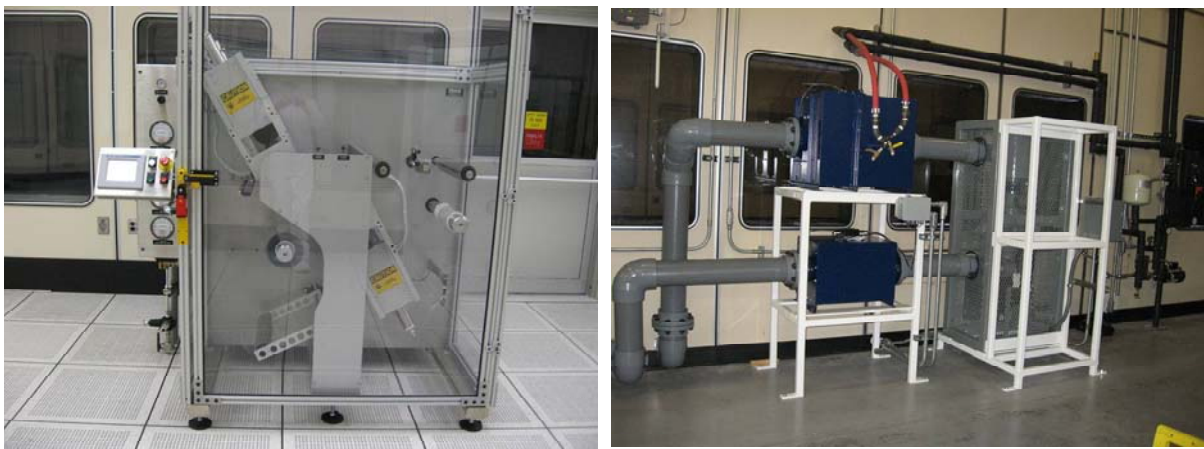
Figure 14 – web cleaning line installed at DCC utilizing dual ultrasonic air knives
