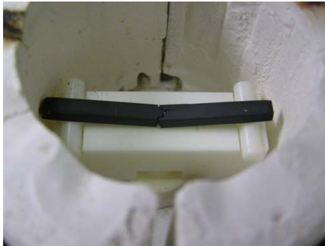
Figure 84: Fracture in OTM membranes under combined elevated temperature and pressure loading. The fracture origins are at the multiple indents placed on the tensile surface.
