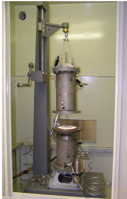
Figure 19 Laboratory set up for testing strength of ceramic membranes for tubes
