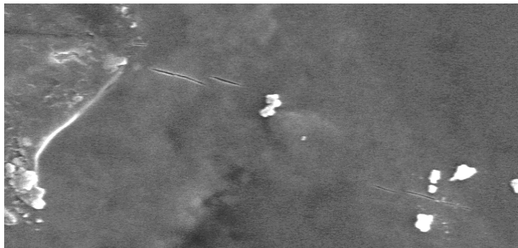
Figure 108. Crack bridging by dense region in the dual phase membrane.
