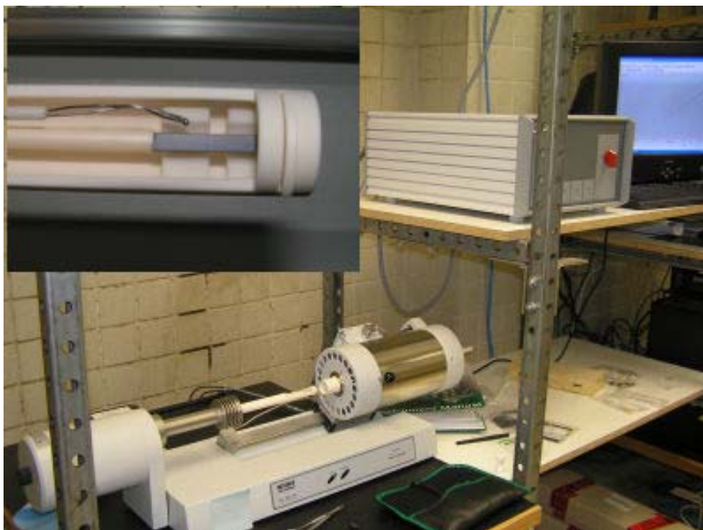
Figure 135. The dilatometer installed at the ceramic membrane lab and the sample holder with a LSFT-CGO membrane is shown in the inset.
