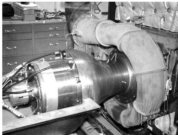
Figure 2. Electric Turbocharger Installed on a Test Stand at GRC
