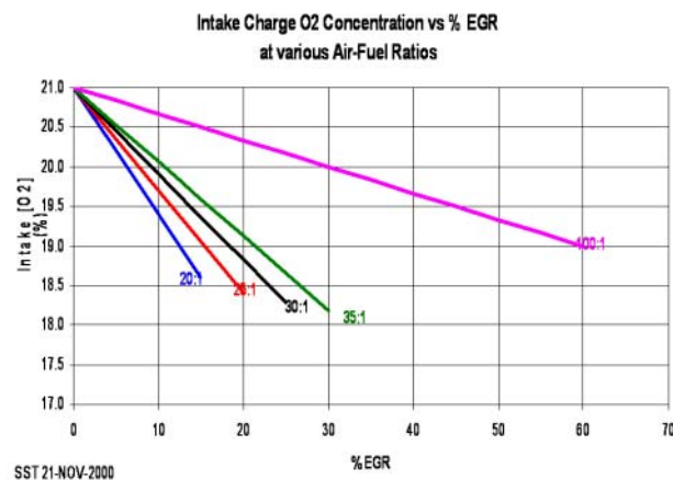
Figure 2. Amount of EGR Required to Lower Intake Air Oxygen Concentration at Different Air-Fuel Ratios
