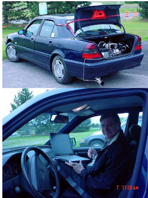
Figure 3. The Instrumented 1999 Mercedes C-Class Vehicle (top) Sensors Inc. Personnel Taking On-Vehicle PM Data (bottom)
