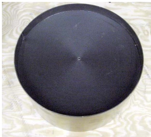
Figure 3. Example of 13" Diameter Prototype Substrate with Alloys B and C and a Straight-Channel Design
