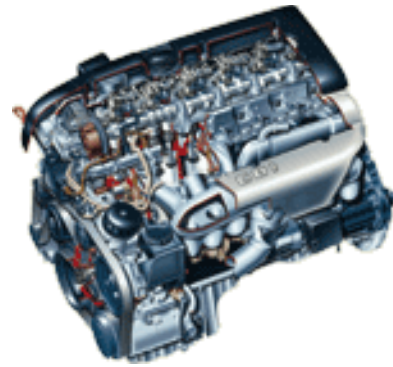
Cut-Away of DaimlerChrysler 3.2 L CIDI Engine that Achieves 30% Better Fuel Economy than its Gasoline Counterpart in Mercedes Light-Duty Vehicles
