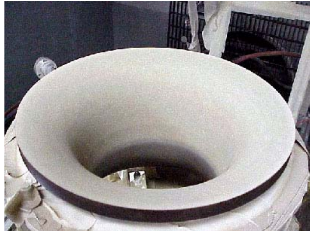
Figure 3. Turbocharger Air Inlet after Application of Polymeric Abradable Coating
