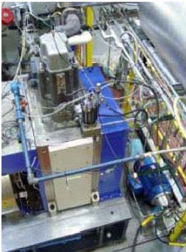
Figure 1. Common Rail Fuel System Components Installed on the Single-Cylinder Locomotive Engine at GE GRC
