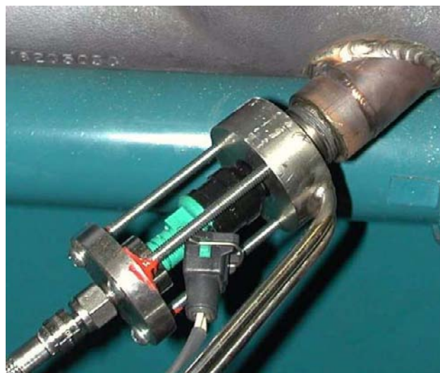
Figure 2. In-Pipe Fuel Injection for NO x Adsorber Regeneration
