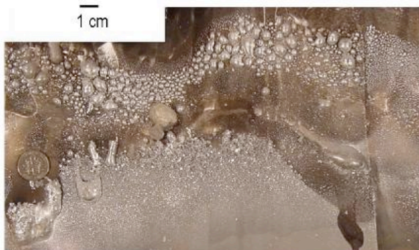
Figure 127 - Magnesium deposit from scale-up experiment
