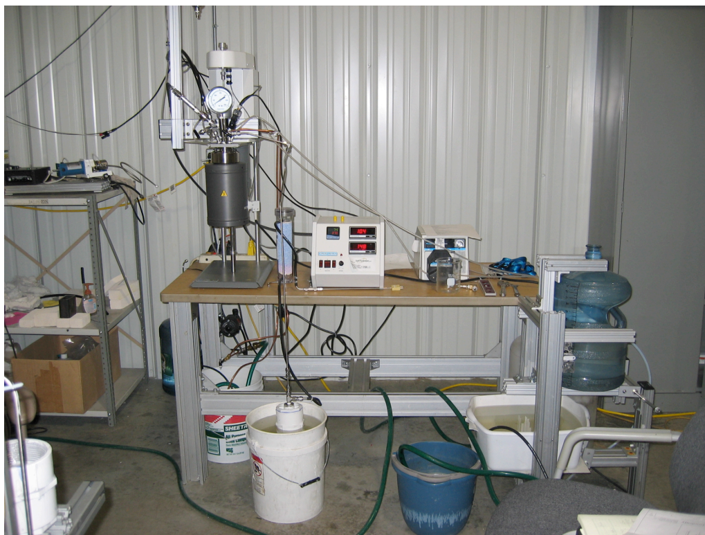
Figure 10 - Parr Autoclave Reaction Rate Testing Apparatus
