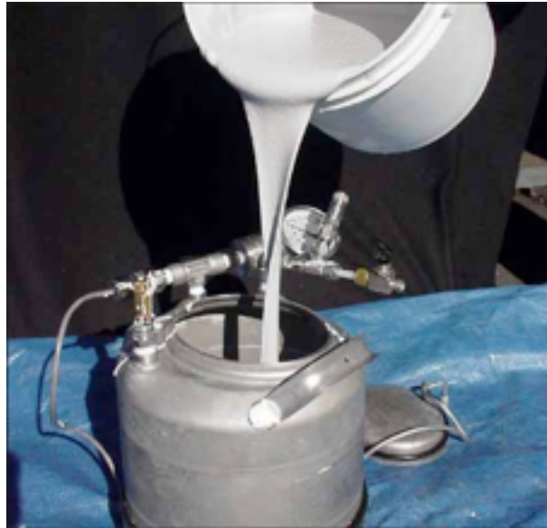
Figure 1 - Lithium Hydride slurry prepared during previous chemical hydride slurry development program
