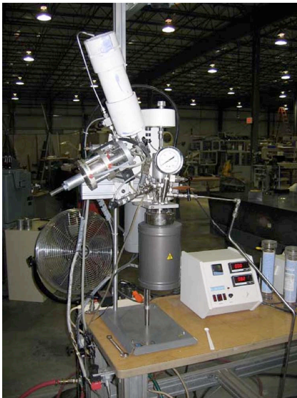
Figure 34 - Slurry Piston Pump with Parr Autoclave Apparatus
