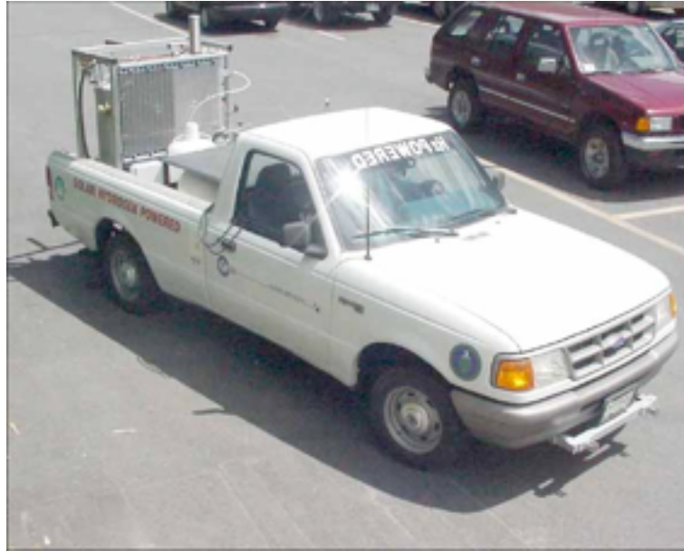
Figure 2 - Lithium Hydride slurry laboratory mixing system mounted in the bed of a Ford Ranger pickup truck to demonstrate its ability to provide hydrogen for a modified IC engine
