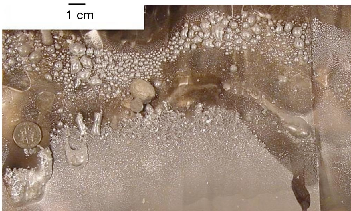
Figure 119 - Magnesium deposit from scale-up experiment
