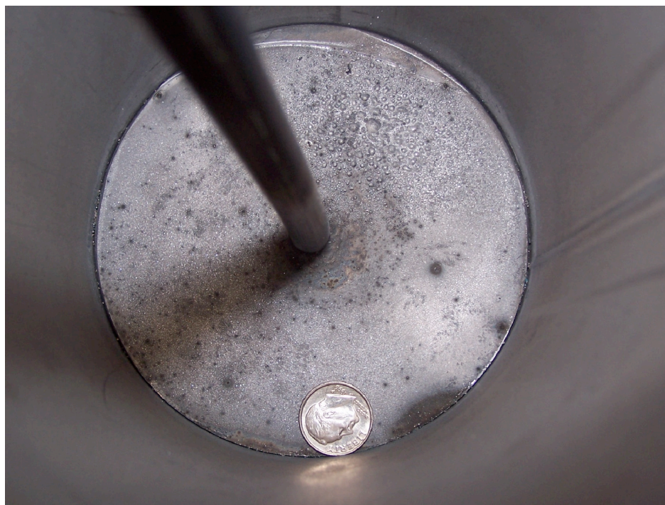
Figure 187 - Magnesium Deposit on Floor of Condenser
