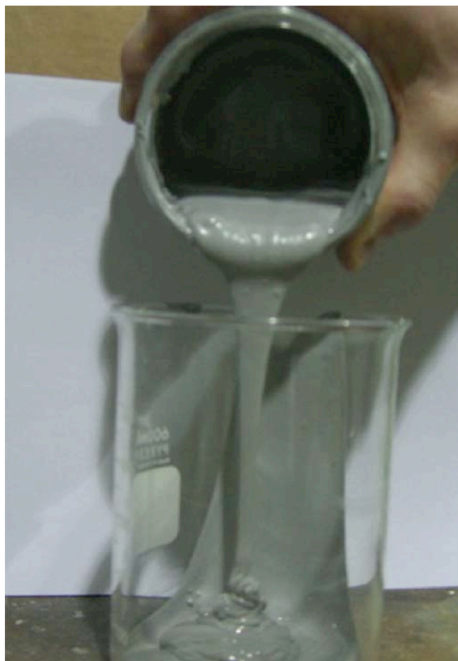
Figure 4 - 70% Magnesium Hydride Slurry Pouring
