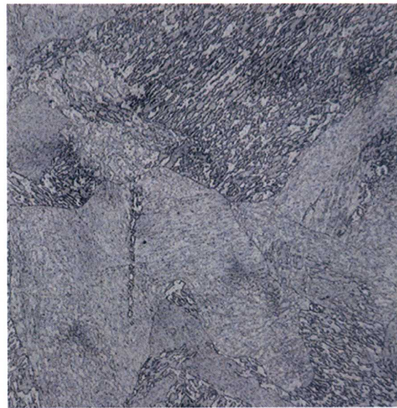
#2 3Cr-2WVTa 1100°C/700°C 200X 20μm 50H 2 O/5HNO 3 /1HF
