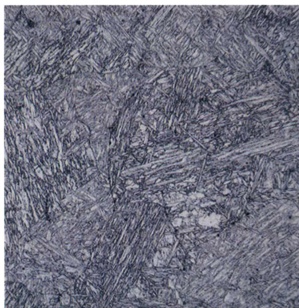
#45 COST CB2 1100°C/700°C 200X 20μm 50H 2 O/5HNO 3 /1HF
