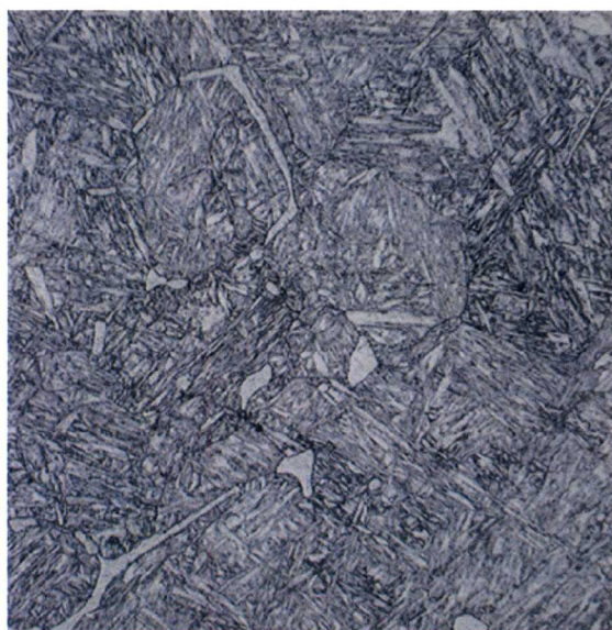
#29 9Cr-2WVTa 1100°C/700°C 200X 20µm 50H 2 O/5HNO 3 /1HF
