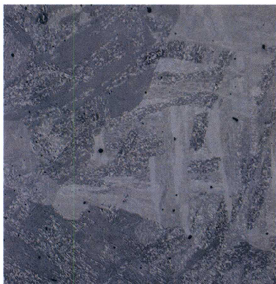
3Cr-3WV #1 1050°C Long. View 50X 100μm 50H 2 O/5HNO 3 /1HF
