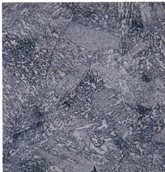
#3 3Cr-2WMoVTa 1100°C/700°C 200X 20μm 50H 2 O/5HNO 3 /1HF
