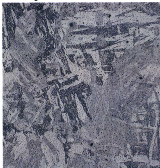
3Cr-3WVTa B #21 1100°C Long. View 50X 100μm 50H 2 O/5HNO 3 /1HF
