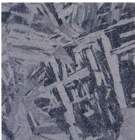
3Cr-3WV #1 1100°C Long. View 50X 100μm 50H 2 O/5HNO 3 /1HF
