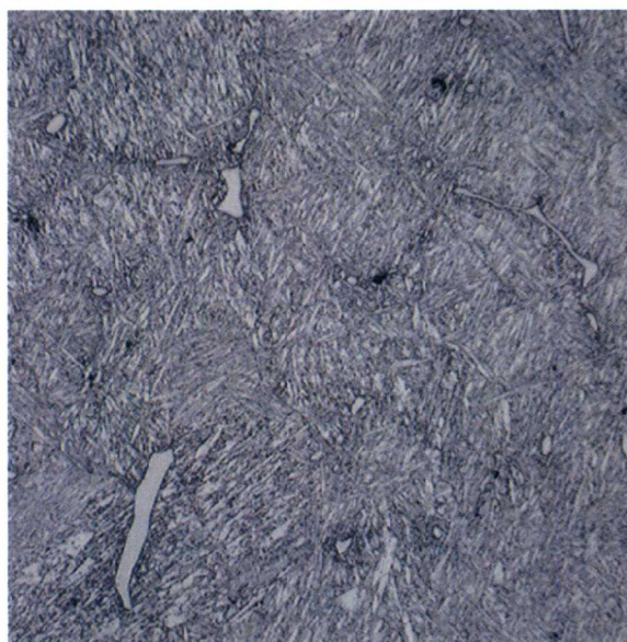
#31 11Cr-2WVTa 200X 20μm 1100°C/750°C 50H 2 O/5HNO 3 /1HF
