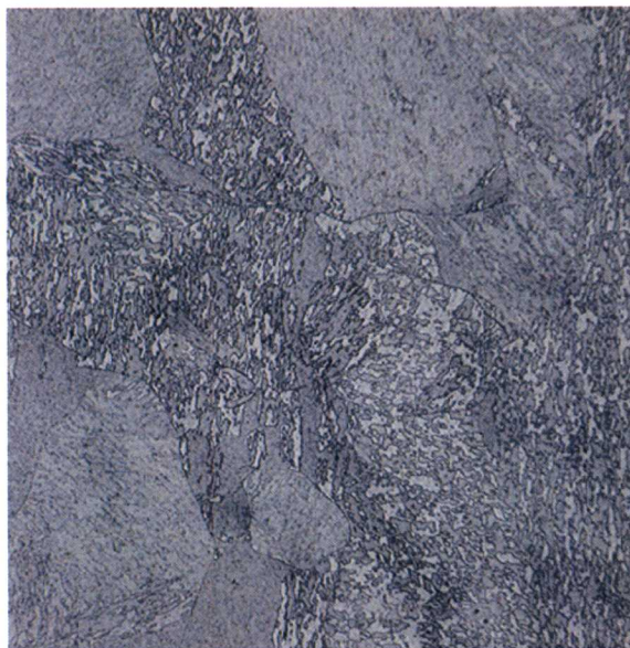
#1 3Cr-3WV 1100°C/700°C 200X 20μm 50H 2 O/5HNO 3 /1HF
