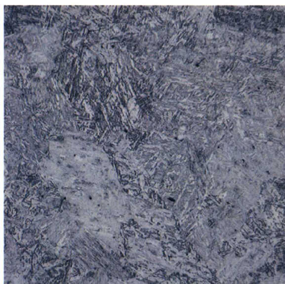
9Cr-2WVTa #29 1100°C Long. View 50X 100μm 50H 2 O/5HNO 3 /1HF
