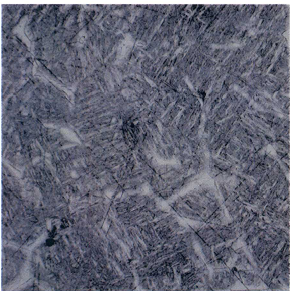
Figure 75. Optical microstructure of 11Cr-2WCoMnNbV steel (Cast E) austenitized 1 h at 1100°C (left) and 7 h at 1100°C (right).
