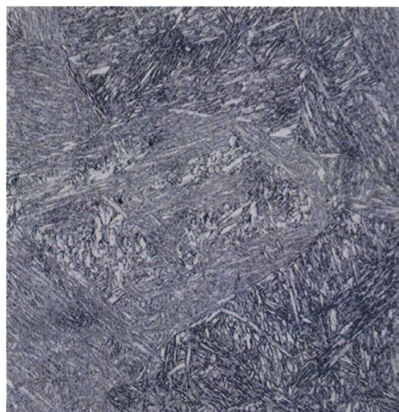
#18 11Cr-1WMoV 200X 20μm 1100°C/750°C 50H 2 O/5HNO 3 /1HF
