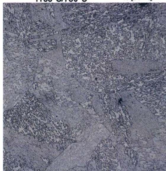
#21 3Cr-3WVTaB 1100°C/750°C 200X 20μm 50H 2 O/5HNO 3 /1HF
