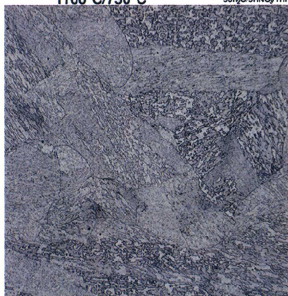
#3 3Cr-2WMoVTa 1100°C/750°C 200X 20μm 50H 2 O/5HNO 3 /1HF
