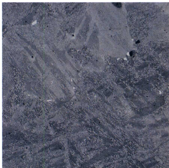
3Cr-2WMoVTa #3 1050°C Long. View 50X 100μm 50H 2 O/5HNO 3 /1HF
