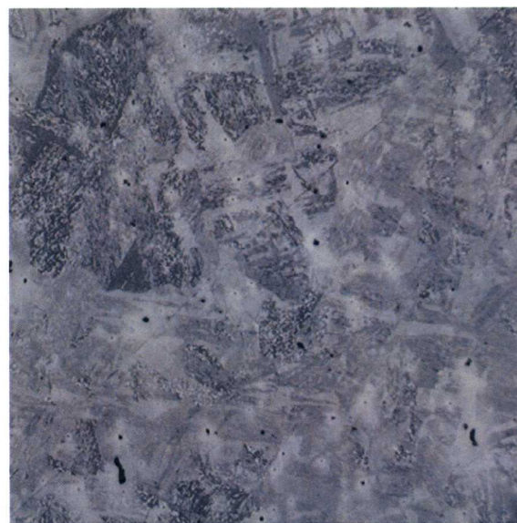
3Cr-3WVTa B #21 1175°C Long. View 50X 100μm 50H 2 O/5HNO 3 /1HF
