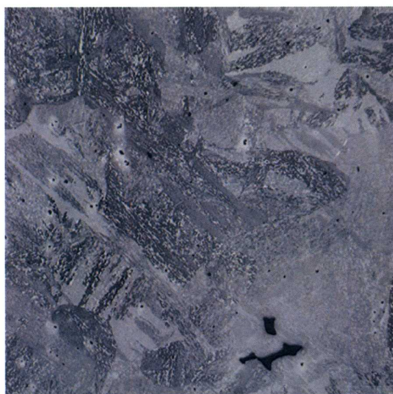
3Cr-2WMoVTa #3 1175°C Long. View 50X 100μm 50H 2 O/5HNO 3 /1HF
