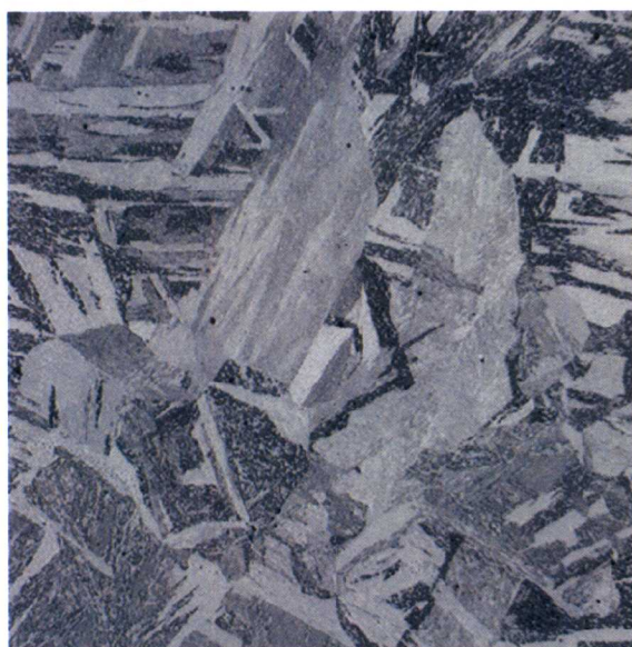
3Cr-2WMoVTa #3 1100°C Long. View 50X 100μm 50H 2 O/5HNO 3 /1HF
