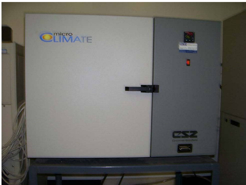
Fig 3. Climatic chamber & thermostat with temperature range from -80^{\circ}\text{C} to +120^{\circ}\text{C}
