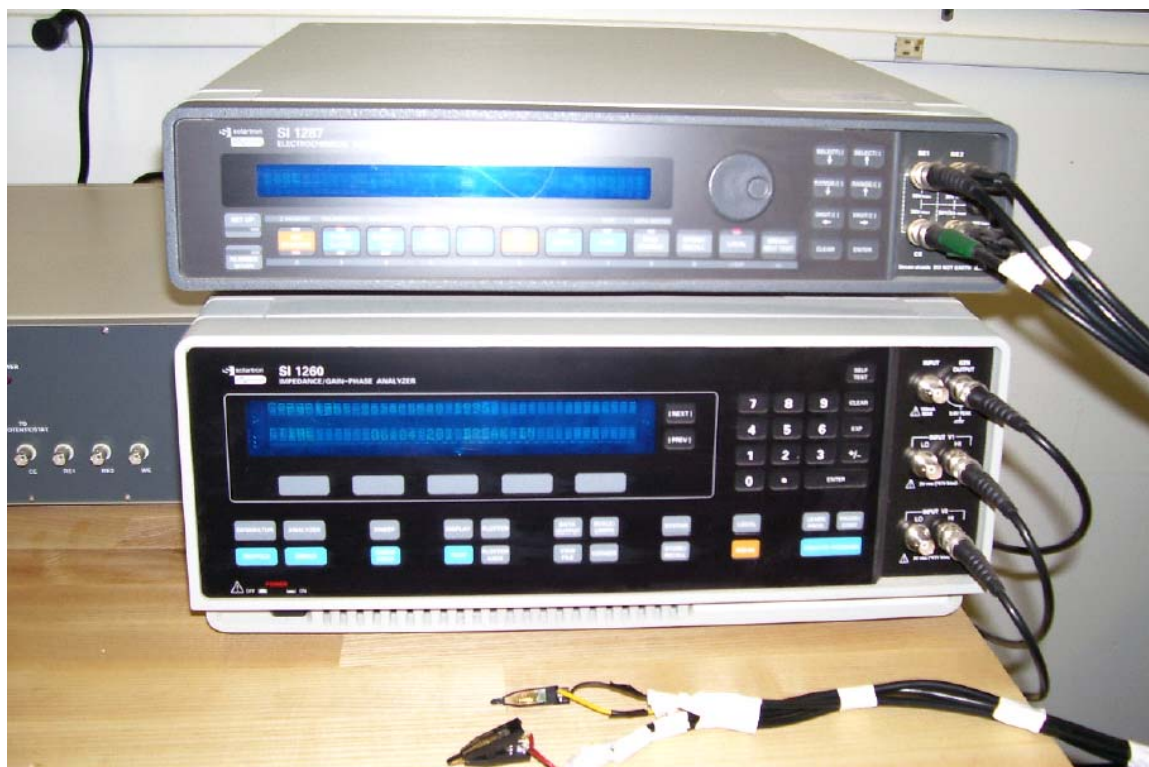
Fig. 5 EIS measurements are performed with Solartron frequency response analyzer with electrochemical interface
