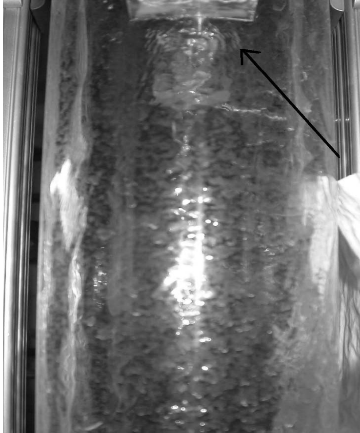
Figure 3.17 Appearance of wakes in the flow during a liquid only run of the facility
