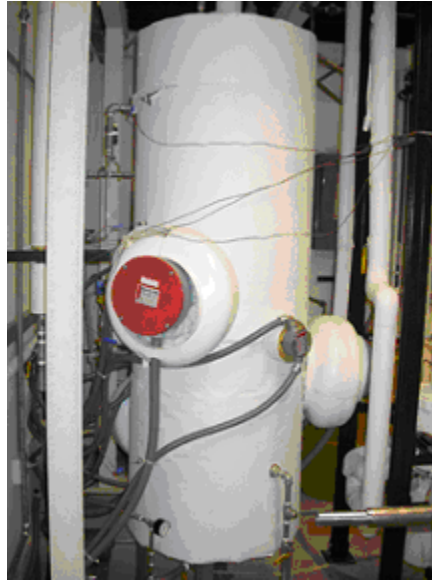
Figure 3.28 Steam generator after insulating.
