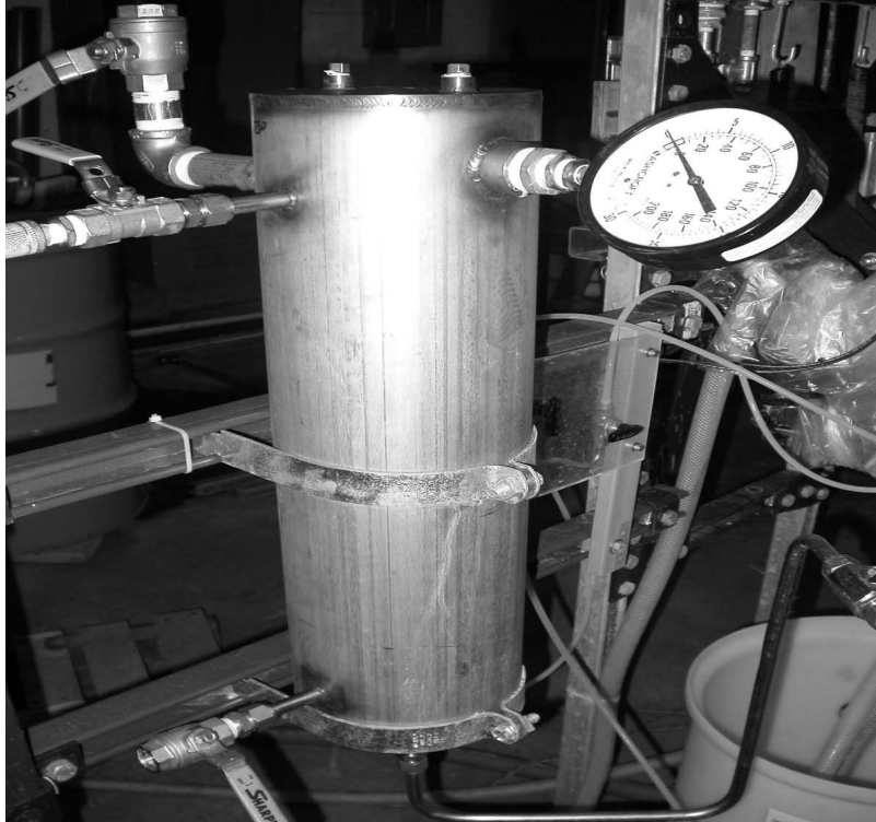
Figure 3.10 Pressure vessel for water delivery to the upper pressure transducers and aiding in the purging process
