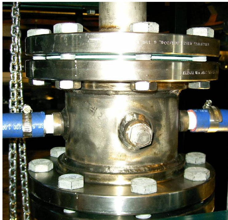
Figure 3.26 Water injection device prior to insulation
