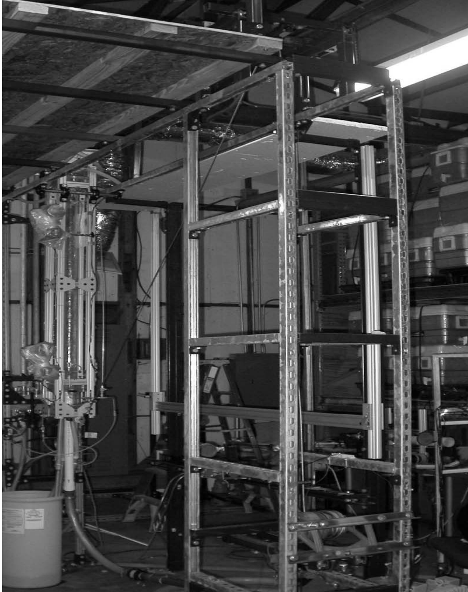
Figure 3.5 The frame used to support the test section and the necessary experimental equipment
