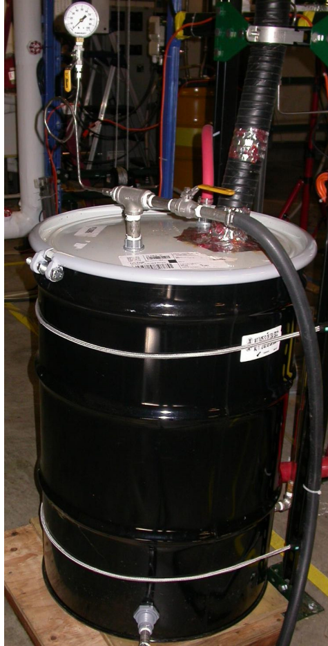
Figure 3.29 Steam-water outlet tube connected to the blow down tank
