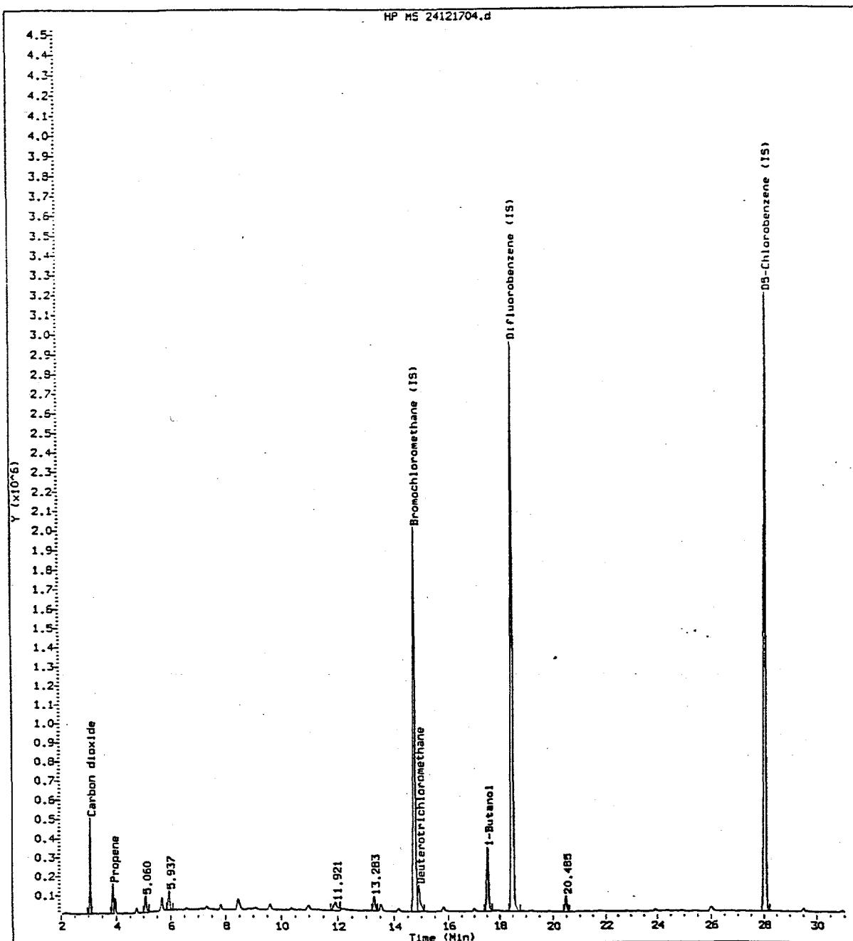
**Figure 3.1a** Total Ion Chromatogram (0 - 30 minutes) of Hanford Tank C-105 SUMMA™ Canister S4005 04.B16 Collected on 2/16/94
