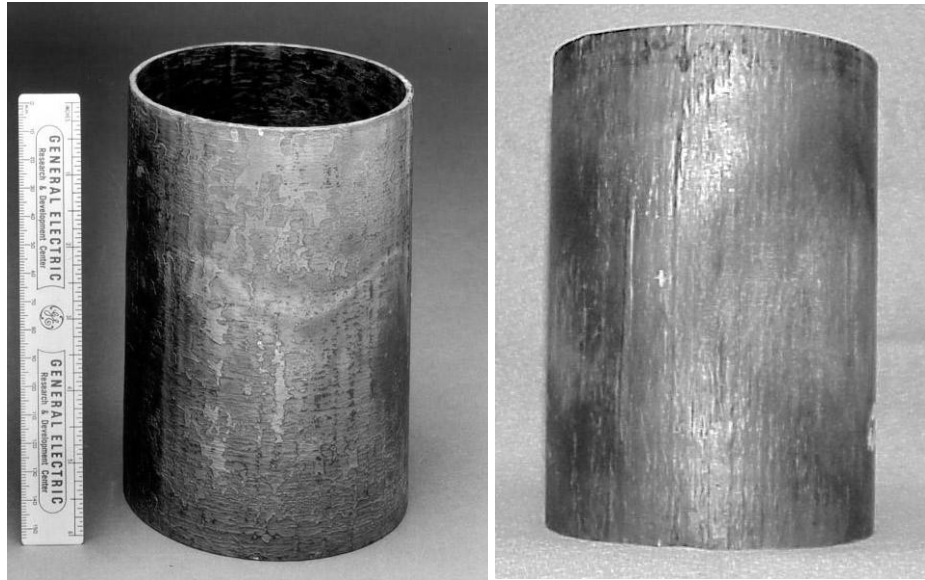
Figure 3-148. Photographs of the Prepreg MI CMC liners made for the shroud combustion test rig.
