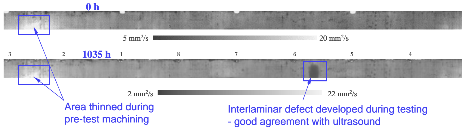
Figure 3-247. IR transmission thermography images of the PGT-2 CMC stage 2 shroud both before and after engine testing.
