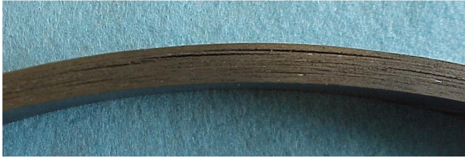
Figure 3-267. Photograph of the thick edge of stage 1 shroud ring #1 showing the presence of the ply delaminations.
