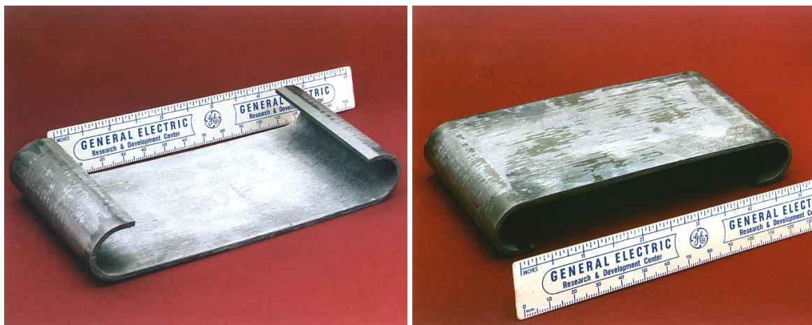
Figure 3-143. Photographs of a typical GE Prepreg MI shroud in the as-fabricated state.
