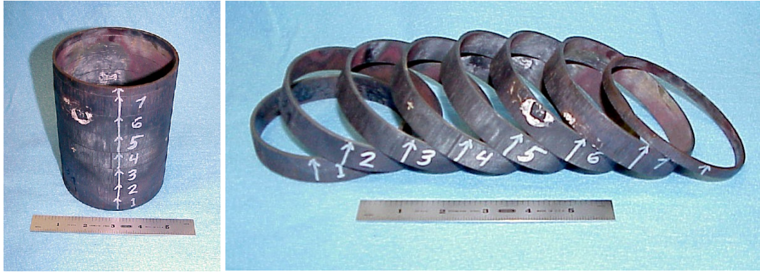
Figure 3-183. Photographs of the 2nd shroud rig combustor liner following sectioning for burst tests. Left – with the rings stacked in their original positions; Right – with the rings splayed apart to show the individual pieces. The arrows mark the direction of gas flow during rig operation.
