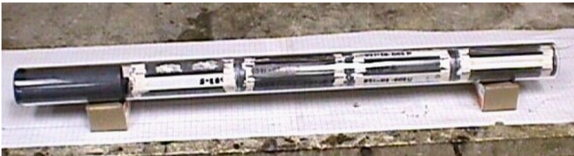
Figure 3-282. Top - Photograph of a single sample “cartridge” assembly consisting of seven test bars and two retaining rings; Middle – Photograph of four cartridges showing the alumina-silica cement used to hold the sample ends securely to the retaining rings; Bottom – one spacer tube and four sample cartridges (left to right) inside a glass tube to show the arrangement of samples as they would be inside the long-term combustion rig main sample tube.
