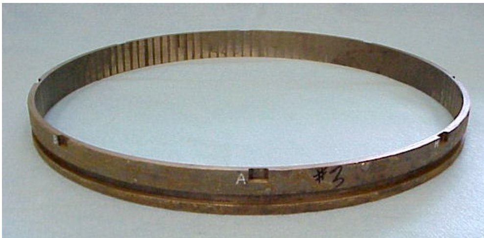
Figure 3-268. Photograph of the PGT-2 CMC 1 st stage shroud ring #3 following machining.
