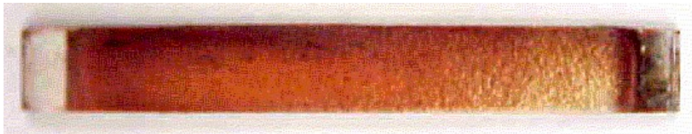
Figure 3-291. Photograph of a prepreg MI CMC sample with an environmental barrier coating (EBC) that was exposed in the first rank of the long-term rig during run #1. The gas flow direction is left to right.
