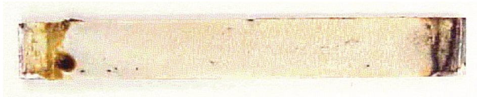
Figure 3-290. Photograph of a prepreg MI CMC sample with an environmental barrier coating (EBC) that was exposed in the fourth rank of the long-term rig during run #1. The gas flow direction is left to right.
