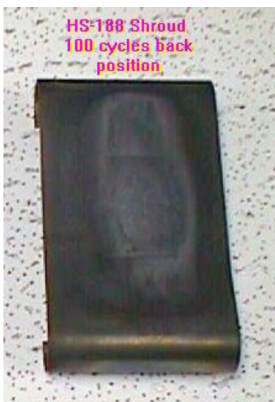
Figure 3-155. Photograph of the second HS-188 shroud following rig testing in a rear position during run 31. The shroud hot gas path face was highly warped and heavily oxidized after ~2 hours exposure and 100 thermal cycles.
