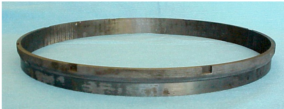
Figure 3-266. Photograph of the PGT-2 stage 1 shroud ring #1, made to design “C” with a stepped cross section thickness, following machining. The ID of the shroud ring 422mm.
