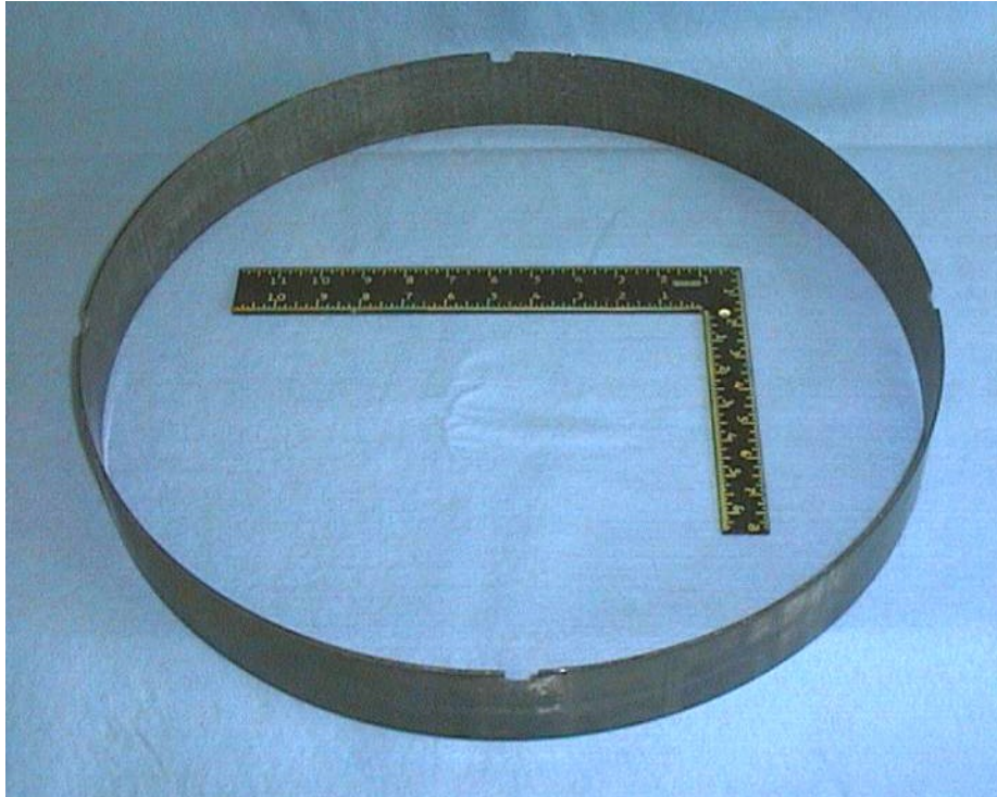
Figure 3-235. Photograph of the 2nd PGT-2 stage 2 shroud ring following machining.
