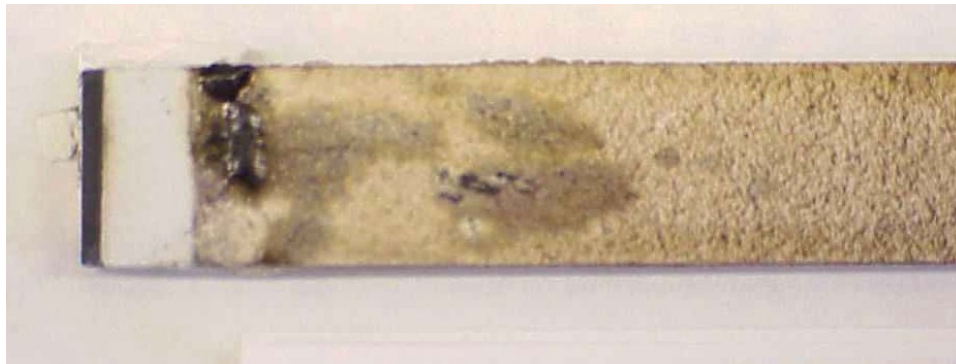
Figure 3-284. Close-up photograph an EBC-coated sample from the 2h rig run at 1200°C, showing deposition of a glassy contaminant on the sample surface.
