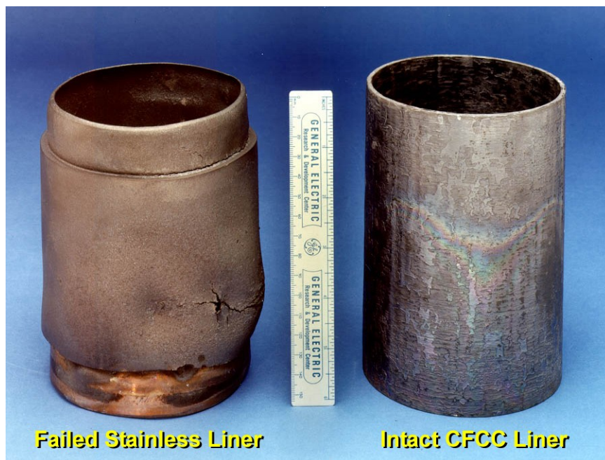
Figure 3-177. Photograph of the failed stainless steel combustor liner and the 1 st GE Prepreg CMC liner used in the shroud combustion rig tests.
