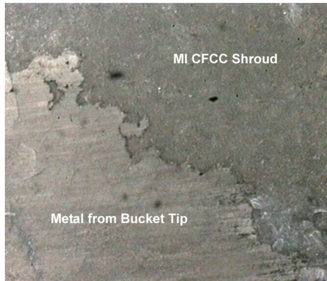
Figure 3-244. Close-up photograph of the edge of the blade rub region showing the metal from the blade smeared over the CMC shroud. Little to no abrasion of the CMC was noted.
