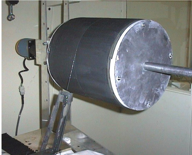
Figure 3-219. Photograph of drum winding process for applying hoop-oriented plies to a Prepreg MI Frame 5 combustor preform. This particular liner was built on a carbon mandrel with BN spray coating (white) on the surface.
