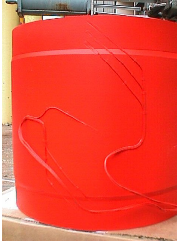
Figure 3-223. Photograph of one of the instrumented metallic liner segments following application of the temperature-indicating paint.
