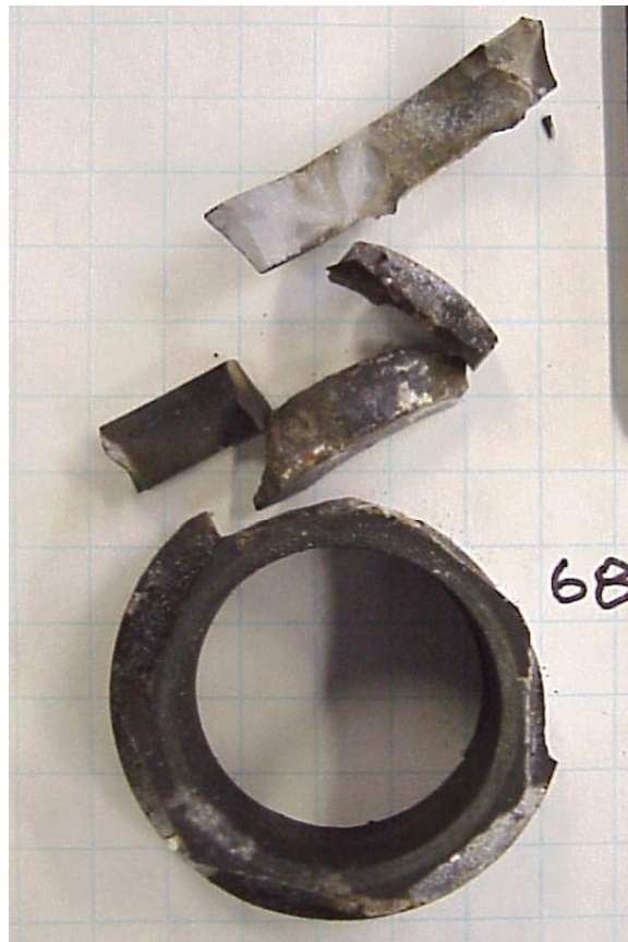
Figure 3-285. Photograph of one of the sample retaining rings following the first 500 hour test in the long-term combustion rig. The inner portion of the ring, which was fiber reinforced, maintained integrity whereas the outer monolithic SiC-Si portion broke in several locations.
