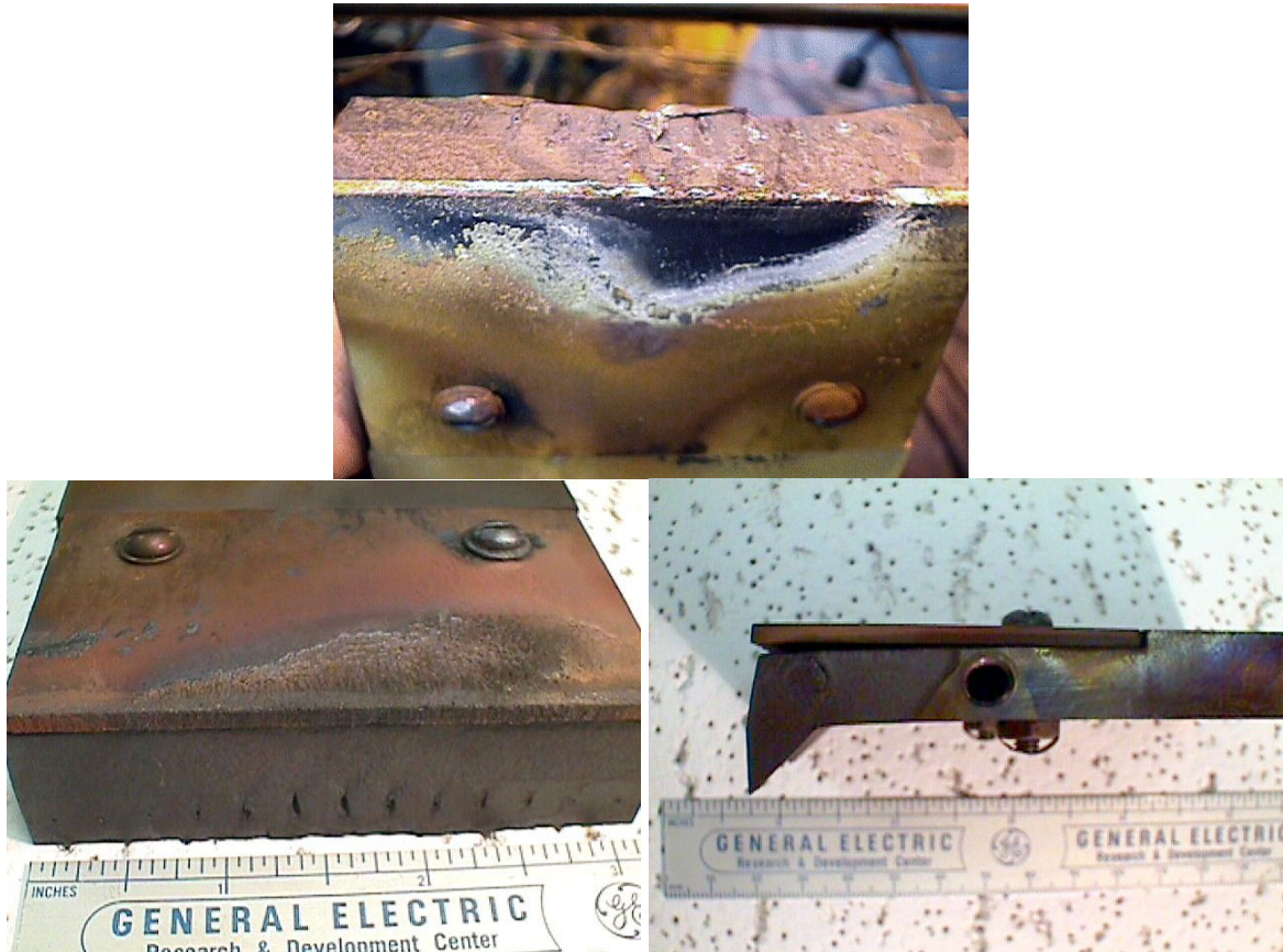
Figure 3-158. Photographs of two of the modified nozzle simulation flanges incorporating the bolted-on CMC plate on the leading edge. The reddish appearance of the CMC plates is from iron oxides that deposited during rig testing.
