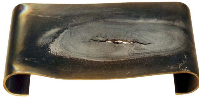
Figure 3-154. Photograph of the HS-188 shroud following rig test exposure in rig run 28. Shroud warping, oxidation and thermal fatigue cracking are evident.
