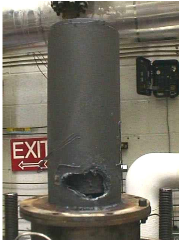
Figure 3-279. Photograph of the inner pressure vessel shell showing the hole that was burned out due to the failed fuel nozzle dome plate.
