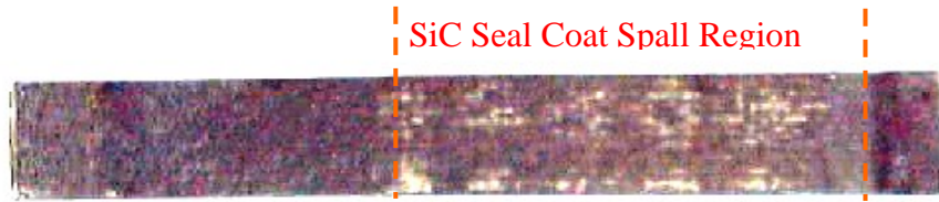
Figure 3-289. Photograph of a slurry cast MI CMC sample on which approximately 50% of the CVD SiC seal coat has spalled during long-term rig run #1. The gas flow direction is left to right.
