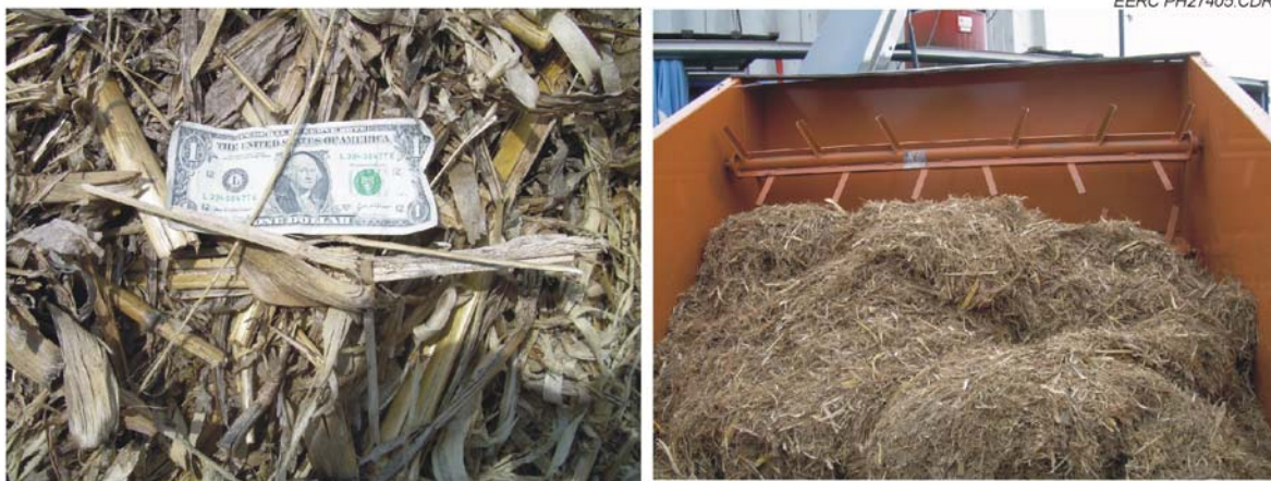
Figure 18. Corn stover before reduction in size (left) and after size reduction (right).
