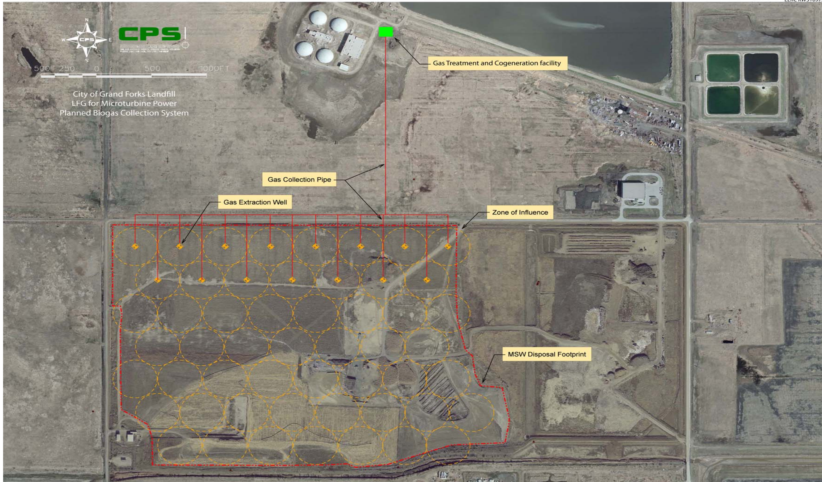
Figure 64. Planned biogas collection system. This schematic shows the relative distance between the landfill site, the baling facility (northeast corner of landfill, across from the composting site), and the wastewater treatment plant (upper center). The image shows 53 gas extraction wells, the 250-foot zone of influence for each well, the collection system, and the biogas treatment and power generation package. The possible scenario given here places the cogeneration package at the WWTP and assumes only electricity would be sent to the baling facility over a city-owned transmission system, while both electricity and heat would be utilized at the WWTP.
