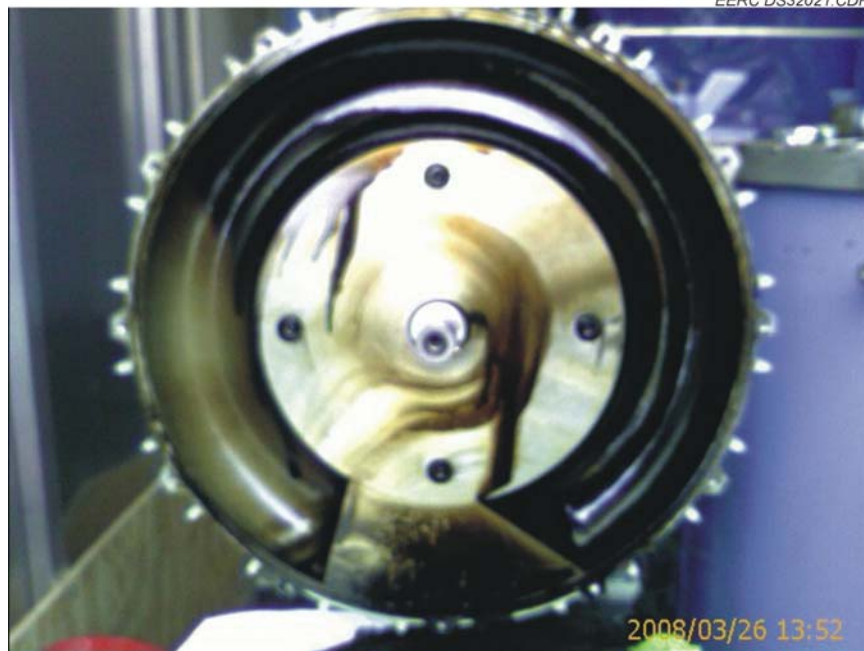
Figure 34. Tar condensation in the process blower.
