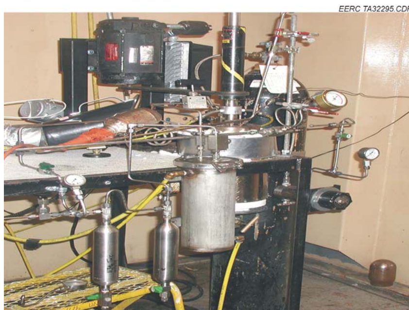
Figure 53. Photo of thermal cracking apparatus.
