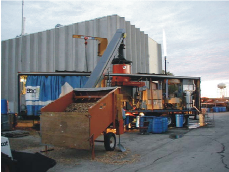
Figure 7. Portable gasifier test setup.
