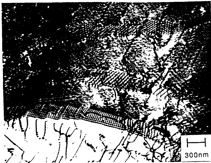
Fig. 4.47 Dislocation array in DO 3 ordered FA-129 fatigued in air at 450°C.
