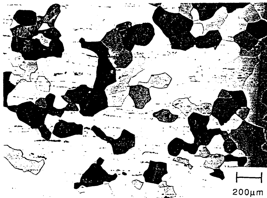
Fig. 4.2 Grain structure of B2 ordered FA-129 utilizing a 900°C + 700°C anneal. Rolling direction ↔
