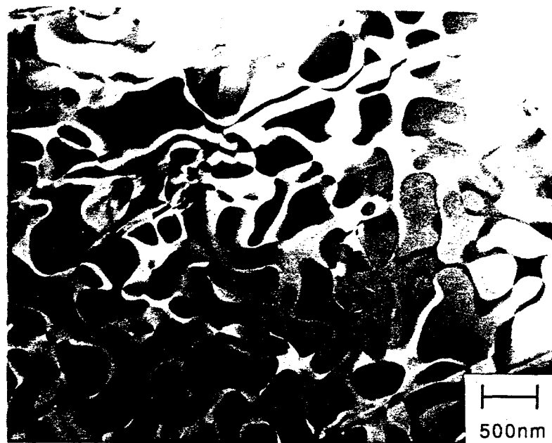
Fig. 4.46 APB's in DO 3 ordered FA-129 fatigued in hydrogen at 25°C.
