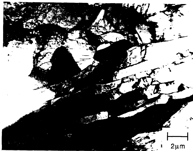
Fig. 4.45 Dislocation structure in B2 ordered FA-129 fatigued in air at 25°C.
