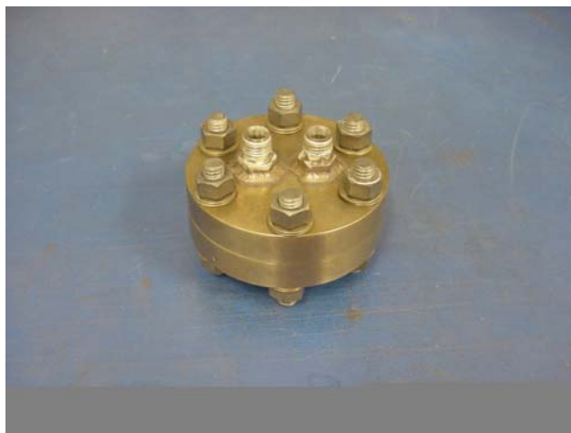
Figure 59. IdaTech permeation cell used in initial pressure testing of thin membranes
