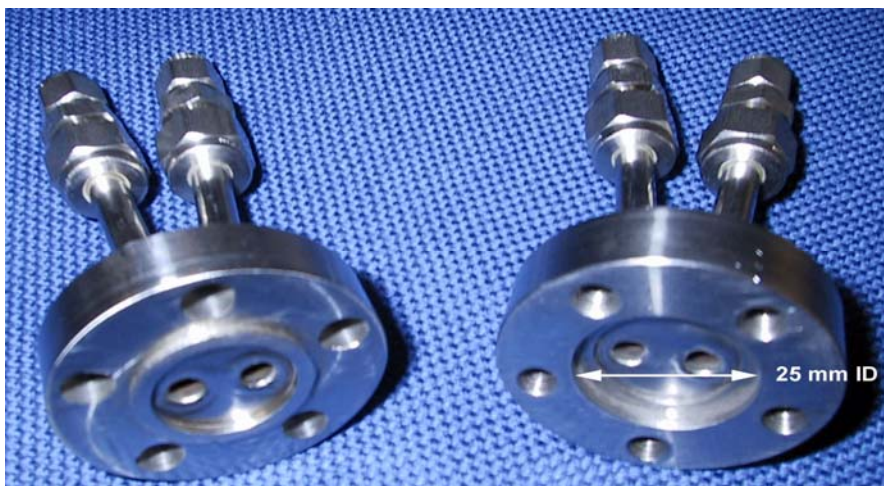
Figure 3. New stainless steel flow cell for 25 mm diameter membrane samples
