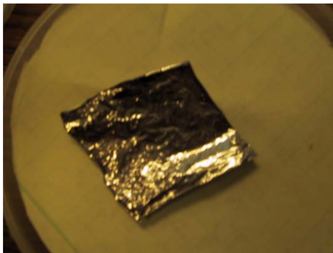
Figure 55. Sample 073106#1 after 24 hours at 400°C in forming gas
