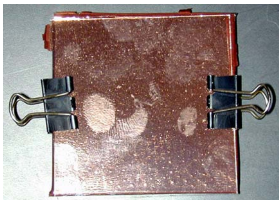
Figure 5. Copper film (3 \mu\text{m} ) on PVA; sample is sandwiched between two pieces of glass
