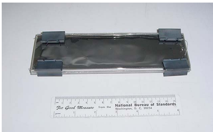
Figure 23. Photograph of fixture used to hold membranes flat during annealing
