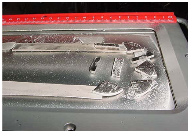
Figure 22. Sputter target modified to increase the membrane Pd content
