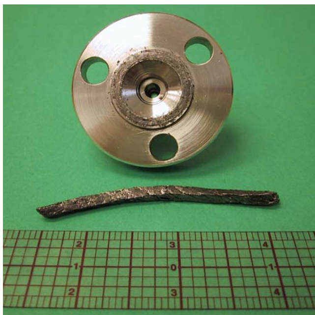
Figure 2. 25 mm Millipore membrane cell with high temperature Grafoil valve packing material used in place of a polymer o-ring. Maximum use temperature of Grafoil material is 650°C.
