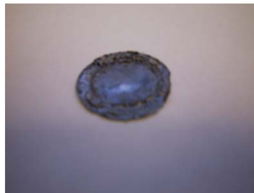
Figure 35. Image of Pd60Cu40 standard foil showing the apparent carbon contamination on the surface that appeared after testing.
