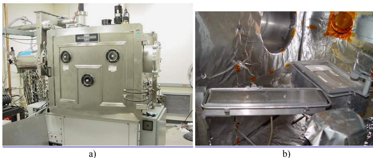
Figure 1. a) Mill Lane Vacuum Coating Platform, b) plasma cleaning & magnetron set-up
