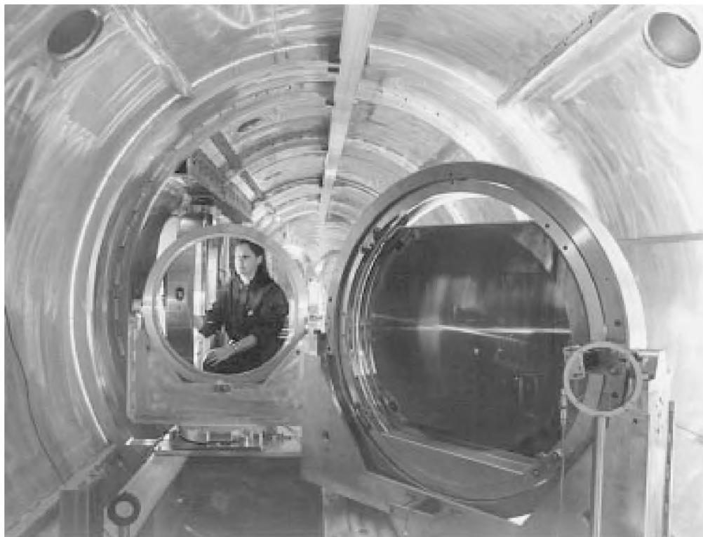
FIGURE 15. Inside the Petawatt vacuum compressor chamber. The two pulse-compression gratings produce a subpicosecond output pulse from a spectrally chirped input pulse more than a thousand times longer in duration.
