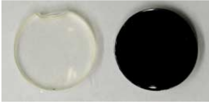
Figure 51. Material A at 0 (left) and 24 (right) hours of exposure to 225 °C in air.
