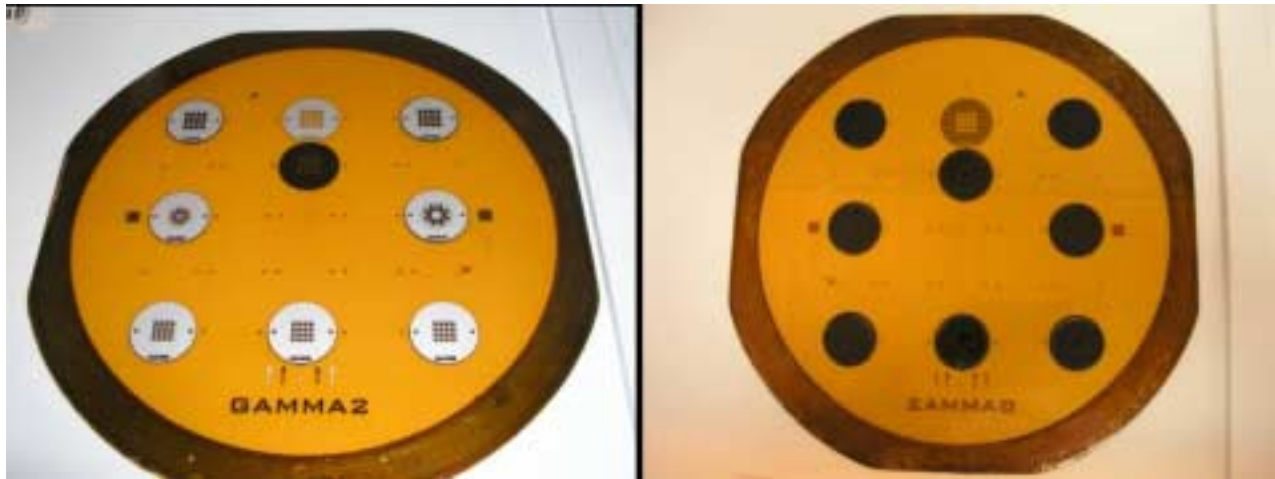
Figure 39. Gen 2 APD sub-mount build, showing several arrays on a Kapton frame. At left, the front side is shown, while the back-side is shown at right.
