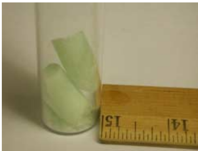
Figure 65. Photo of the initial trial growth of \text{Cs}_2\text{NaPrCl}_6 . The adjacent rule has units of inches.
