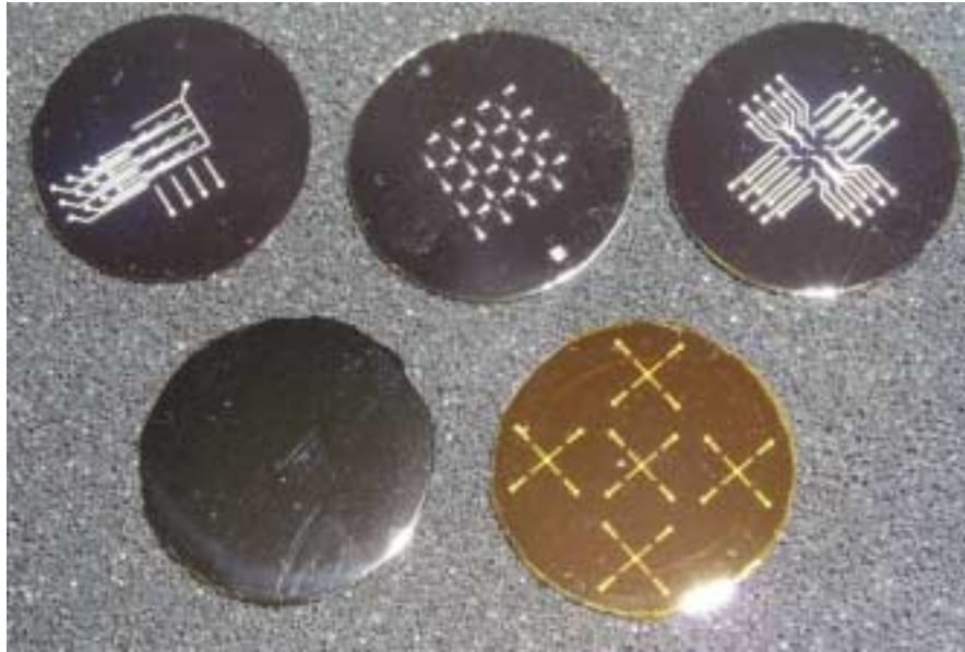
Figure 38. APD array sub-mounts from the first iteration ('gen 1'). Various metals as well as various layout geometries were prototyped to make the process as robust as possible.
