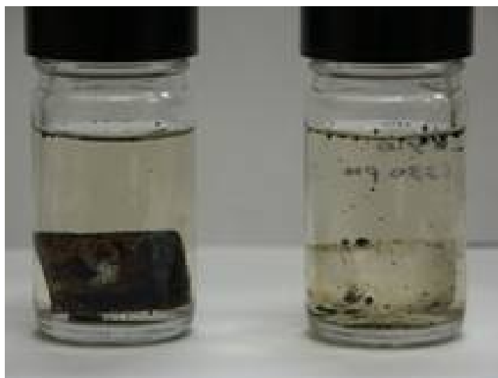
Figure 2. (Left) -- calcite crystal initially coated with a heavy oil and immersed in a surfactant solution (Right) - calcite crystal after several weeks exposure to an efficient surfactant. Almost all of the surface of the crystal is visible.
