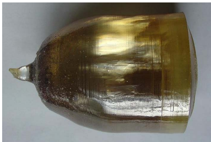
Fig. 3.2. \text{Cd}_{0.9995}\text{Gd}_{0.0005}\text{WO}_4 single crystal boule with 60 mm diameter
