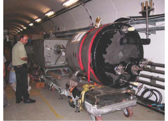
Fig. 20. Photograph of the MERIT apparatus installed in the TT2A tunnel at CERN. The 15 T solenoid is in the foreground with the Hg containment located downstream.
