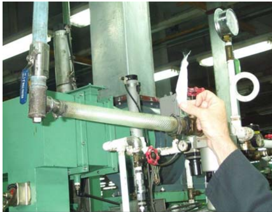
a. leaks at rubber hose connection
