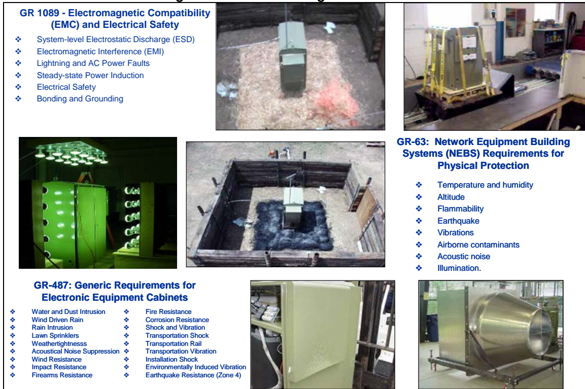
Figure15 : NEBS Testing of the GenCore
