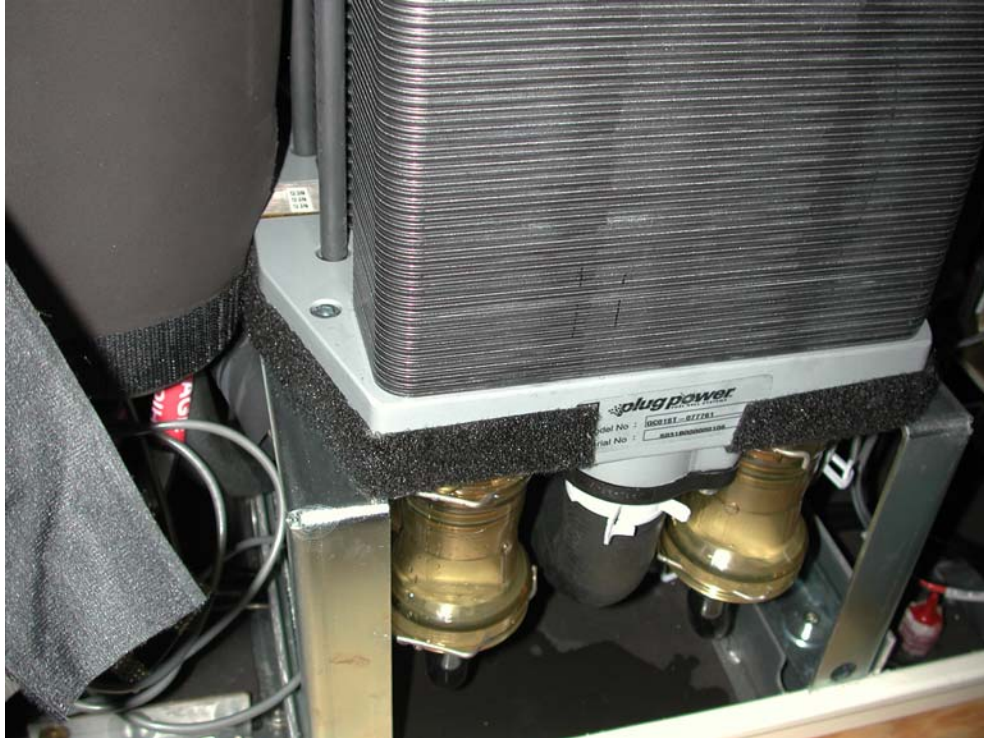
Fig. 21. Photograph of the inside, left-hand (as you look at it) corner of the GenCore unit. There is a colorless liquid present on the bottom of the unit; most likely this is ethylene glycol-based coolant.
