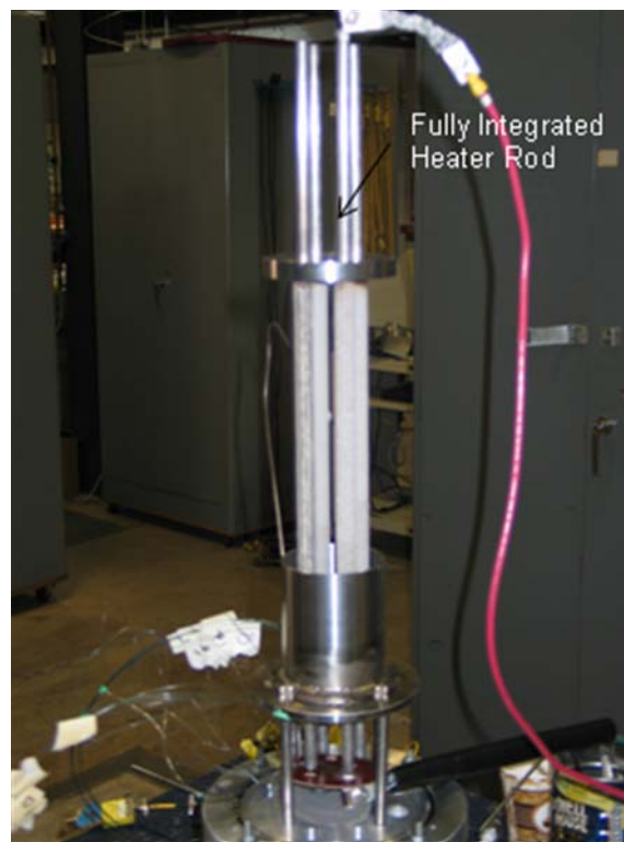
Figure 9: Internally heated test configuration
