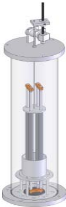
Figure 11: The motor-driven mechanism to position the wick assembly
