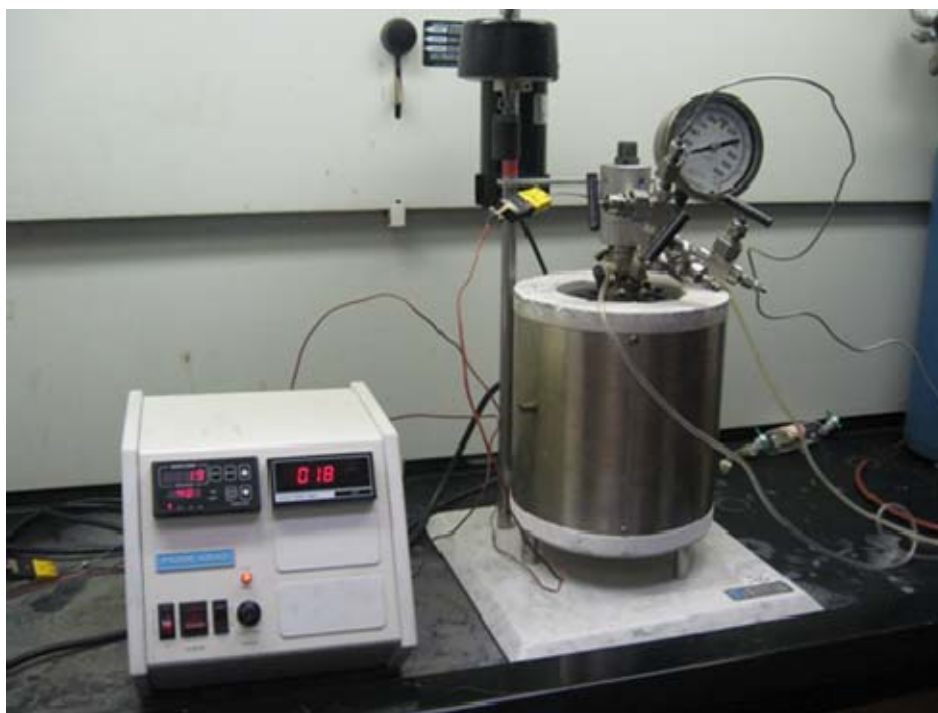
Figure 6. High temperature-high pressure reactor used in heavy oil conversion
