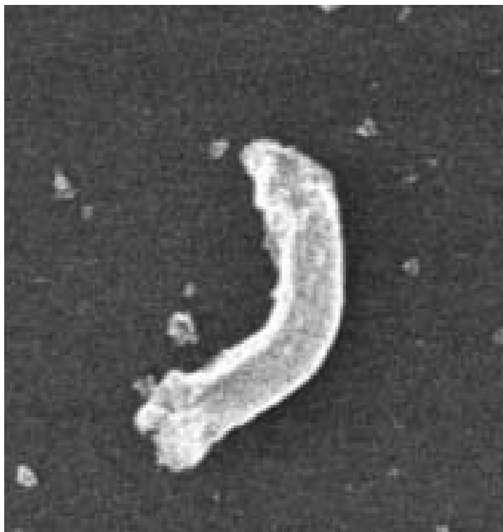
Figure 22. SEM pictograph of SBA-15/ZY synthesized from 3.0 g of 24 hr aged ZY precursor.
