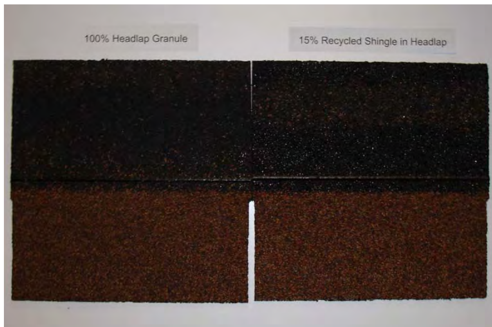
Fig. 6: Picture showing headlap portion of a shingle made with (a) standard headlap granule and (b) 15%wt recycled shingle -8/+20 mesh size.
