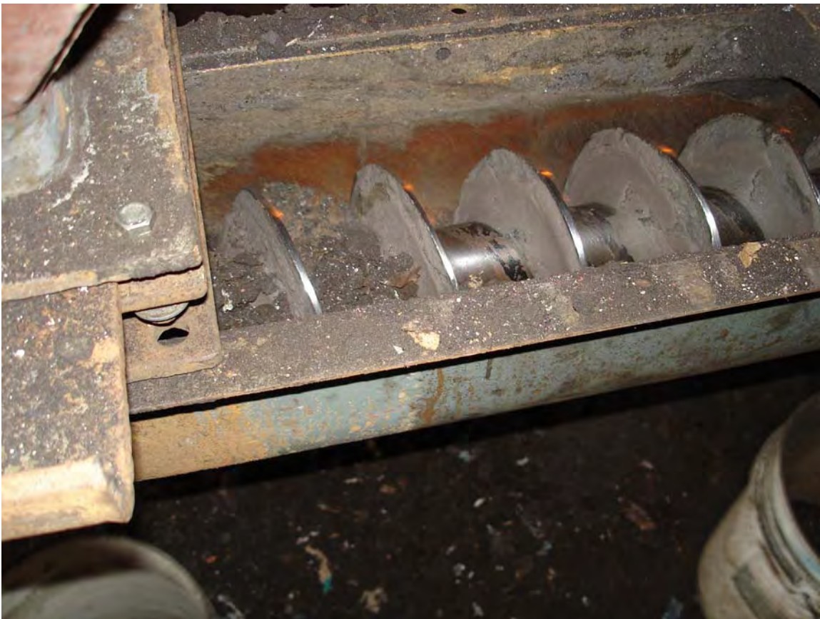
Shingle Feed Screw Figure 3
