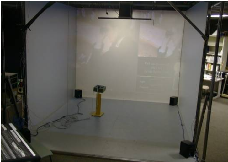
Fig. 2. The CAVE's visual and audio output hardware.
