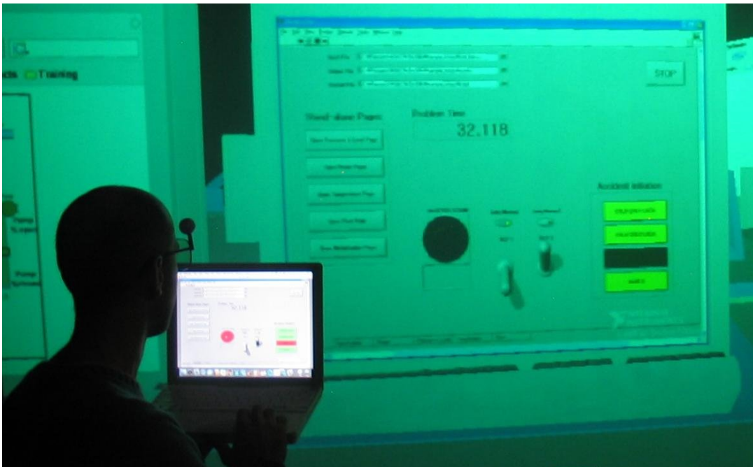
Figure 5. Picture of the virtual control room. One of the screen displays color-coded void fraction distribution in the reactor
