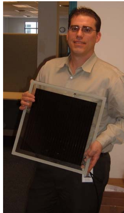
Figures 6 and 7: Pictures of encapsulated modules. The edge seal around perimeter and series interconnection lines are visible.
