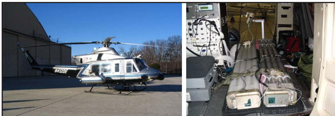
Figure 1. Bell 412 helicopter with AMS external gamma detector pods (left) and the two neutron modules mounted on the helicopter's floor (right)
