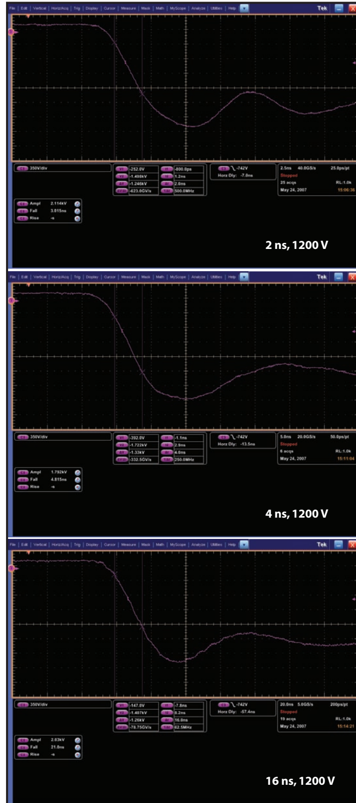
Figure 1. Three fastest sweeps (2 ns, 4 ns, and 16 ns) from negative ramp board, switching 1200 V. Filters can be designed to run longer than 40 ns.
