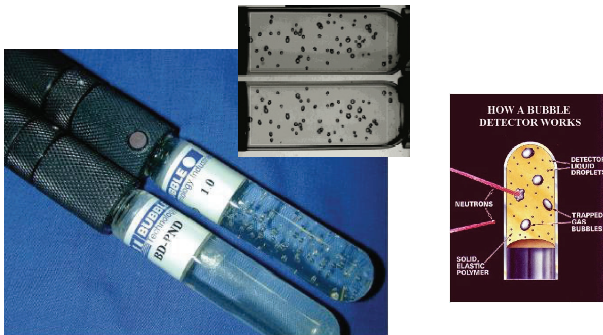
Figure 1. (left) BTI's Defender neutron detector; inset shows bubbles formed after neutron exposure; (right) Elastic scattering of incident neutron with fluorine atoms in a superheated liquid droplet vaporizes the droplet to form a gas bubble.
