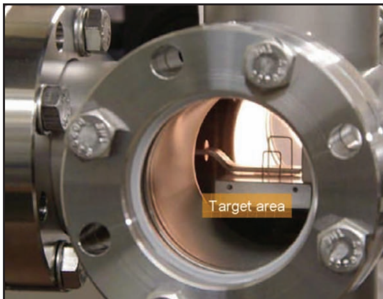
Figure 1. Plume generation area with alignment loops and movable aluminum target at base of the loops. The plasma generation laser enters through the top arm of the vacuum chamber.
