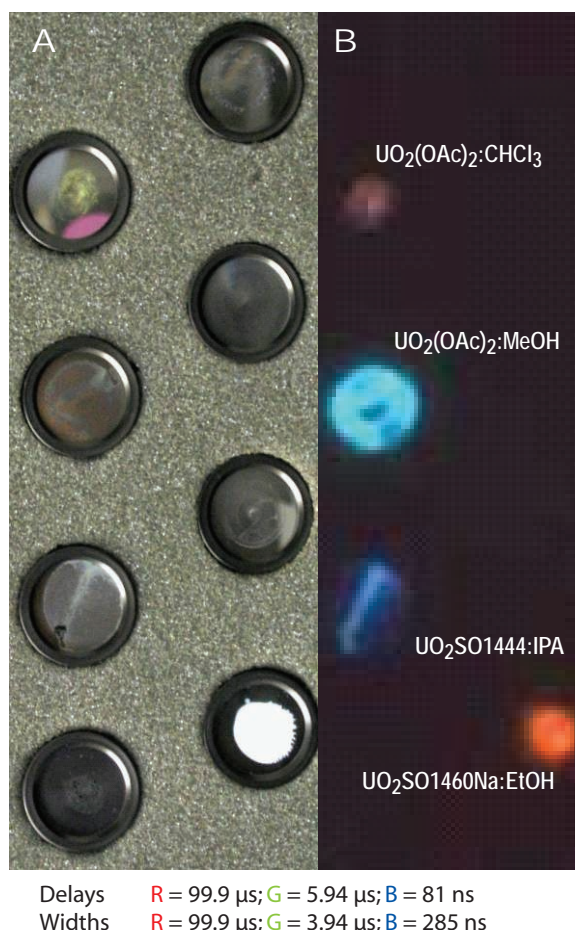
Figure 4. (a) Photograph of test samples and (b) LIFI imagery. Panel is a false-color composite (RGB), with the red (R) given from the longest band (delay = 99.9 \mu s, width = 99.9 \mu s), green (G) at 5.94 \mu s and below, and blue (B) from the shortest/earliest band (d = 81 ns, w = 285 ns).
