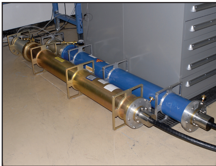
Figure 2. Supersaver Marx banks. The Supersaver is a 37-stage, 8.1-nF-per-stage, 150-joule Marx bank. It delivers a 400-kV, 35-ns pulse to the load.
