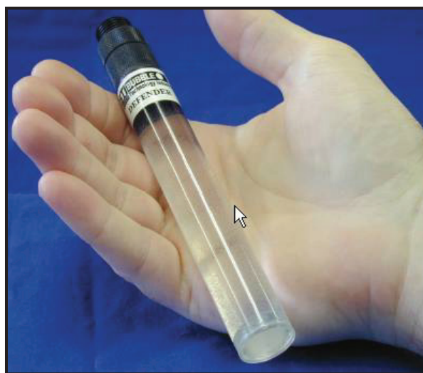
Figure 3. BTI Defender: ultra-sensitive formulation in personal dosimeter format (~1000 counts/mrem, 100 counts/ \mu Sv)
