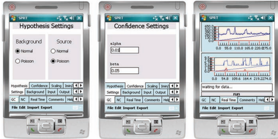
Figure 2. Selected screen captures of the software prototype for RSL in-house radiation detector; (left) hypothesis settings, (center) confidence settings, (right) execution window.
