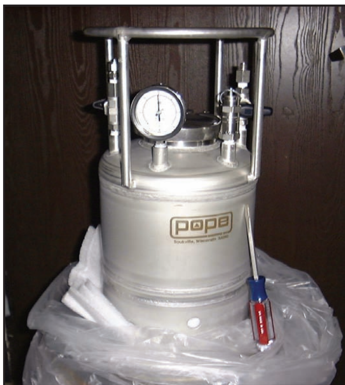
Figure 4. Pope 200+ psi pressure vessel for BTI gel bubble detector storage and reset
