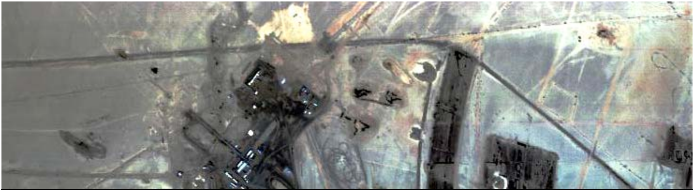
Figure 19. HyperSpecTIR data acquired by Sierra Nevada Corporation, 4-26-05. Cessna 404 Twin Engine Aircraft flying at 2000 feet AMT, 2 meter data, HST-2 sensor, at 120 Knot speed, 483, 554, 648 nm, BGR, gaussian stretch.
