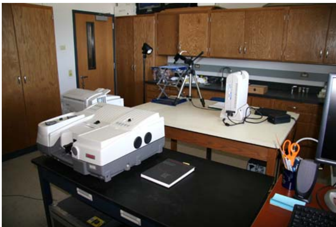
Figure 2. ABL Spectroscopy Laboratory showing Thermo/Electron FTIR Optical Spectrometer in foreground and ASD Full-Range Field Spectrometer in the background.
