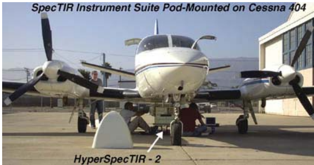
Figure 26. Sierra Nevada Corporation Cessna 404 with instrument pod and showing installation of HST-2 instrument for April 28, 2005 overflight.
