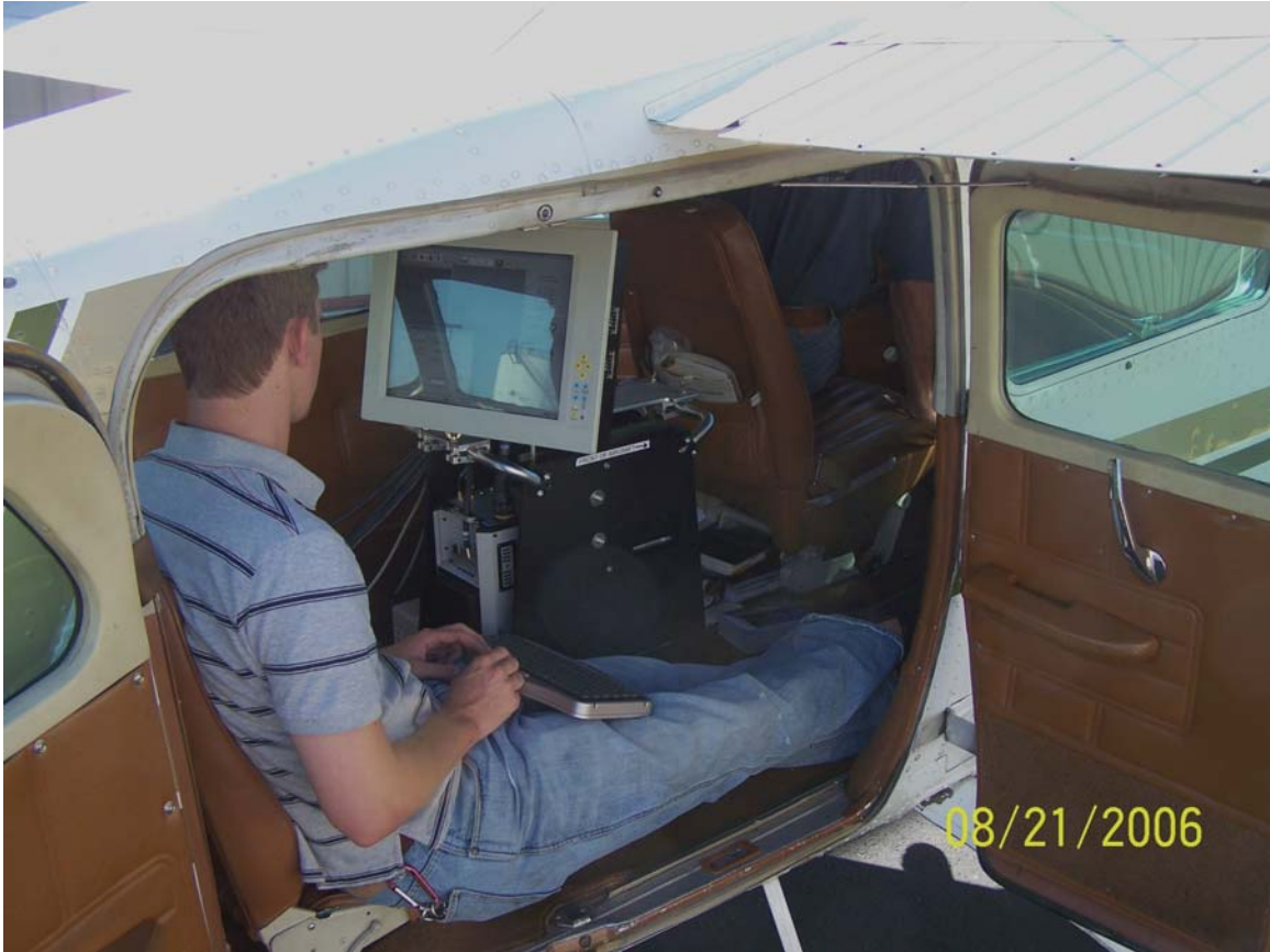
Figure 48. Operator and ProSpecTIR in Cessna 206. Sensor system is mounted in vibration isolation to the floor of the aircraft, but is not in a pitch, yaw and roll stabilized mount.
