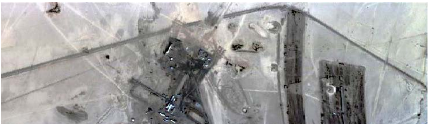
Figure 20. HyperSpecTIR data acquired by SpecTIR Corporation, 9-28-05, Cessna 206 Single Engine Aircraft flying at 2000 feet AMT, 2 meter data, HST-3 sensor, at 80 Knot speed, Bands 479, 549, 656 nm, BGR, Gaussian stretch.
