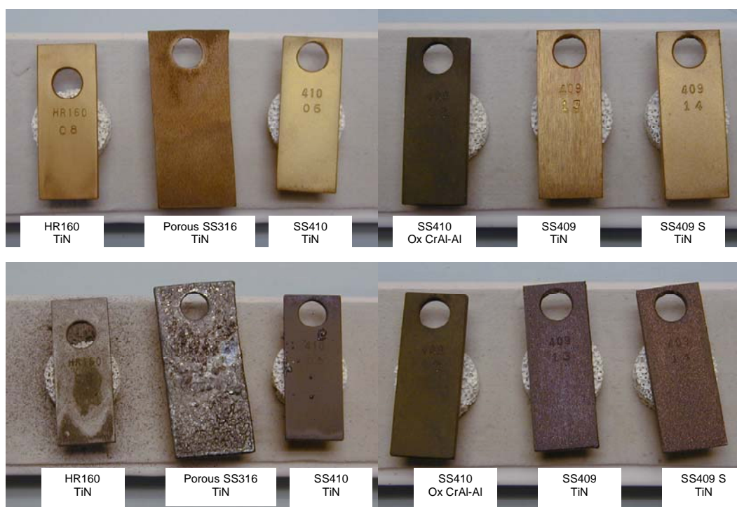
Figure 24. Samples from Test #7a before and after exposure to simulated gasifier environment for 96 h.
