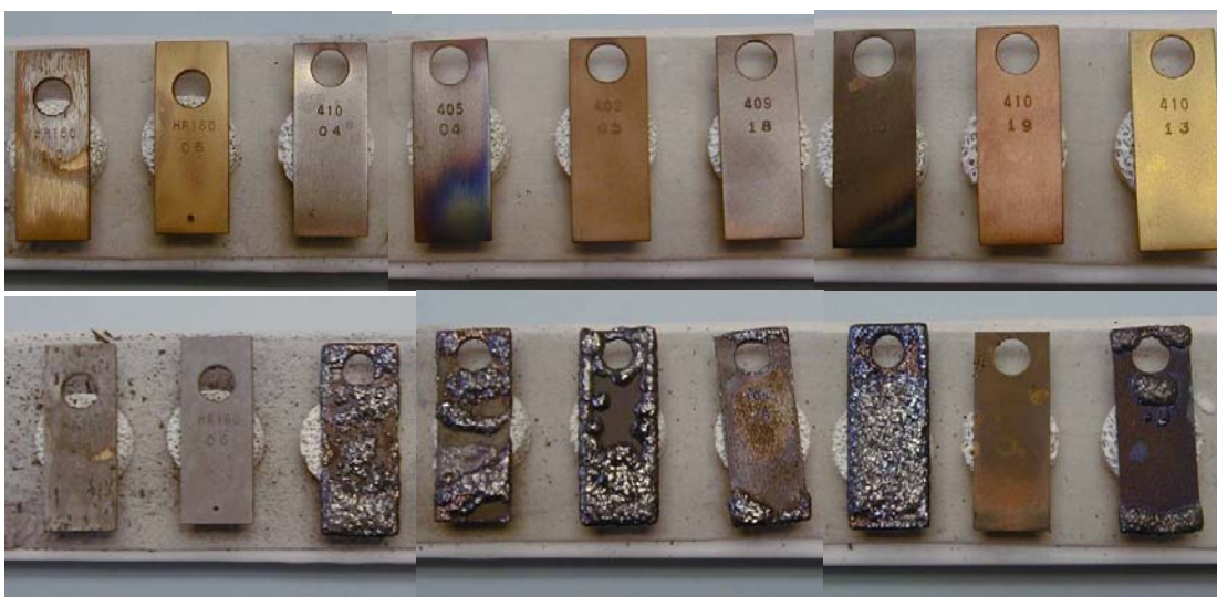
Figure 26. Samples before and after exposure for 306 h at 900°C to a simulated coal gas in Test #9a.
