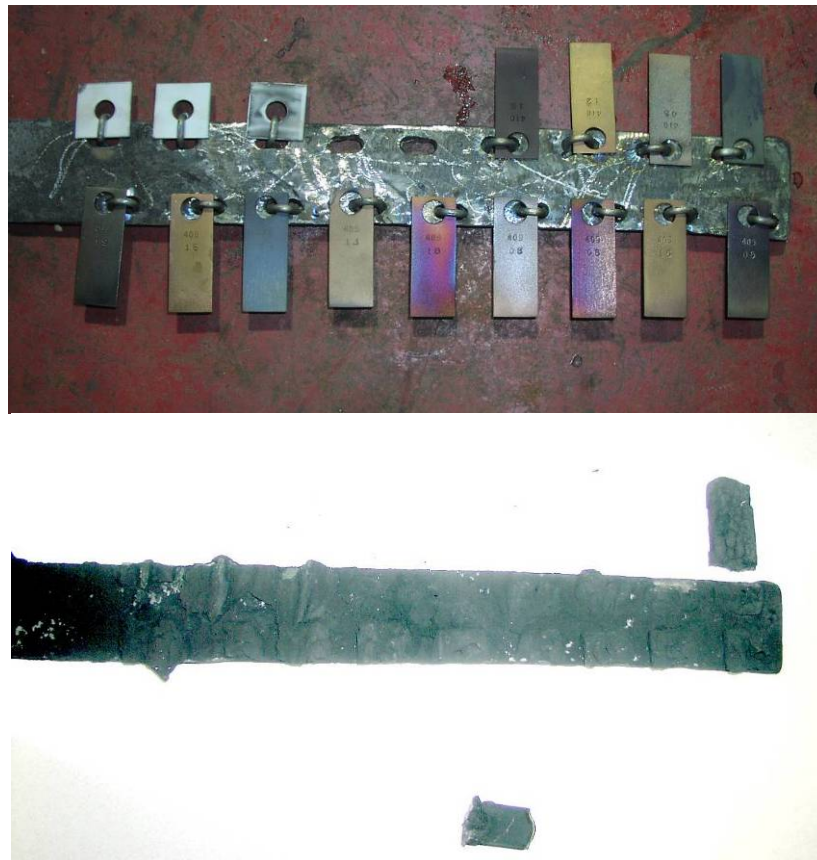
Figure 64. Samples before and after exposure to the hot gas stream in the Wabash River Plant during May-Sep, 2005 (3,814 h)
