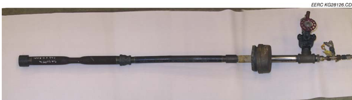
Figure 5-6. Photograph of the corrosion/deposition probe assembly.
