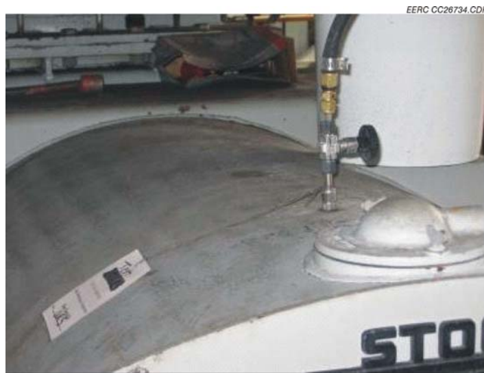
Figure 3-2. Stock feeder deck (top) and insertion of halogen feed line into top of stock feeder for MoSES Unit 3.
