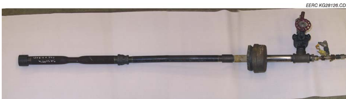
Figure 4-1. Photograph of the corrosion/deposition probe assembly.
