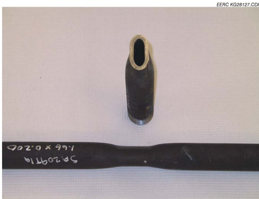
Figure 5-7. Photograph of coupon and a cross-sectioned coupon.
