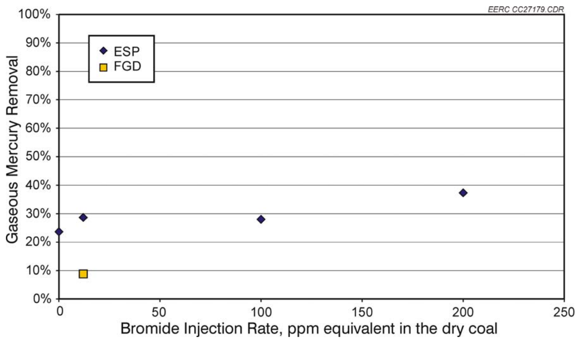
Figure 4-9. Mercury removal across the ESP and FGD for \text{CaBr}_2 during parametric injection tests at MoSES.
