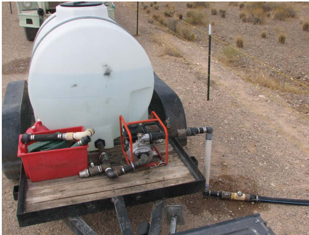
Figure 2-11. Trailer Mounted Tank with Pump and Manifold
