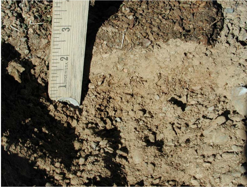
Figure 2-6. Field Emulsion Penetration Test
