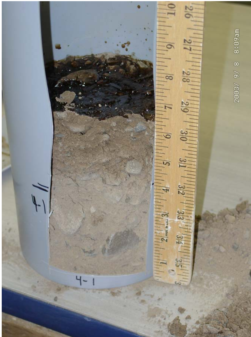
Figure 2-5. Laboratory Emulsion Penetration Test
