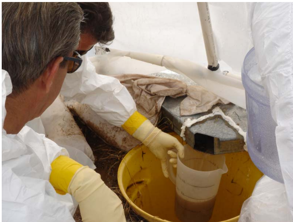
Figure 2-17. Collection of Runoff from Test Plot
