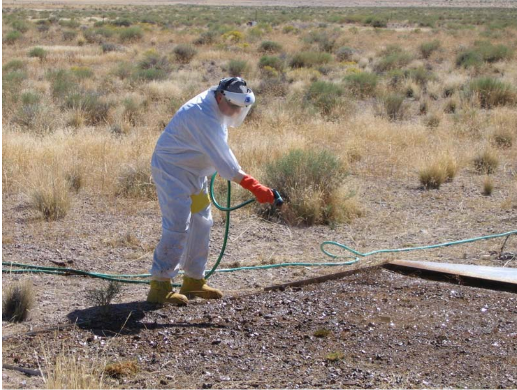
Figure 2-12. Application of the Encapco Emulsion to Test Plot
