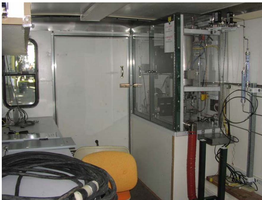
Figure 7 – S Zorb™ SRT Slipstream Test Unit Installed in Mobile Trailer
