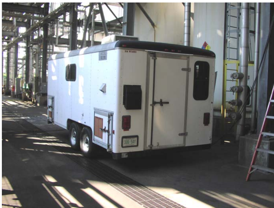
Figure 8 –S Zorb™ Slipstream Test Mobile Trailer Unit Installed in SGS Facility
