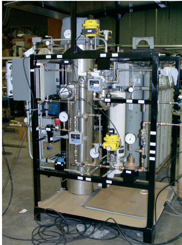
Figure 3 –Photograph of Bench-Scale Slipstream Unit - Metal Oxide Impregnated Carbon
