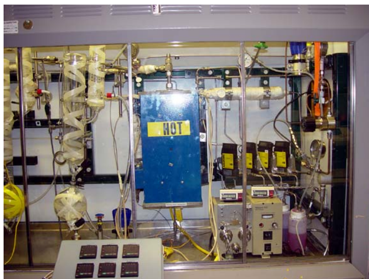
Figure 6 – Photograph of COP S Zorb SRT Warm Gas Desulfurization Laboratory Unit
