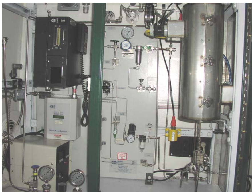
Figure 6 – S Zorb™ SRT Slipstream Test Unit Installed in Mobile Trailer
