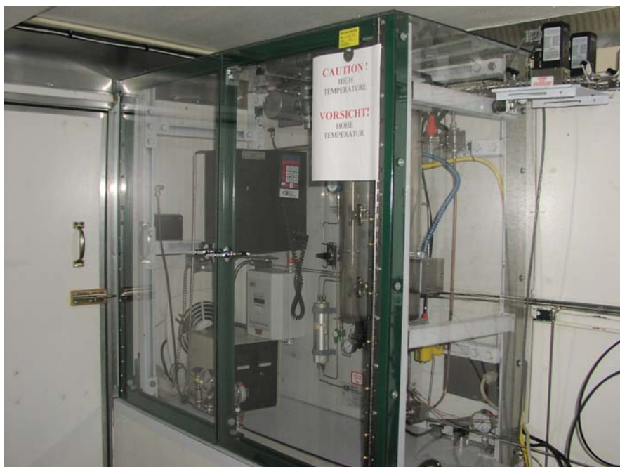
Figure 5 – S Zorb™ SRT Slipstream Test Unit Installed in Mobile Trailer
