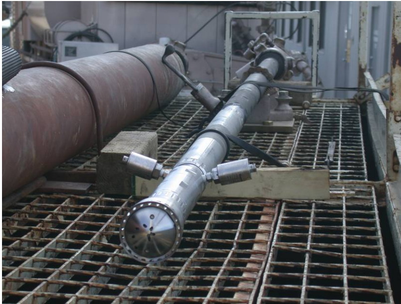
Figure 14. Microhole jet drilling bottomhole assembly mounted on top of water supply tank with pressure transducers attached.
