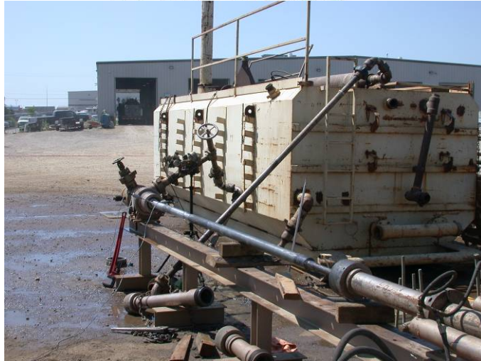
Figure 10. Horizontal test chamber and recirculation tank at Trican's Red Deer yard. Test chamber is setup for Microhole instrumented performance tests.
