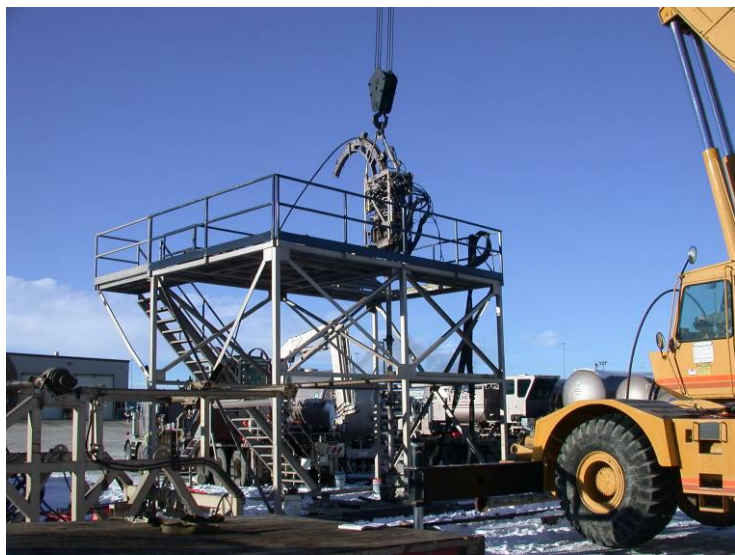
Figure 13. Trican test well with injector and lubricators installed. Head frame was removed for last yard test.
