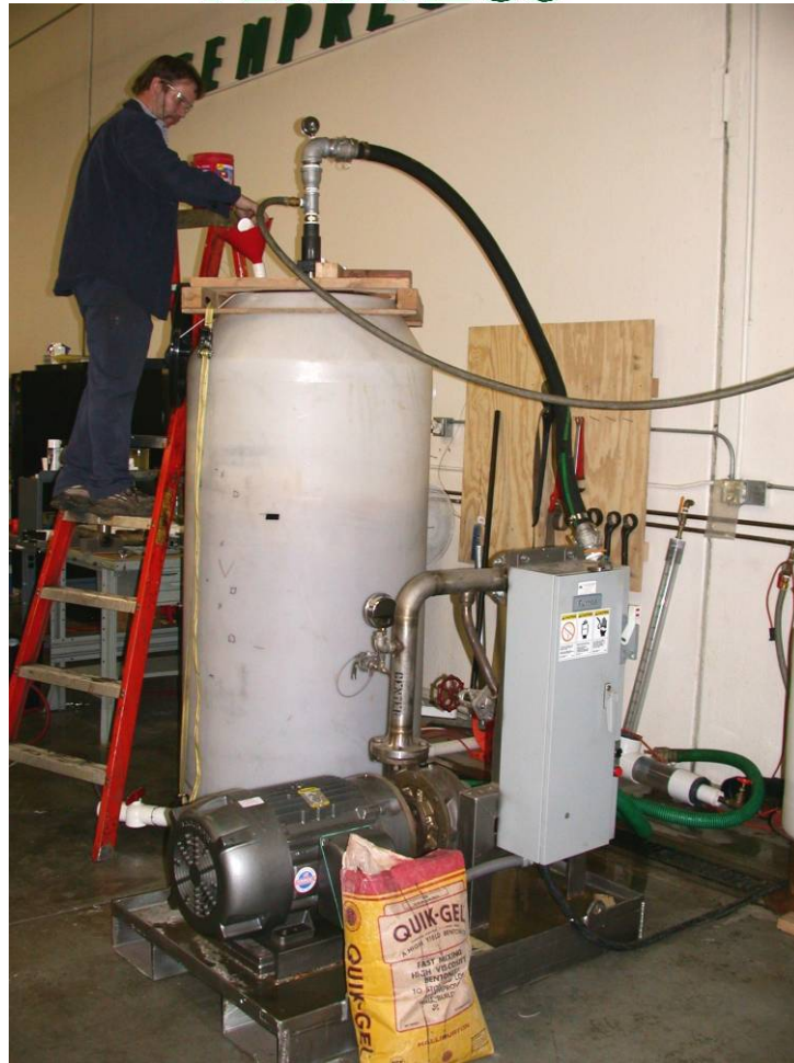
Figure 9. Dirty water circulation test with gas separator.
