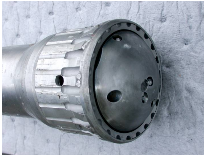
Figure 2. 6-jet nozzle head and gage ring.
