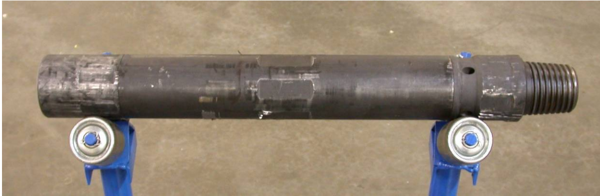
Figure 7. 2.875" Commercial Motor Gas Separator (patent pending).
