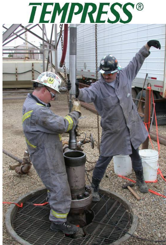
Figure 12. Microhole BHA being inserted into shallow test well at Trican’s Red Deer yard
