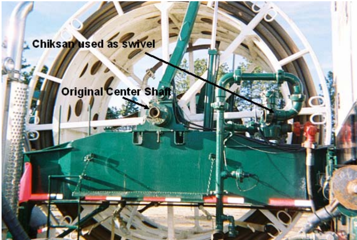
Figure 10-7 Coiled Tubing Reel prior to modifying reel swivel and manifold
