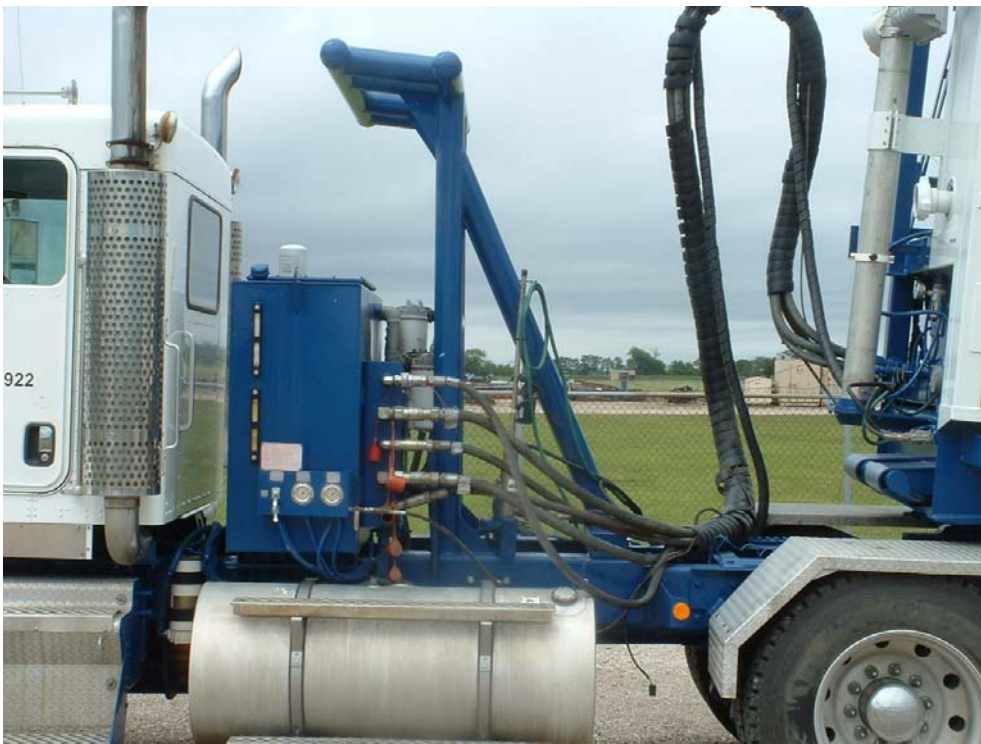
Figure 10-22 Pipe handling tractor after installing roll bar
