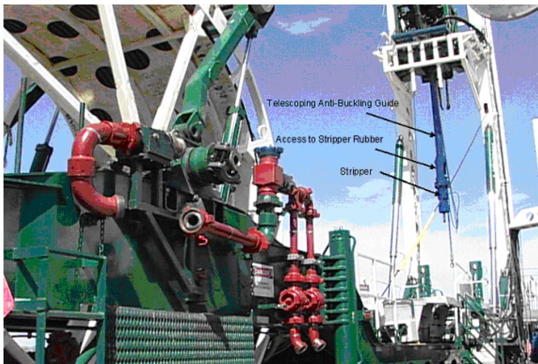
Figure 11-4 Installation of Telescoping Anti-Buckling Guide
