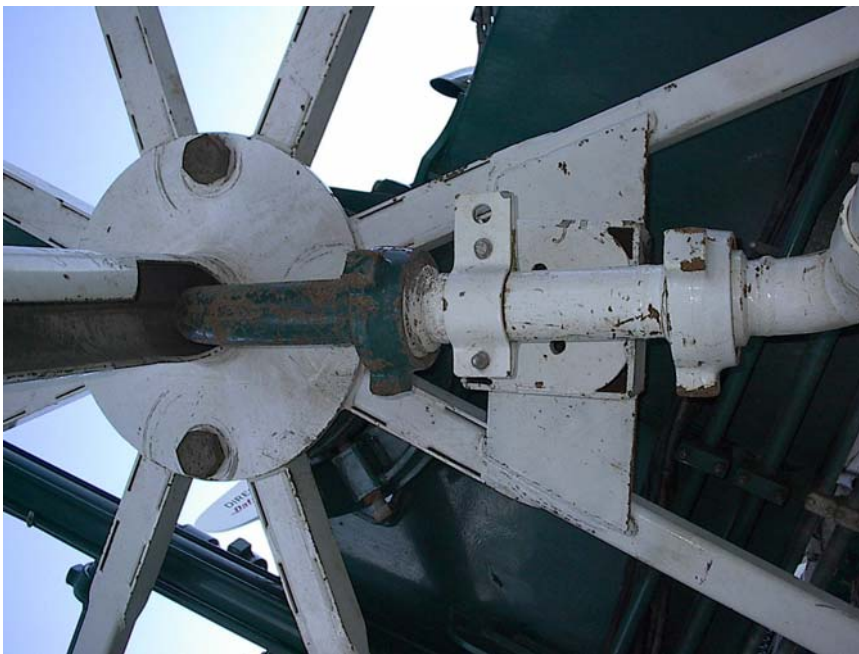
Figure 10-6 Showing original reel center shaft, which connected to external swivel treating iron
