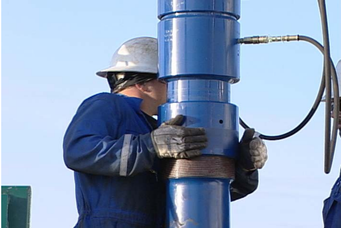
Figure 11-7 Connecting Telescoping Anti-Buckling Guide to Lubricator Cont'd
