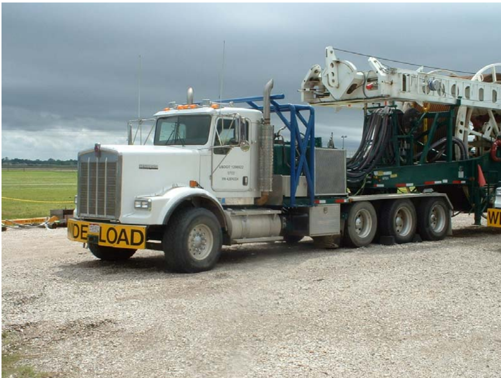
Figure 10-24 Mast unit tractor after installing roll bar
