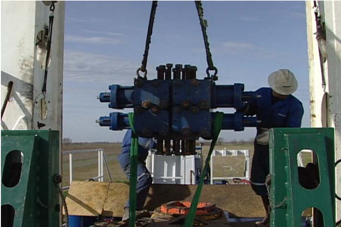
Figure 13-8 Preparing to lower 7-1/16" Combi BOP onto well
