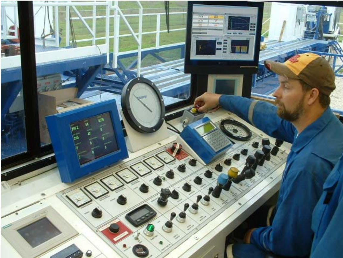
Figure 12-7 Re-setting CoilSAVER after testing trip on test well
