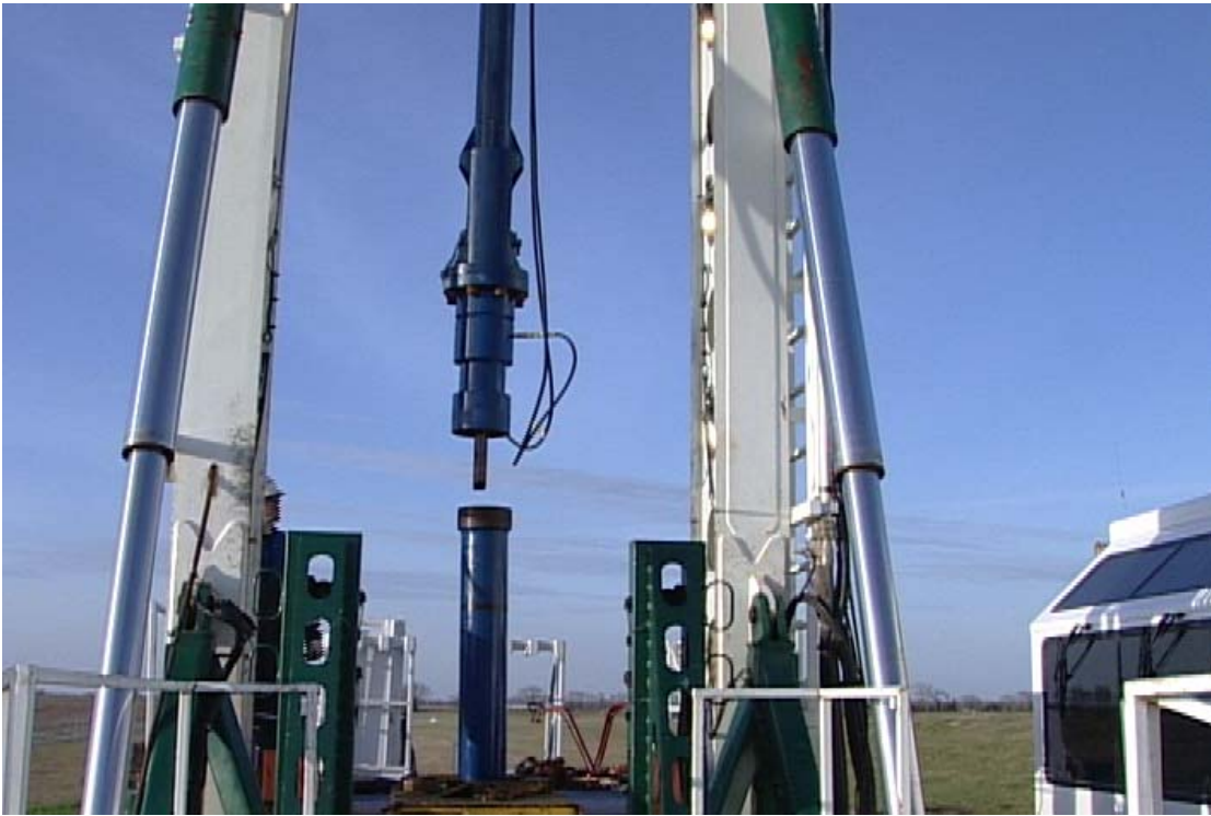
Figure 11-5 Connecting Telescoping Anti-Buckling Guide to Lubricator
