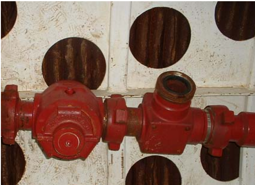
Figure 12-14 Internal Reel manifold with tee to connect pressure bulkhead
