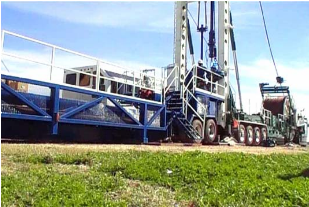
Figure 13-1 Starting to pull 4-1/2" completion from test well
