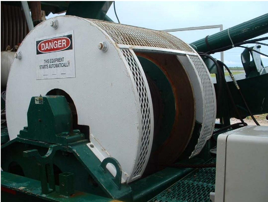
Figure 10-11 New drawworks cover with reinforced grating
