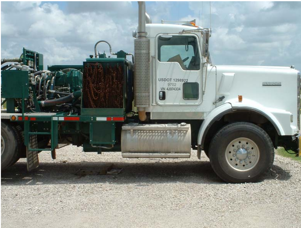
Figure 10-23 Mast unit tractor prior to adding roll bar
