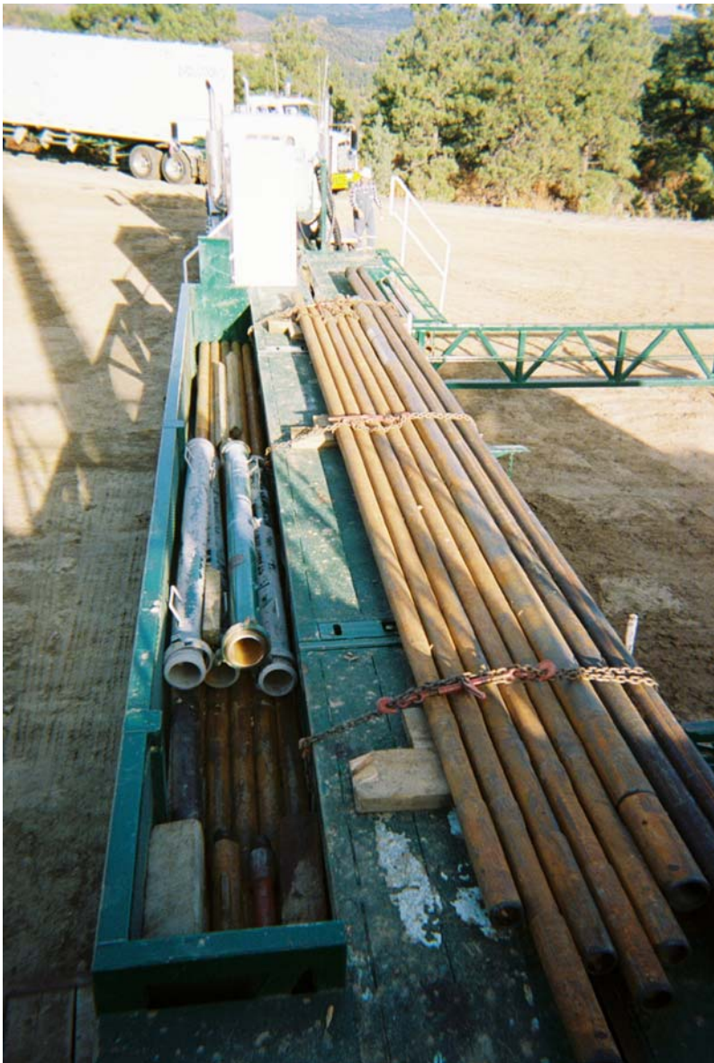
Figure 10-12 Pipe trailer prior to addition of hand rails
