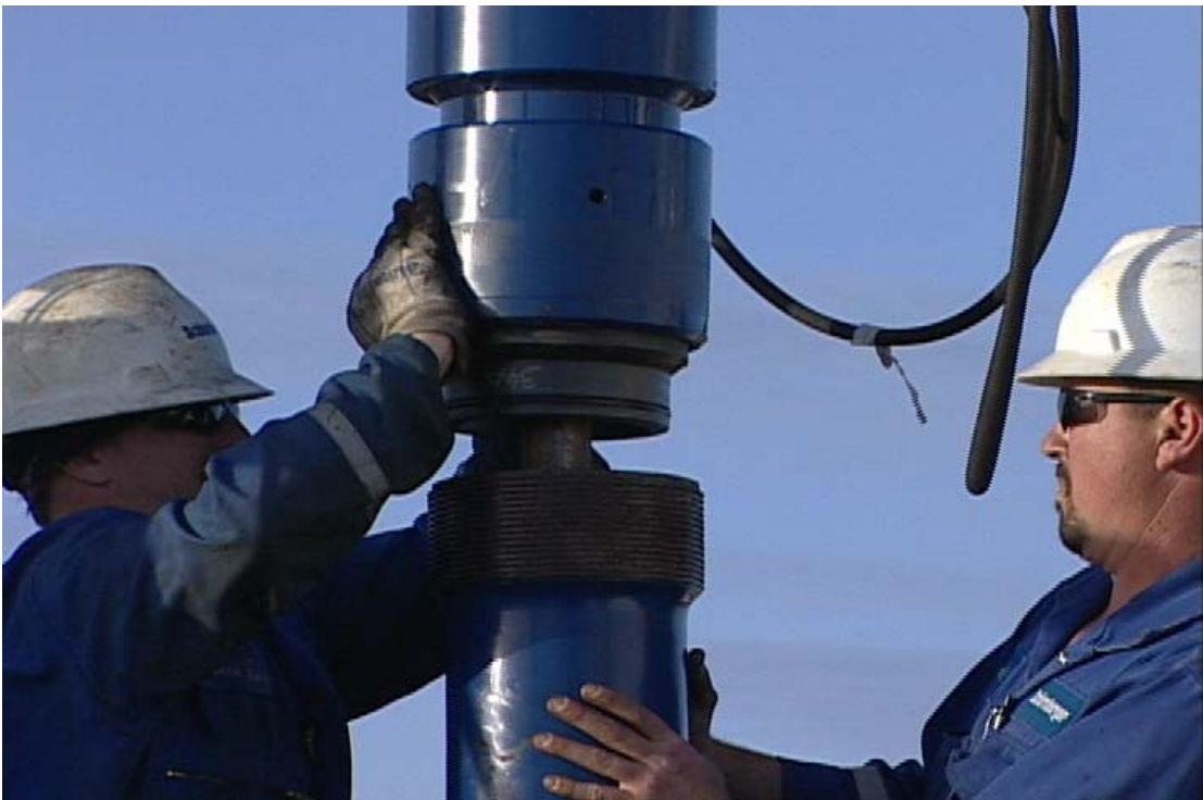
Figure 11-6 Connecting Telescoping Anti-Buckling Guide to Lubricator Cont'd
