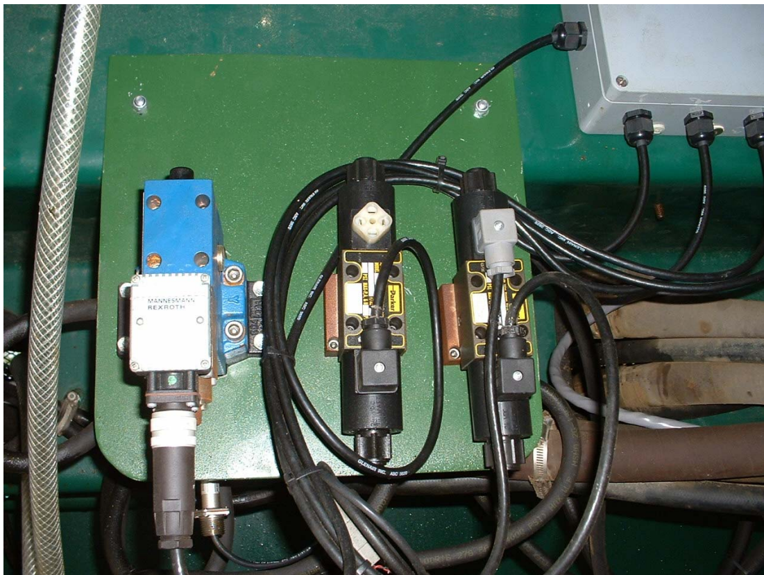
Figure 12-9 CTInSPEC Control valves mounted beneath floor
