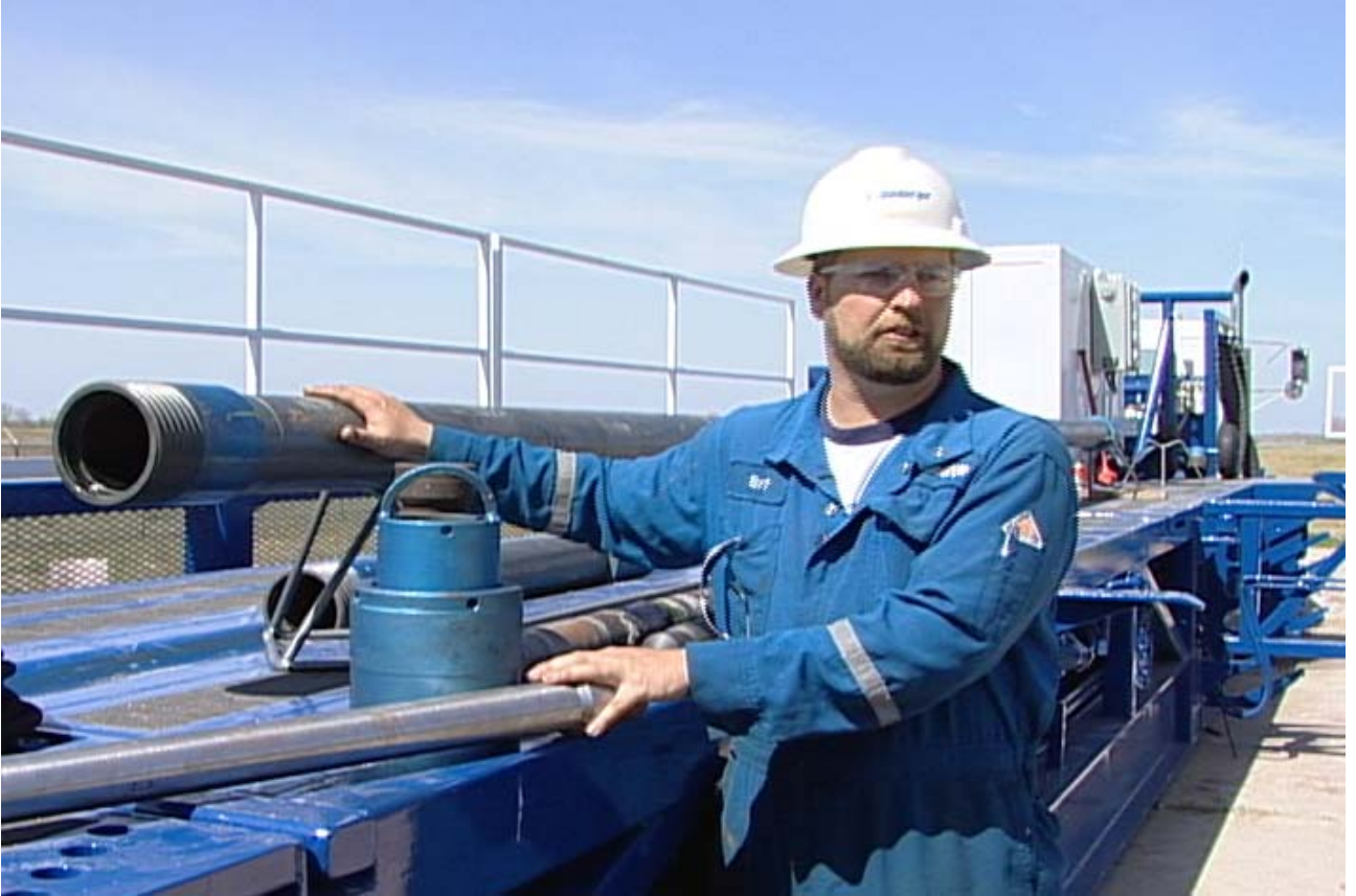
Figure 11-18 Slickline lubricator and deployment bar
