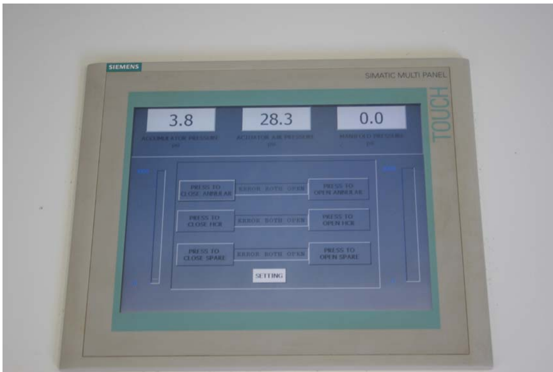
Figure 10-19 Original Main BOP Control Panel
