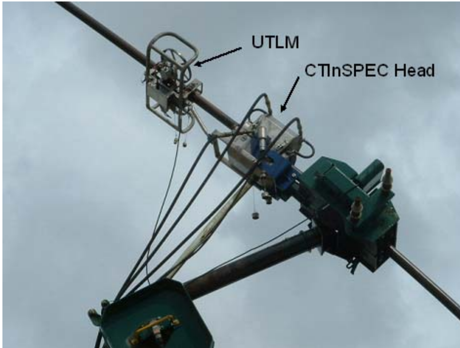
Figure 12-8 Installation of CTInSPEC on pipe
