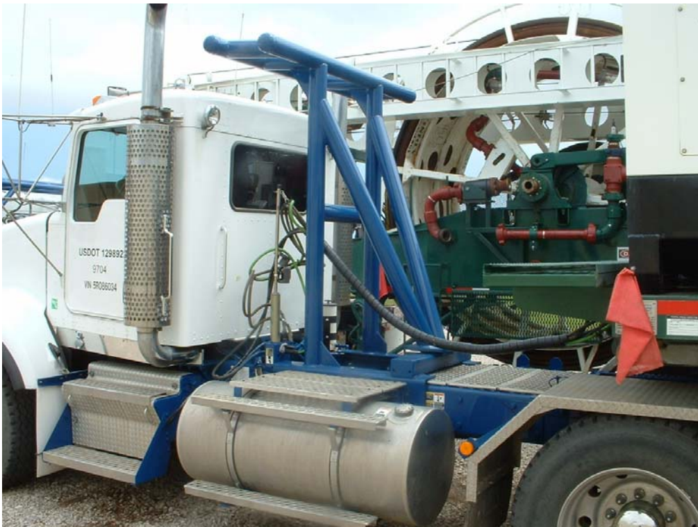
Figure 10-26 Control cabin tractor after installing roll bar
