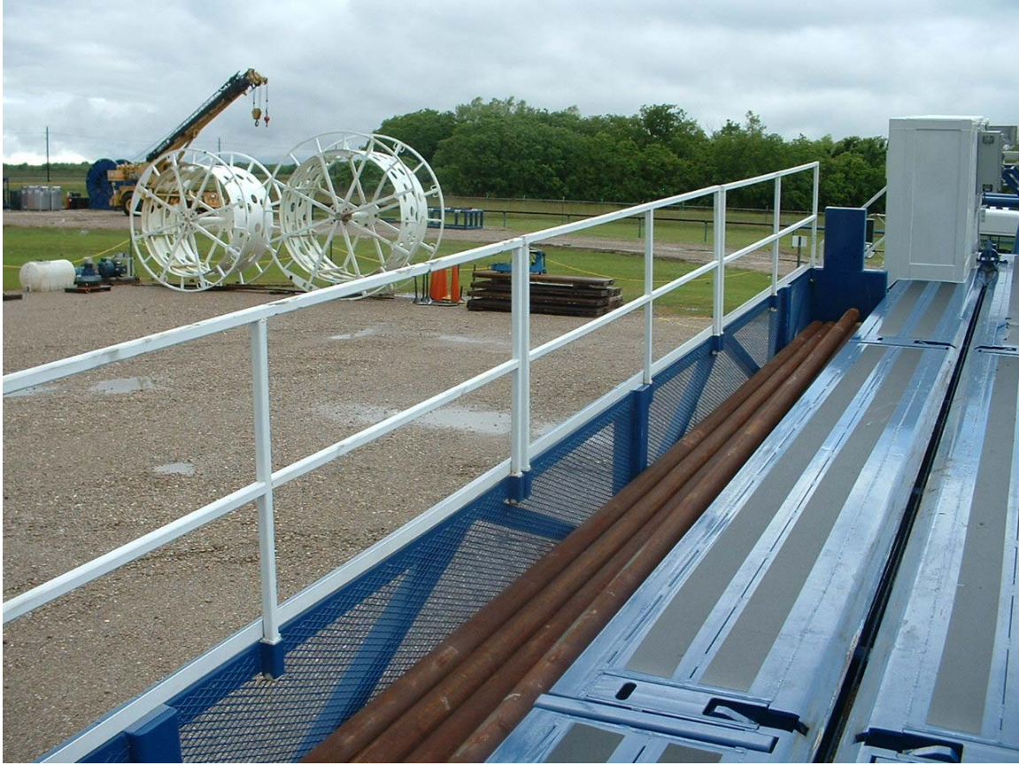
Figure 10-13 Addition of hand rails to pipe trailer
