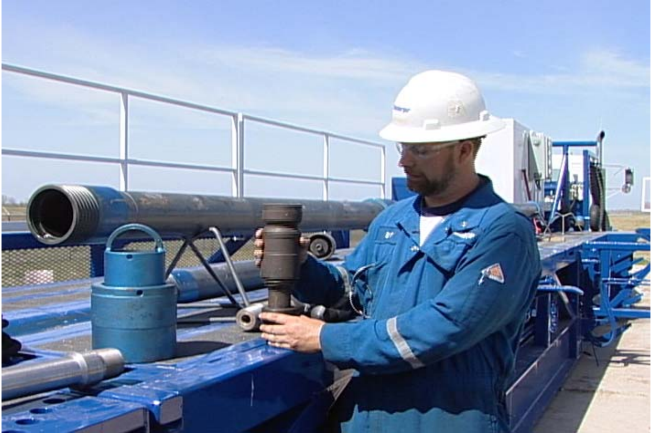
Figure 11-19 Demonstration of one type of non-rotational joint for connecting coiled tubing to the bottom hole assembly
