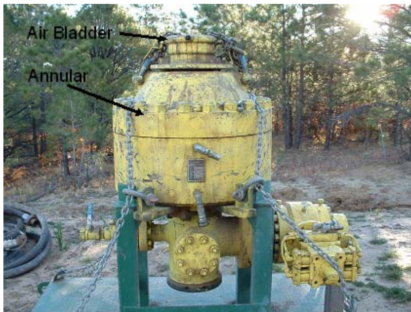
Figure 11-2 Annular with air bladder seal ring
