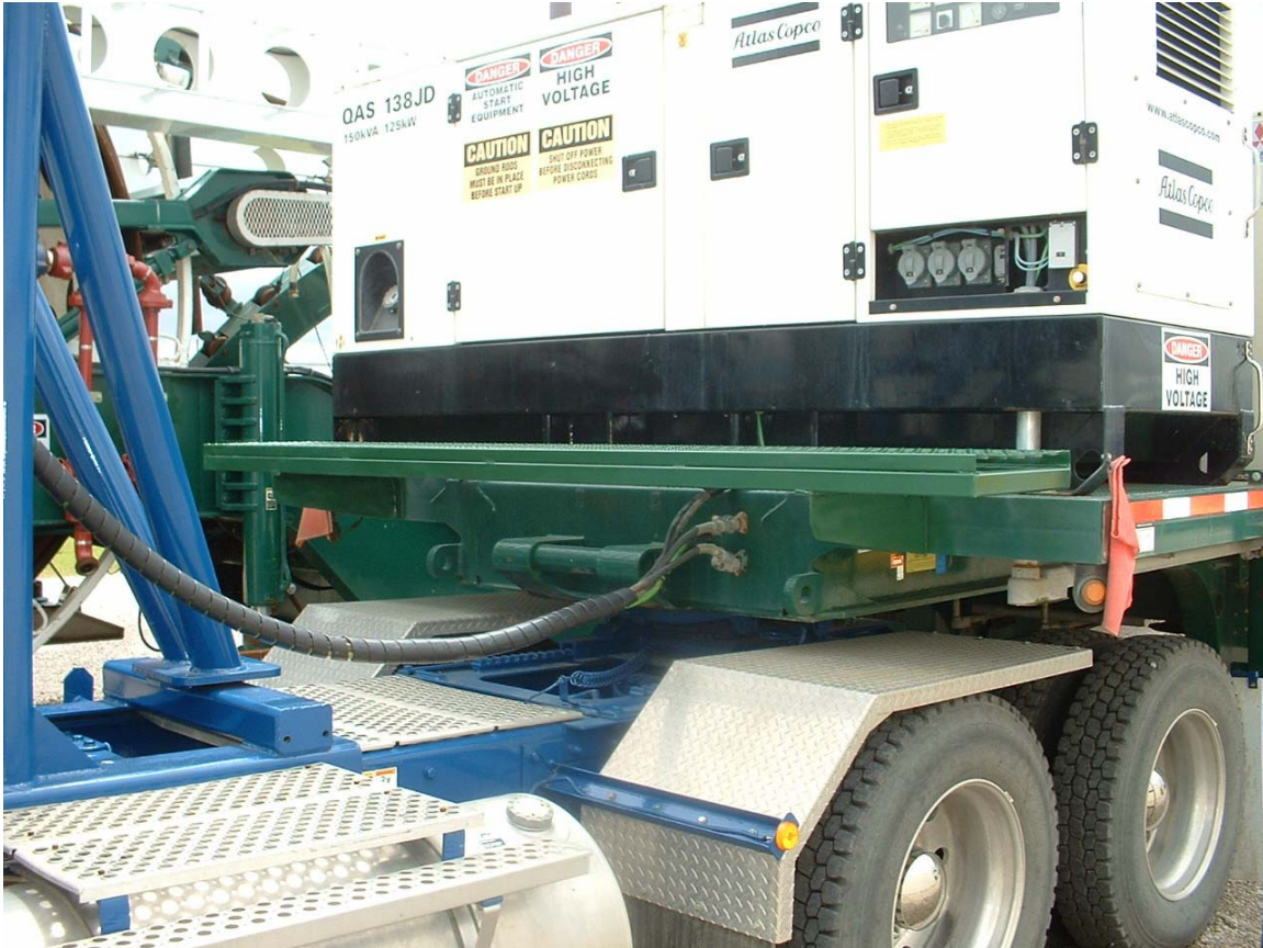
Figure 10-16 Work platform added to generator
