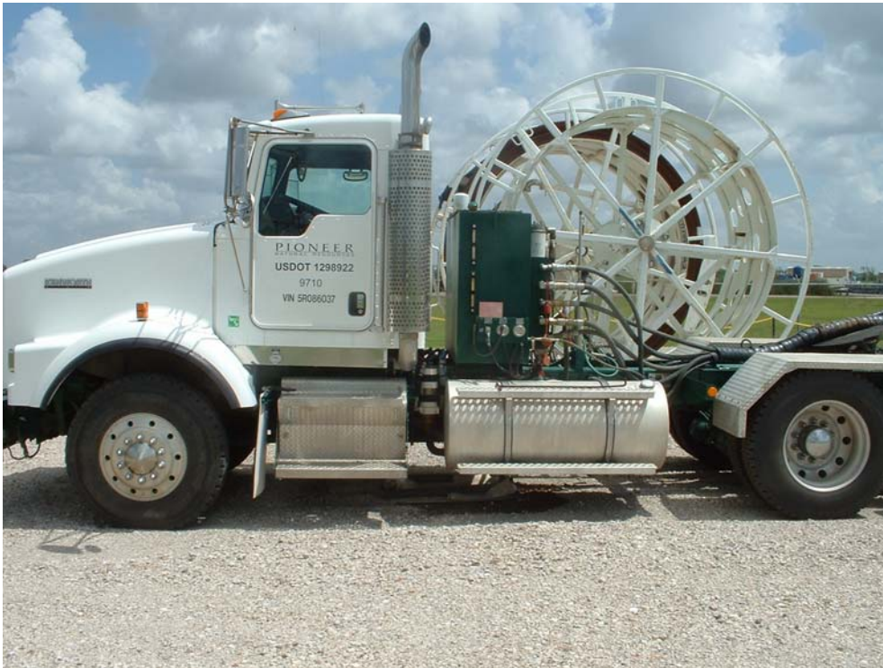
Figure 10-21 Pipe handling tractor prior to addition of roll bar
