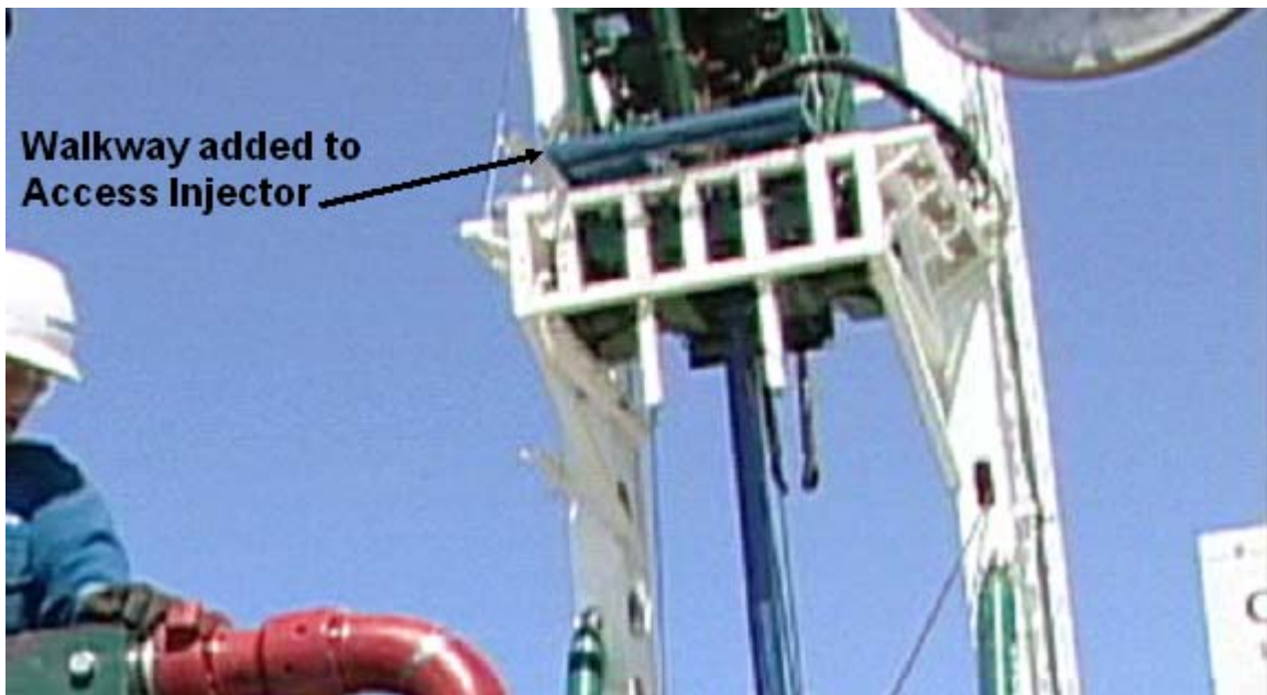
Figure 10-15 Shows location of work platform added to injector for ease of maintenance
