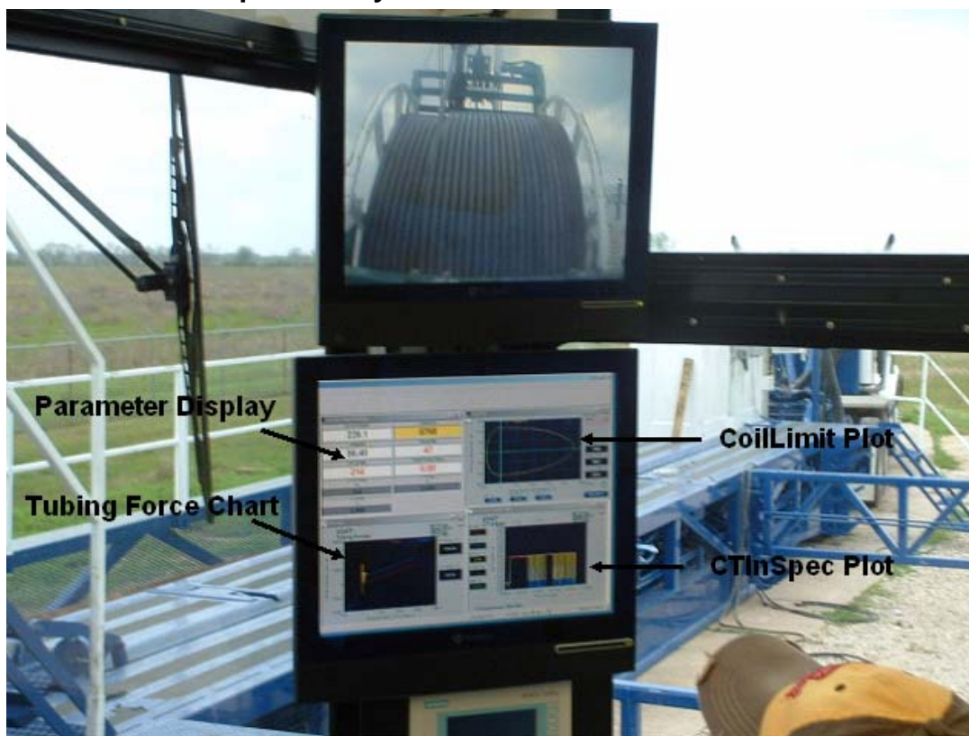
Figure 12-1 CoilCAT real time monitor for operator
