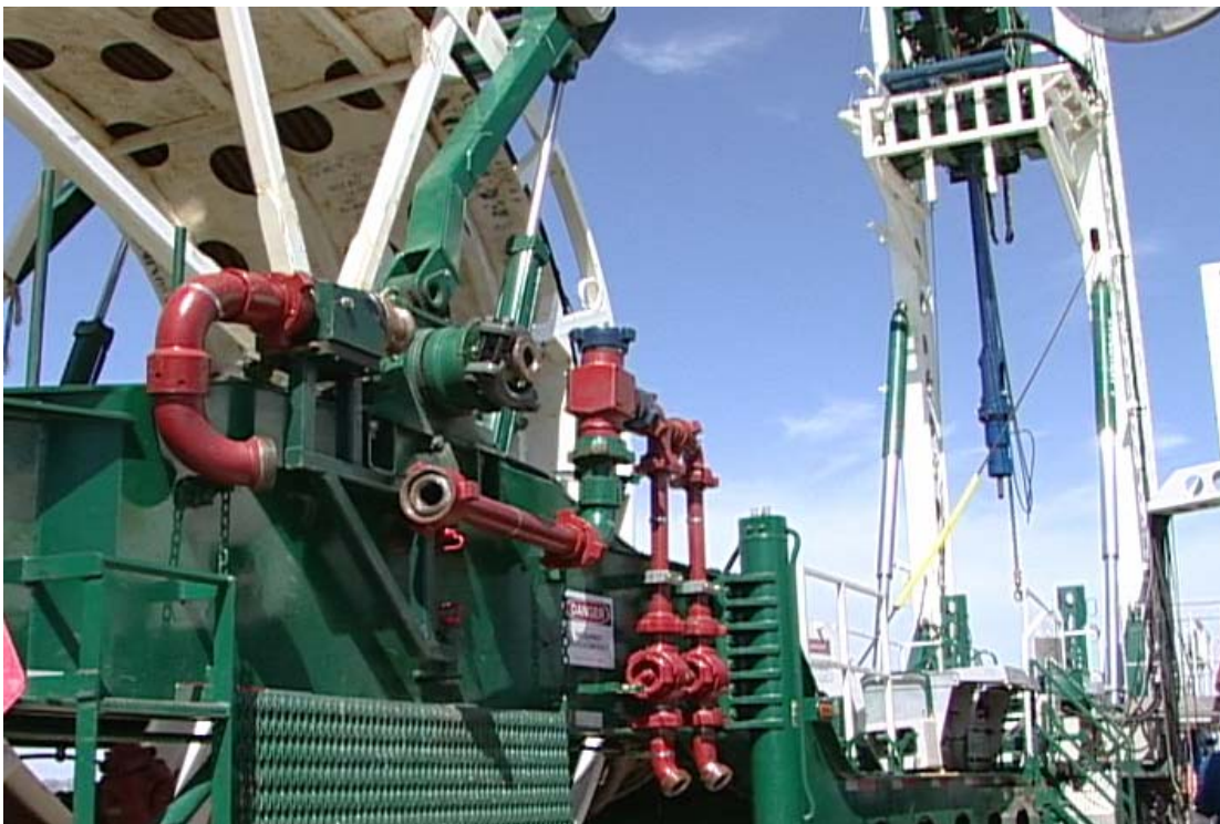
Figure 10-8 New manifold with swivel folded for transport
