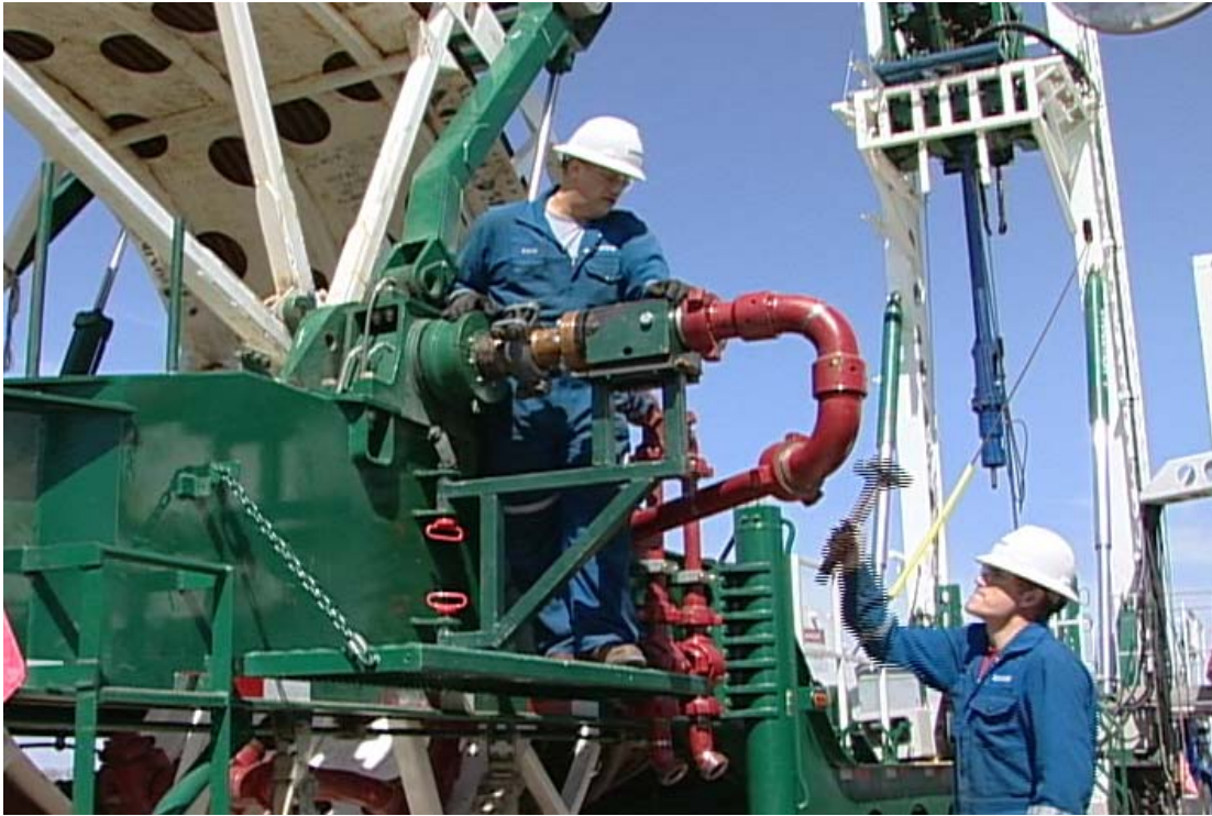
Figure 10-9 New external reel manifold with swivel assembled ready for job
