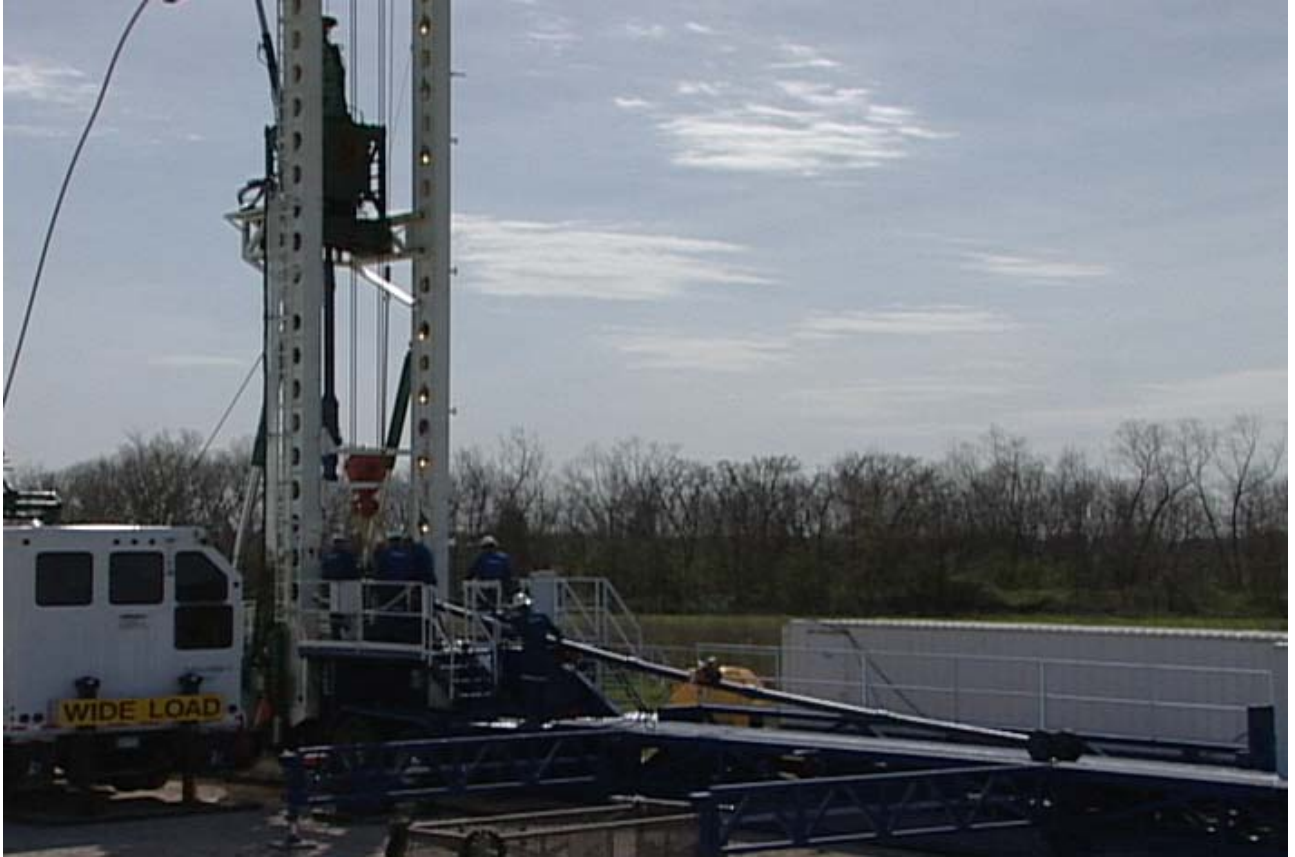
Figure 11-21 Raising slickline lubricator into derrick
