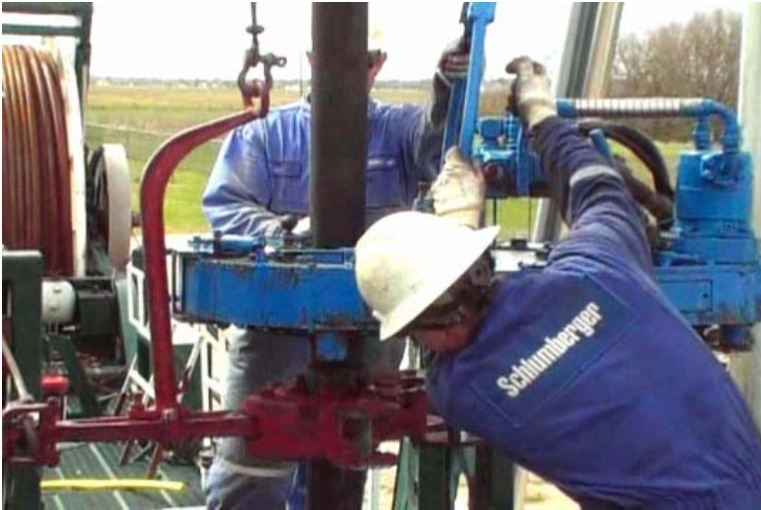
Figure 13-2 Breaking out a connection
