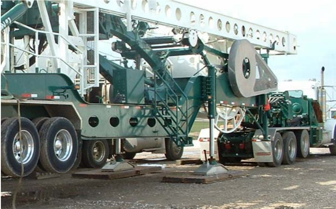
Figure 10-14 Rig stairs prior to adding additional step to reduce distance to ground
