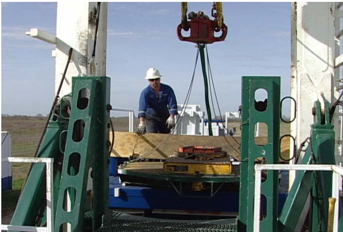
Figure 10-5 Floor being removed with blocks
