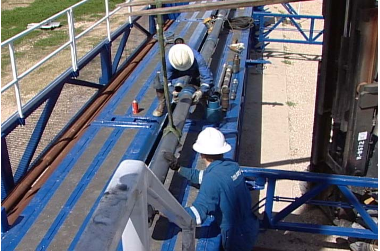
Figure 11-20 Assembling slickline lubricator on pipe trailer
