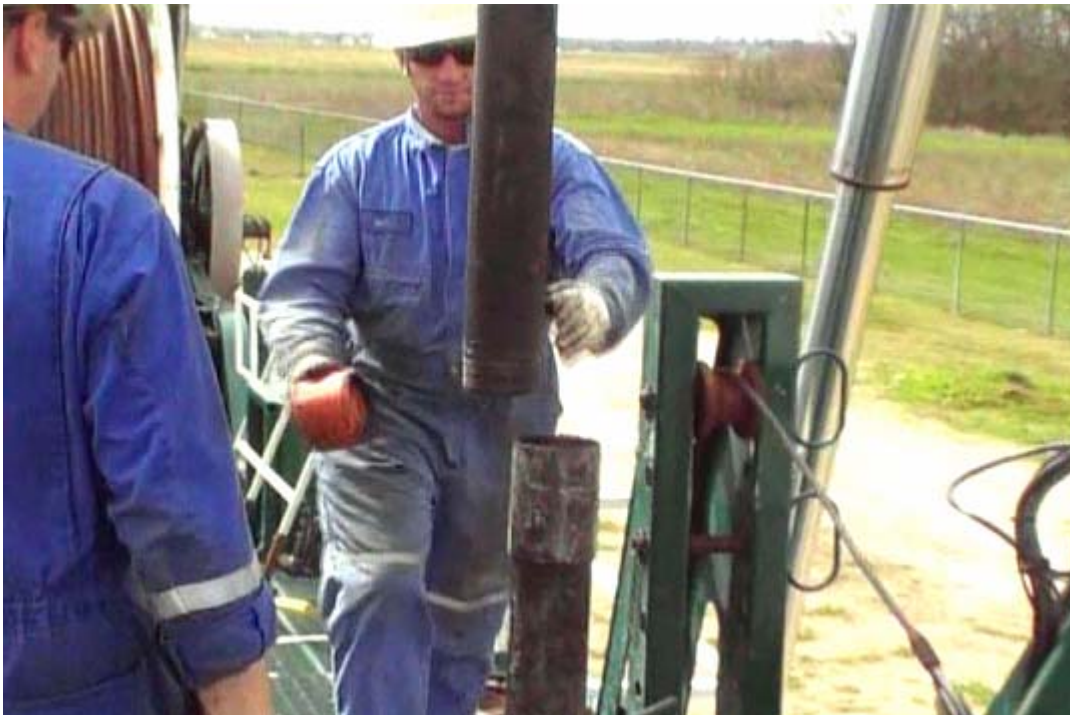
Figure 13-3 Connection broke out ready to lay down tubing
