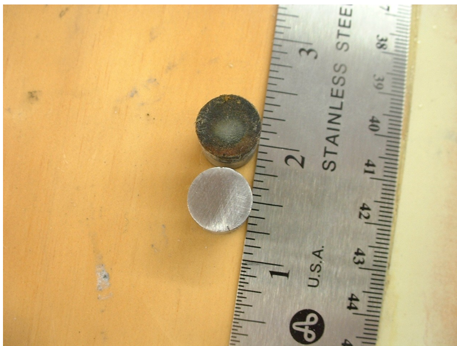
Figure 9: Electrolyte 494-3' Anode versus a Fresh Mg Anode.
