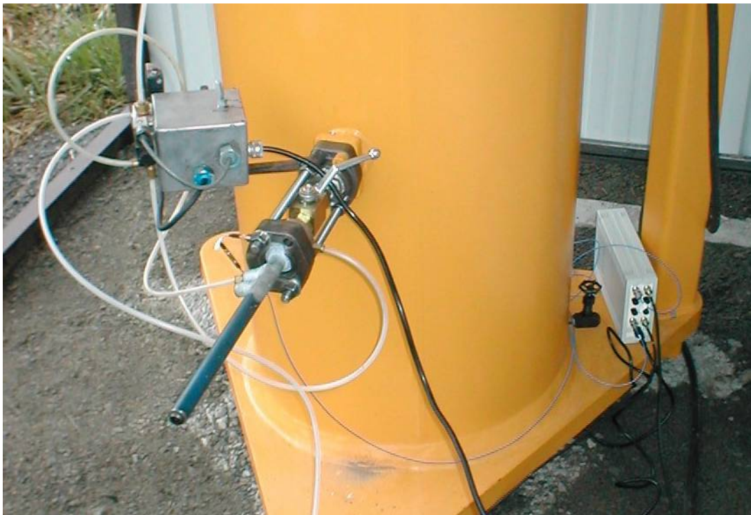
Figure 24. Reflected shock apparatus mounted on EGS1 pressure vessel.
