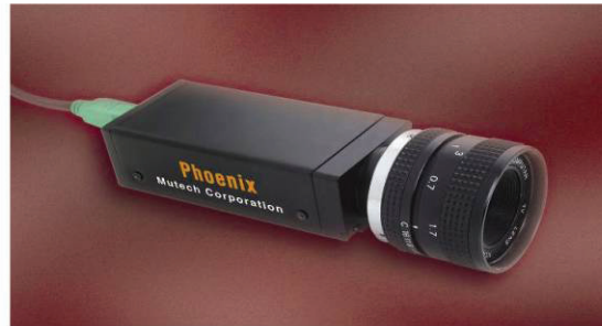
Phoenix USB 2.0 digital camera from MuTech Corporation. This camera was used to obtain digital pictures of the suspect objects when a radiological alarm would generate a software trigger for the camera. The camera resolution is low (a memory of 1.3 Megapixels) but it is appropriate for traffic monitoring. It was used to take the picture of the LPADC, below.
