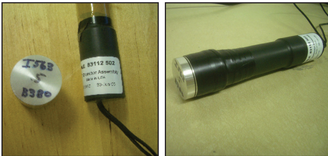
Figure 5. (left) \text{LaBr}_3\text{:Ce} fast scintillator crystal attached to a Burle Industries 1-in. fast PMT; (right) coupled crystal and PMT, tape-wrapped to prevent stray light input
