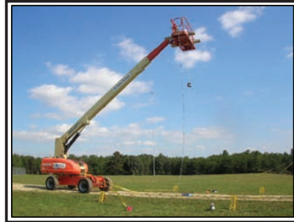
Figure 5. The ^{252}\text{Cf} source suspended at a fixed distance of 10 ft below the boom basket in a measurement to determine the scattering fraction from the ground surface
