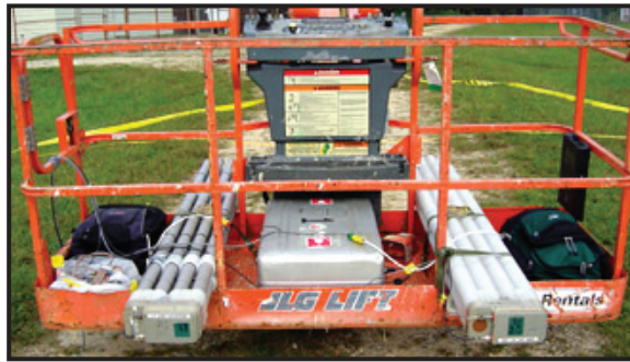
Figure 2. Two 6-ft ^3\text{He} module detectors extending lengthwise across the basket of the boom crane in the measurement geometry. The 6-ft module at left is unmoderated (bare); the module at right is moderated (tubes encased in polyethylene).
