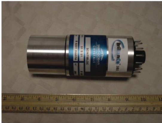
Brilliance 380 LaBr 3 :Ce crystal with its online PMT. The crystal is a 5.08 \text{ cm} \times 5.08 \text{ cm} cylinder requiring 496 VDC to operate.
