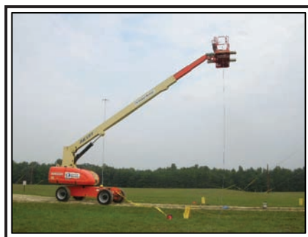
Figure 1. A boom-type crane was used to conduct source-to-detector measurements from 10 to 80 ft
