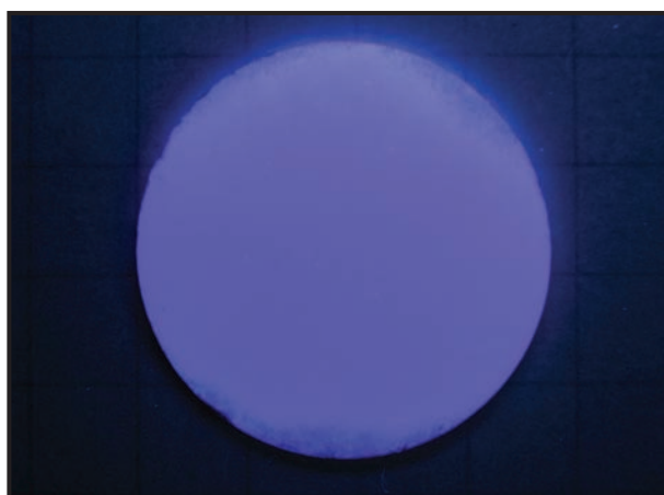
Figure 3. Photo of 25-mm × 1-mm-thick sintered sample illuminated by UV lamp
