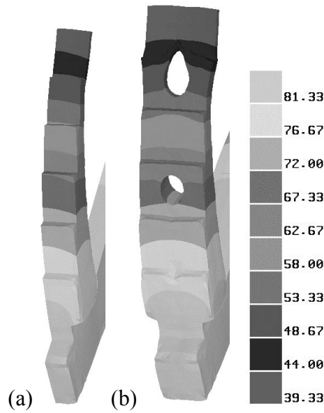
Figure 4.15: Temperature profile and part shape at 4,080 s. Thermal expansion from heating was used. (a) no-hole part, half of the part shown only, (b) two hole-casting.
