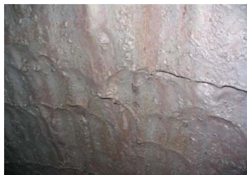
Fig. 3: Refractory surface wear dominated by chemical corrosive (dissolution).
