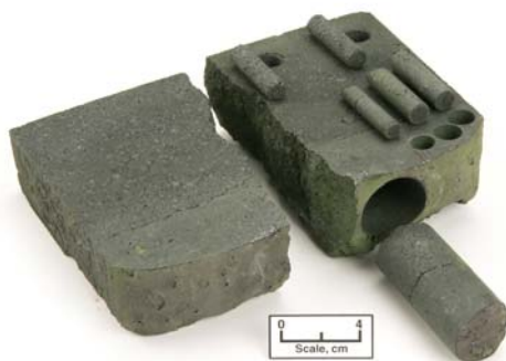
Fig. 7: Location of test samples removed from a Gasifier refractory sample
