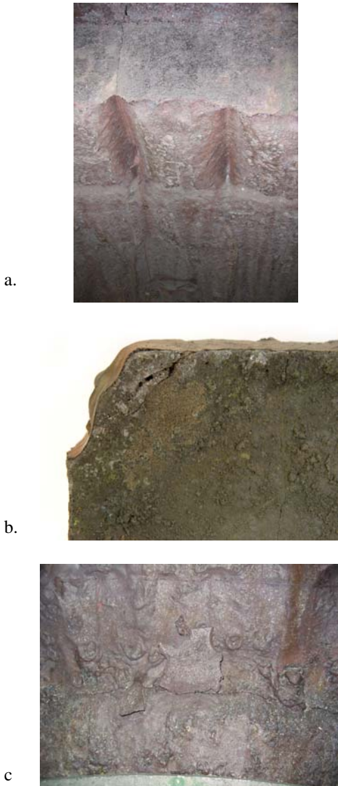
Fig. 4: Spalling examples in gasifier refractory; a) pinch spall along refractory joint, b) thermal spall, and c) structural spall.
