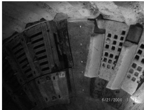
Figure 24: TPL™ Grates on Left. OEM Grates on Right
