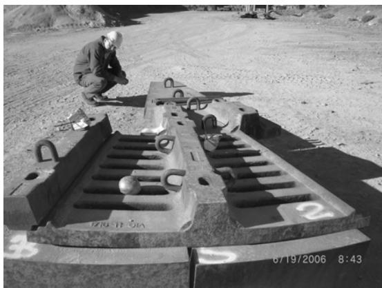
Figure 25: TPL™ Laid Out on Ground for Pre-Installation Review
