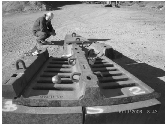
Figure 23: TPL™ Laid Out on Ground for Pre-Installation Review
