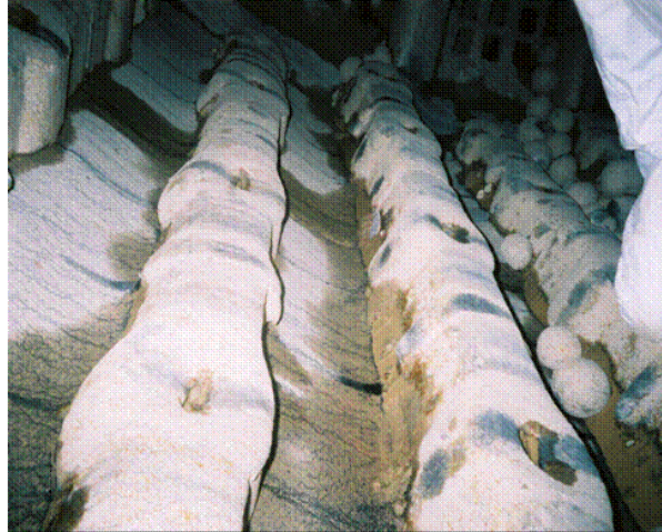
Figure 4: Lifter Peening From Ball Charge Overthrow
