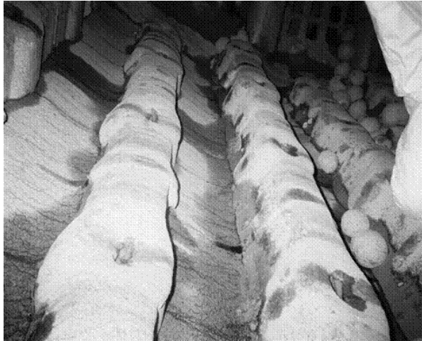
Figure 4: Lifter Peening From Ball Charge Overthrow
