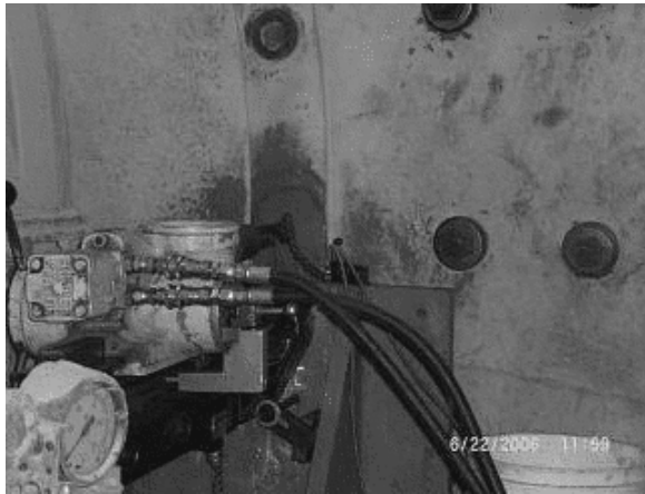
Figure 27: Drilling SAG Discharge Head to Complete Bolt Circle Pattern
