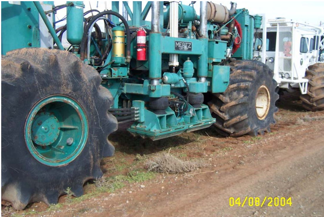
Figure 3-10. One of the trucks used to generate the seismic source energy.
