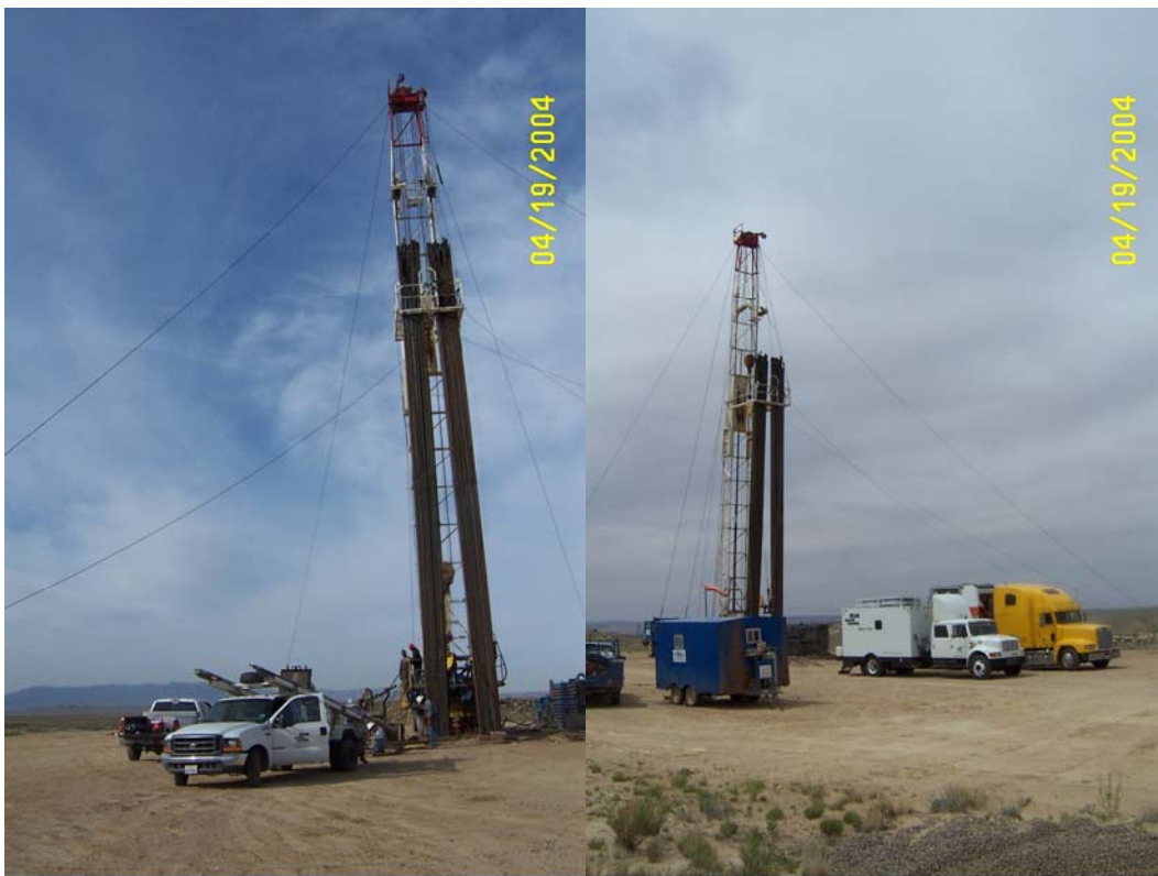
Figure 3-19. Rig for acquisition of the VSP data.
