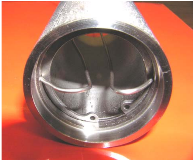
Figure 56. Arrangement used to hold two thermocouples in place with a snap ring.
