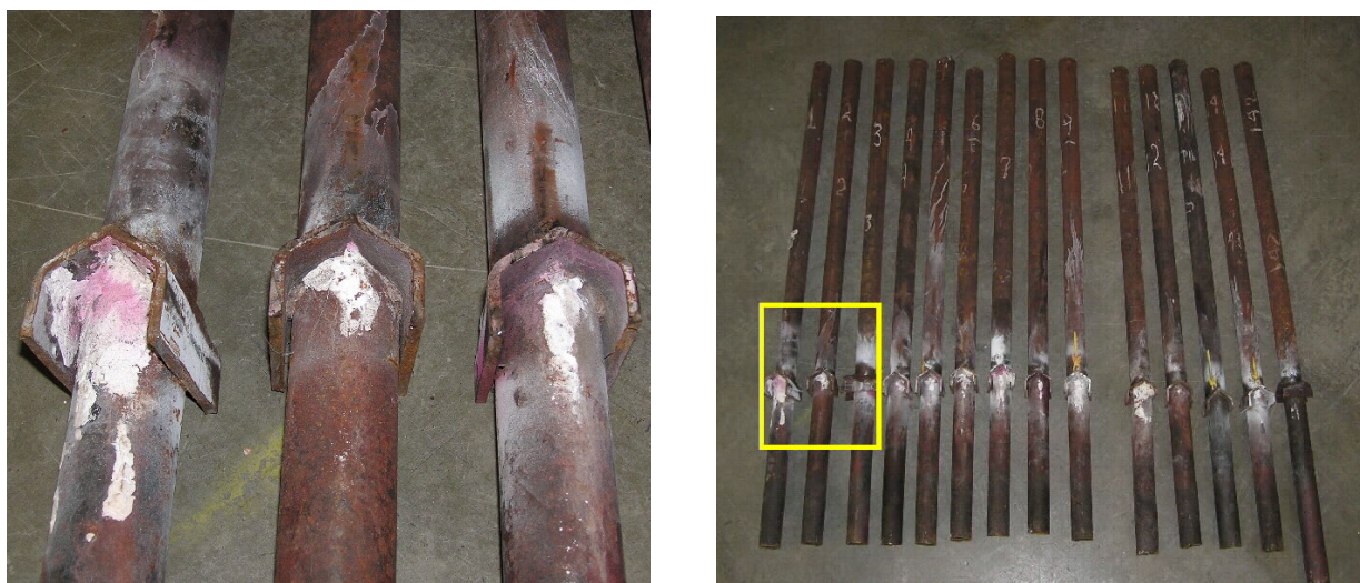
Figure 30. Fourteen unfailed superheater tubes removed from the intermediate superheater for inspection to determine if any cracking has occurred.
