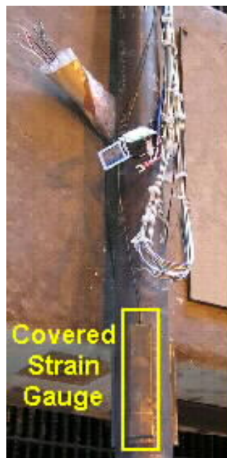
Figure 36. Section of superheater tube with thermocouple and strain gauges mounted and a special protective cover installed.
