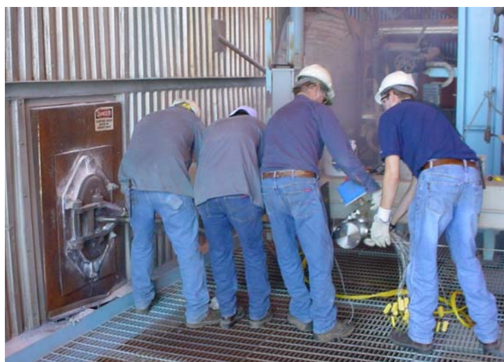
Figure 58. Corrosion probe being inserted through hole in manway door.
