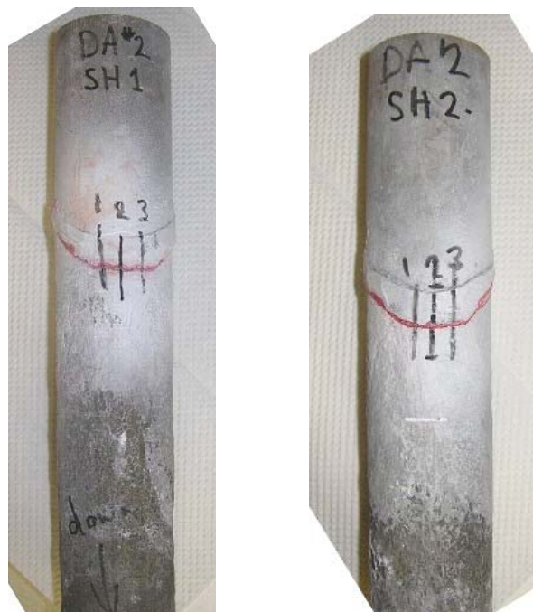
Figure 25. Cracked superheater tubes after dye penetrant examination. Both tubes showed a crack that followed the weld line along the bottom of the tube to high crown seal weld. The vertical lines and the numbers indicate locations from which metallographic samples were cut.
