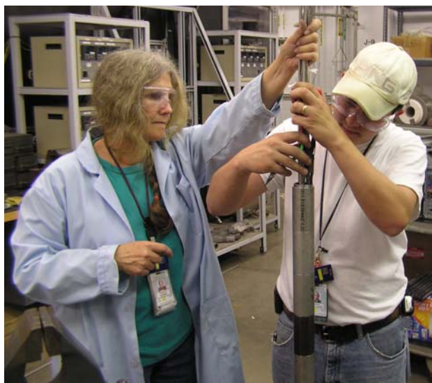
Figure 54. Corrosion probe being assembled. Thermocouples and support rods extend through the four samples already mounted.
