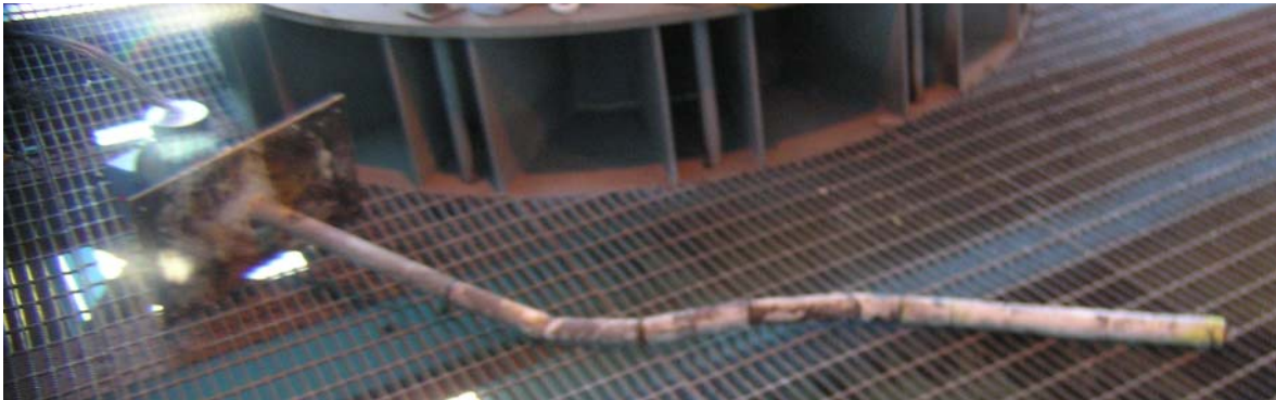
Figure 60. Corrosion probe after removal from recovery boiler. considered to have been exposed at temperatures above the FMT for the majority of the
