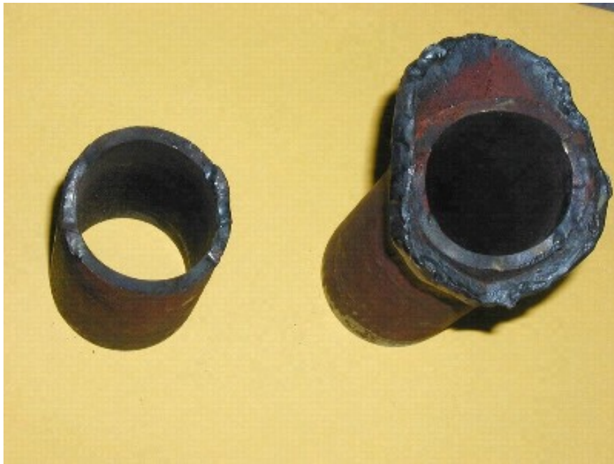
Figure 18. Photo showing the fracture surfaces of the superheater tube shown in the previous figure. Note the smooth surface at the 3 and 9 o'clock positions resulting from damage during removal of the tube.
