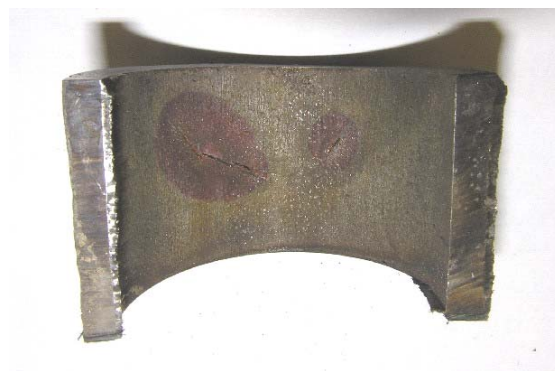
Figure 26. Photos of the inside surfaces of the two tubes shown in the previous figure. Both tubes have cracks that have penetrated through the wall. The crack pattern appears to mimic the directionality of the tube to high crown seal weld.
