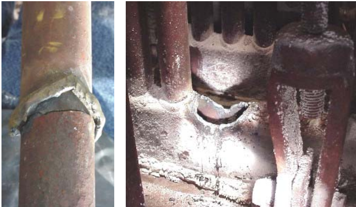
Figure 17. The photo on the left shows the two sections of the failed superheater tube that were examined, and the photo on the right shows the position in the high crown seal from which the tube was removed.
