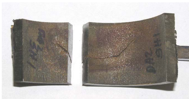
Figure 26. Photos of the inside surfaces of the two tubes shown in the previous figure. Both tubes have cracks that have penetrated through the wall. The crack pattern appears to mimic the directionality of the tube to high crown seal weld.
