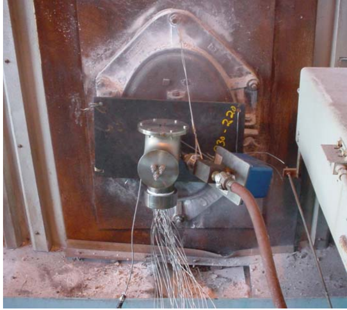
Figure 59. Corrosion probe installed in recovery boiler superheater. The air supply line and regulating valve are on the right and the 30 thermocouples extend from the bottom of the probe.
