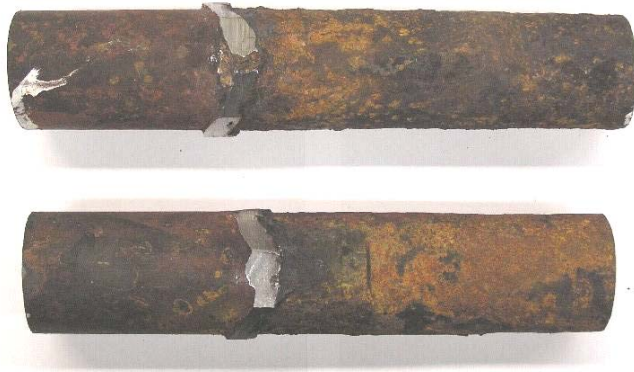
Figure 24. Sections of two failed intermediate superheater tubes removed during Fall, 2004.
