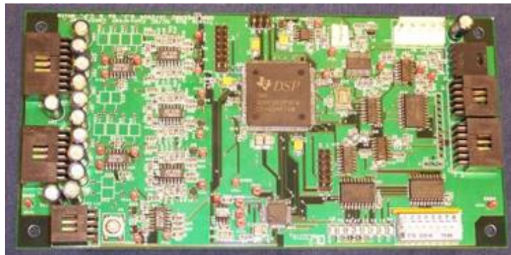
Figure 9. Photo of the DSP control board. Size: 7.0 \times 3.5 in.
