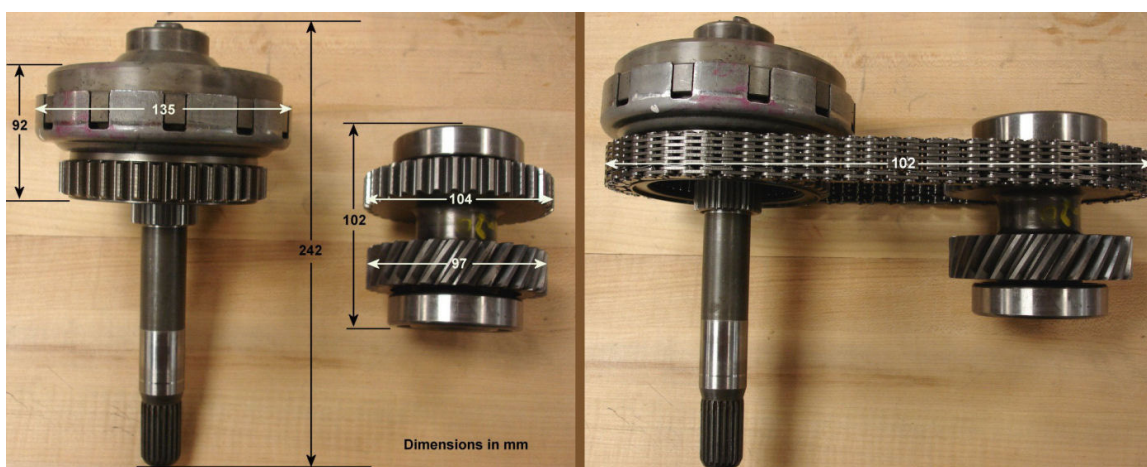
Figure 13. Dimensions for planetary gear, the first reducer gear, and extension.
