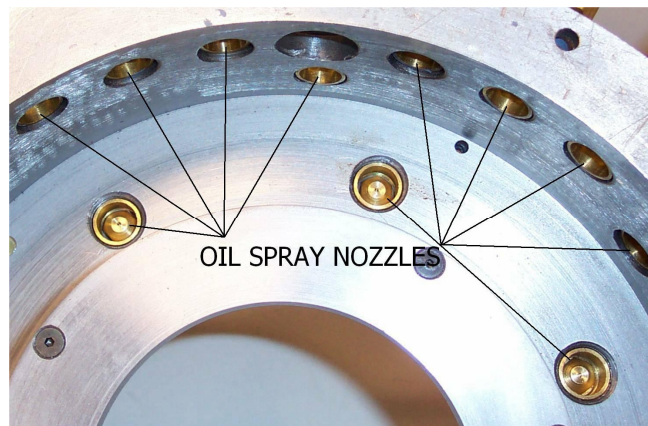
Figure 1. Photo of inside of motor housing showing spray nozzle locations.
