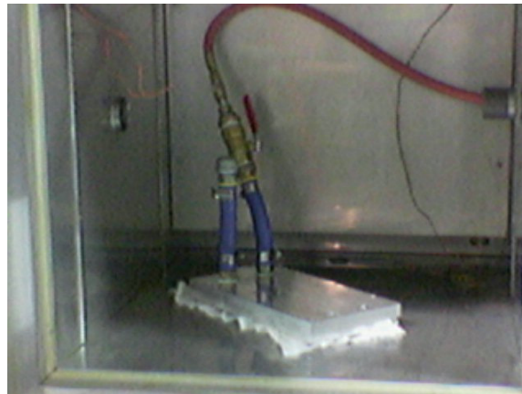
Figure 11. Baseplate leak test setup.
