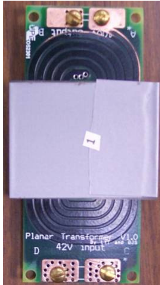
Figure 8. Photo of the planar transformer. Footprint: 4.875 \times 2.125 in.
