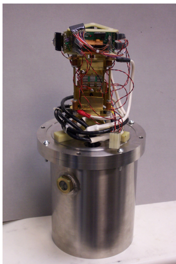
Figure 6. Core of first FY 2006 ORNL prototype inverter.
