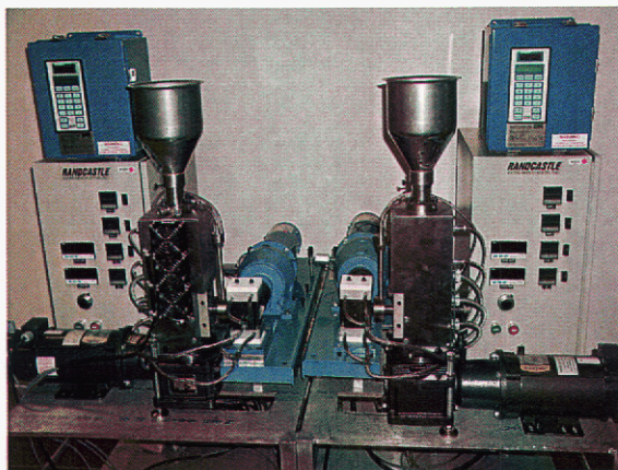
Figure 9: Sandia's multilayer coextrusion system.
