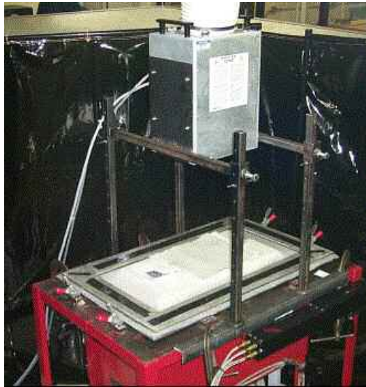
Figure 24. UV Lamp mounted over the RIDFT.
