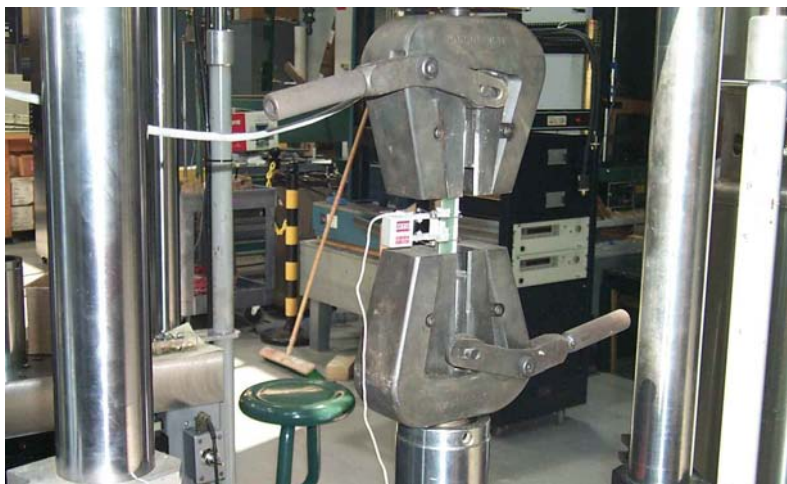
Figure 28. Setup for the tensile testing of composite laminates.
