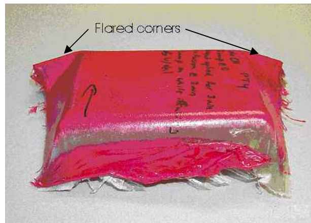
Figure 6. Part with flared corners.
