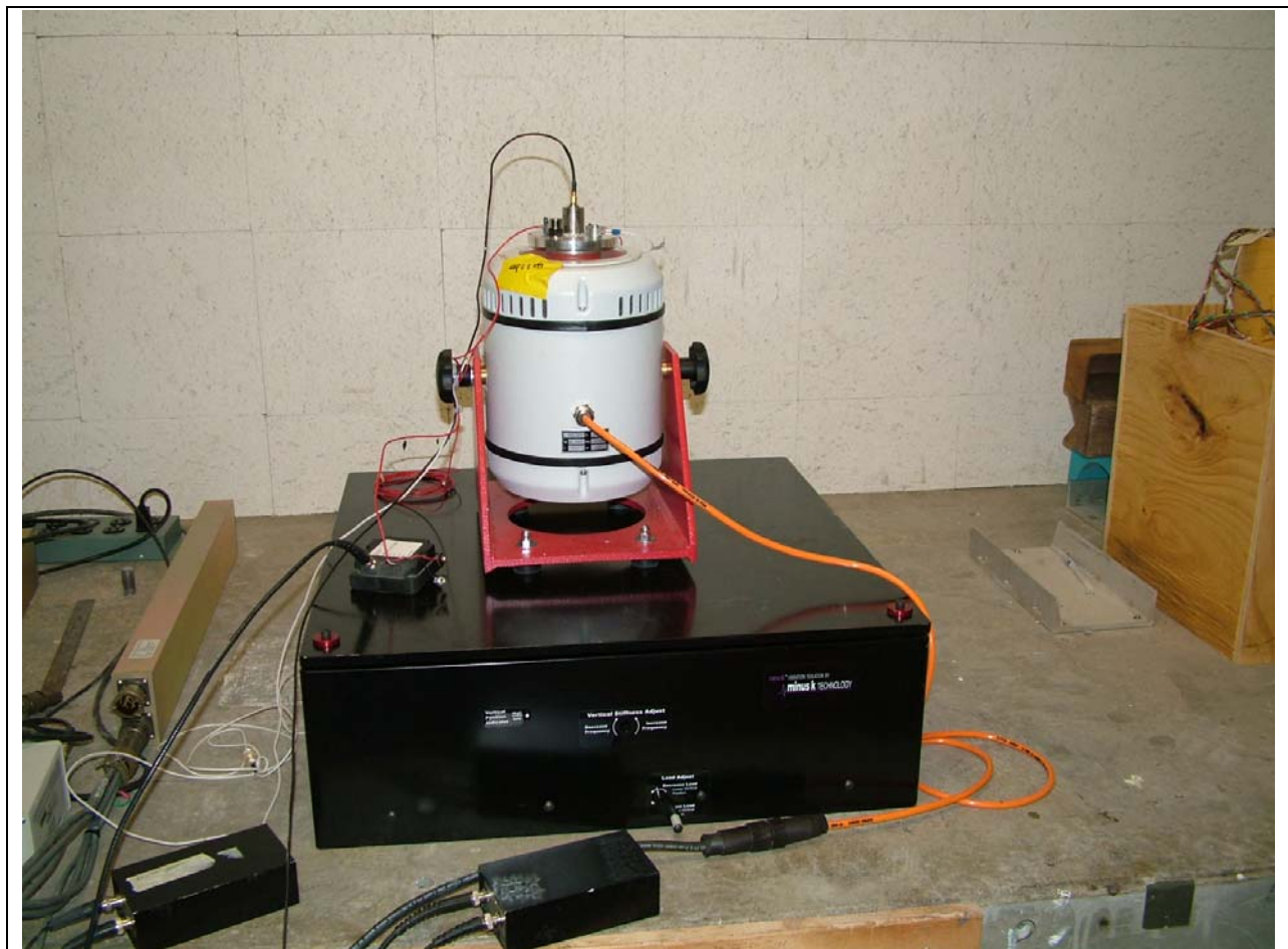
Figure 15. Photograph of shaker table in the underground vault
