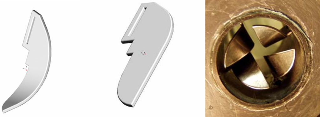
Figure V.1. (a) A sketch of the SMA fin shown in its unheated, relatively soft martensite phase at a temperature below T_c . (b) The same SMA fin shown in its heated, relatively stiff austenite phase at temperatures above T_c . (c) Photo of an assembly of four such SMA fins in the new Vortigen concept.
