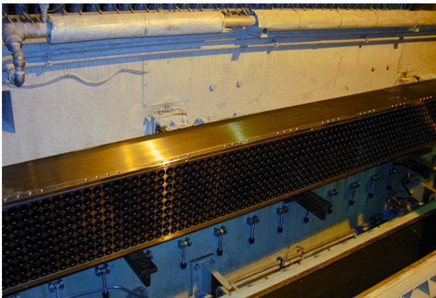
Figure III.3. Vortigen tube block being inserted inside a Voith Headbox.
