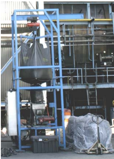
Figure 2-2. Norit Port-a-Pac Carbon Feeding System
