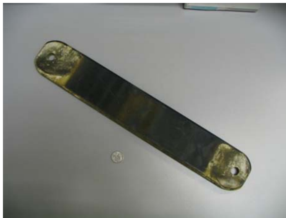
Figure 3-8. Damaged Insulator from Yates Unit 1 ESP
