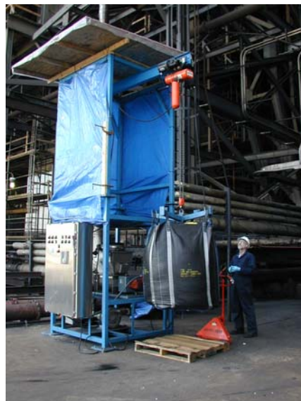
Figure 2-4. Port-a-Pac Dosing Unit Similar to the One Used in Parametric Testing
