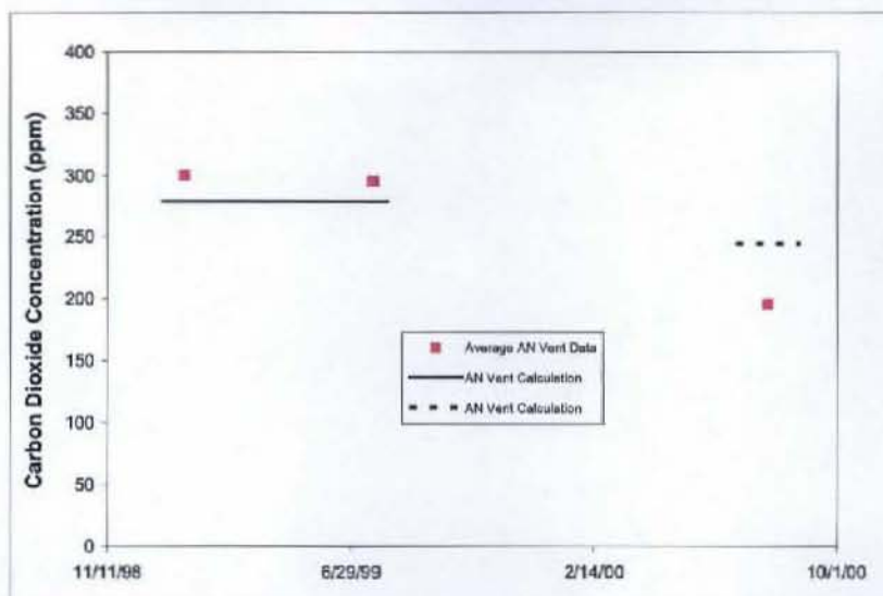
Figure 4-81 241-AN Farm Predicted and Measured Ventilation CO 2 Concentration.
